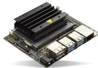
Figure 2. Illustration of sink used in the NVIDIA® Jetson Nano™ Processor.
