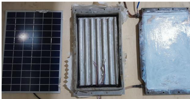
Figure 3. PVT+PCM system components.
