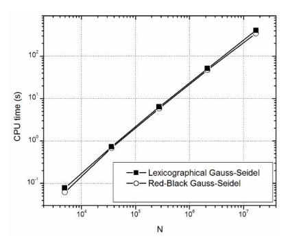
Fig.4. Comparison of the lexicographical Gauss-Seidel (injection restriction) and red-black Gauss-Seidel (full weighting restriction).
