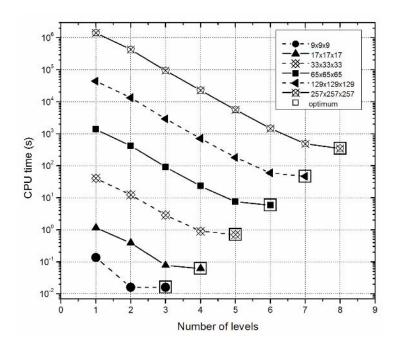
Fig.3. Number of levels versus the CPU time for the grids (from N = 5x5x5 to N = 257x257x257) for the Poisson equation and red-black Gauss-Seidel solver.
