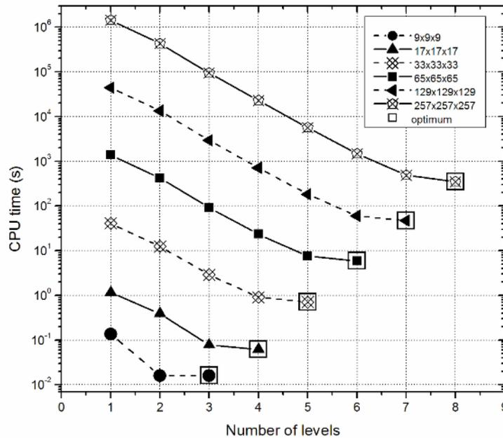
**Figure 2: Number of levels versus CPU time for the grids ( $N = 5 \times 5 \times 5$  a  $N = 257 \times 257 \times 257$ ) for the Poisson equation and red-black Gauss-Seidel solver**
