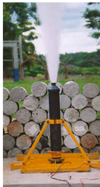
Fig. 2. The rocket motor was mounted vertically, with the nozzle facing upward, in a metallic holder
