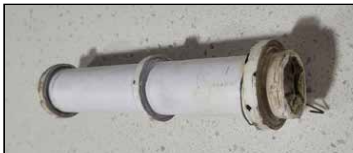
Figure 6. A poorly designed motor mount adapter made from paper. Notice how crushed it is at the base. It couldn't handle the H87 motor I used.
