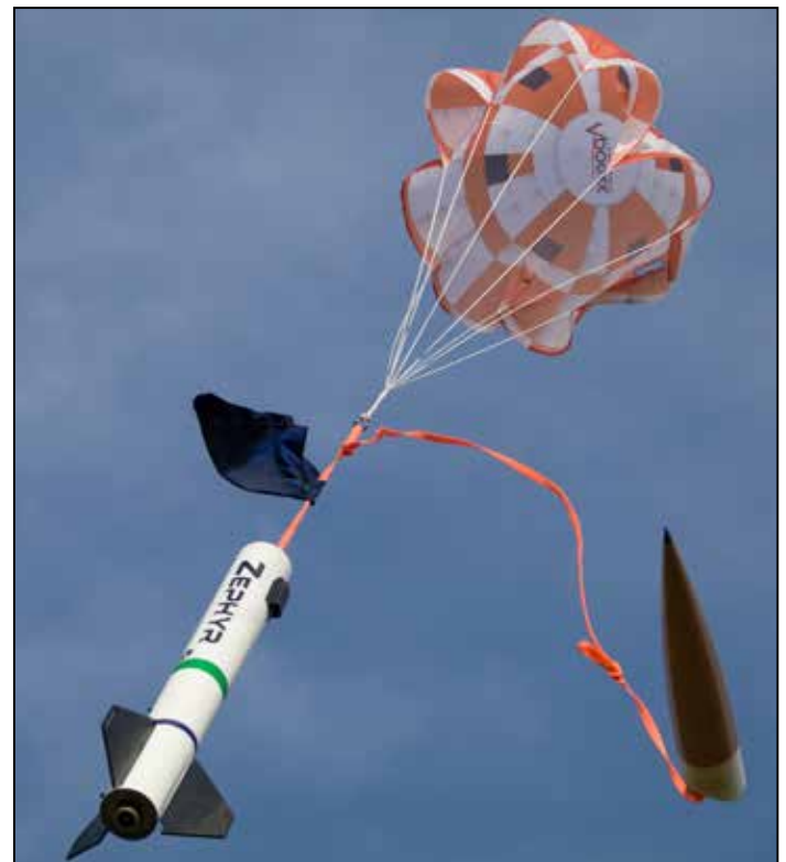
Figure 9 - Look at all the tension in that shock cord. If you have an AV bay, it will need to support that load.
