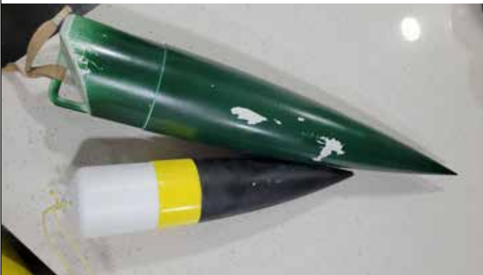
Figure 2. A comparison of the nose cone that comes with the Zephyr (in green) and the nose cone I used for my Electron (yellow and black). Look at how much more beefy the Zephyr nose cone is! After the loop for the shock cord was ripped off the Electron's nose cone, I drilled holes in the base of it to attach the shock cord.
