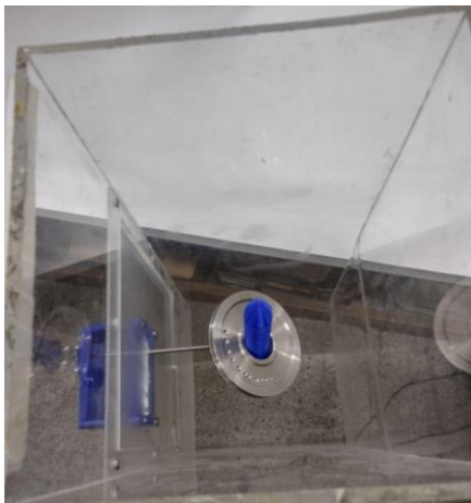
Fig. 5: Load cell during calibration procedures.
