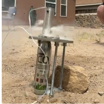
Fig. 74 Vertical ejection system testing: 50g of CO 2 with SRAD altimeters on ground test mode.
