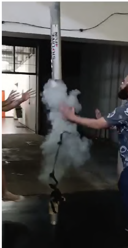
Fig. 79 Vertical ejection system testing: 50g of CO 2 with SRAD altimeters on ground test mode.
