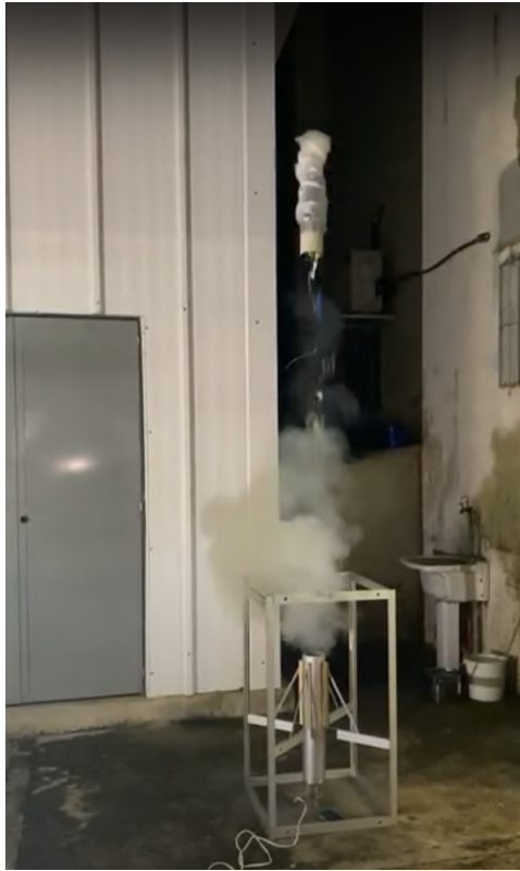
Fig. 71 Vertical ejection system testing: 50g of CO 2 in a 4.2" diameter module.
