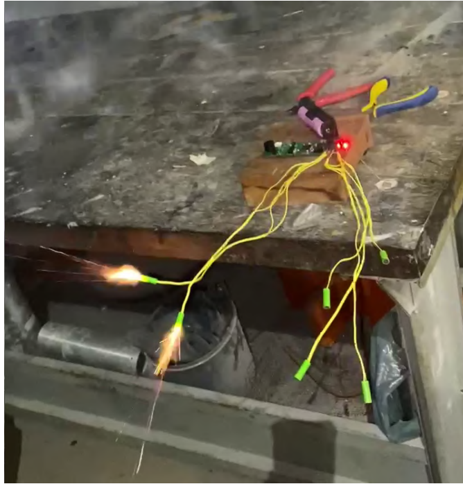
Fig. 83 SRAD altimeter ground test. Moment of e-match activation
