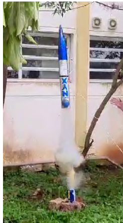
Fig. 78 Vertical ejection system testing: 50g of CO 2 with SRAD altimeters on ground test mode.
