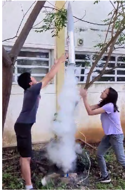
Fig. 80 Vertical ejection system testing: 50g of CO 2 with SRAD altimeters on ground test mode.
