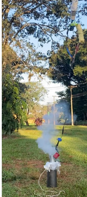
Fig. 72 Vertical ejection system testing: 50g of CO 2 in a 4.2" diameter module.
