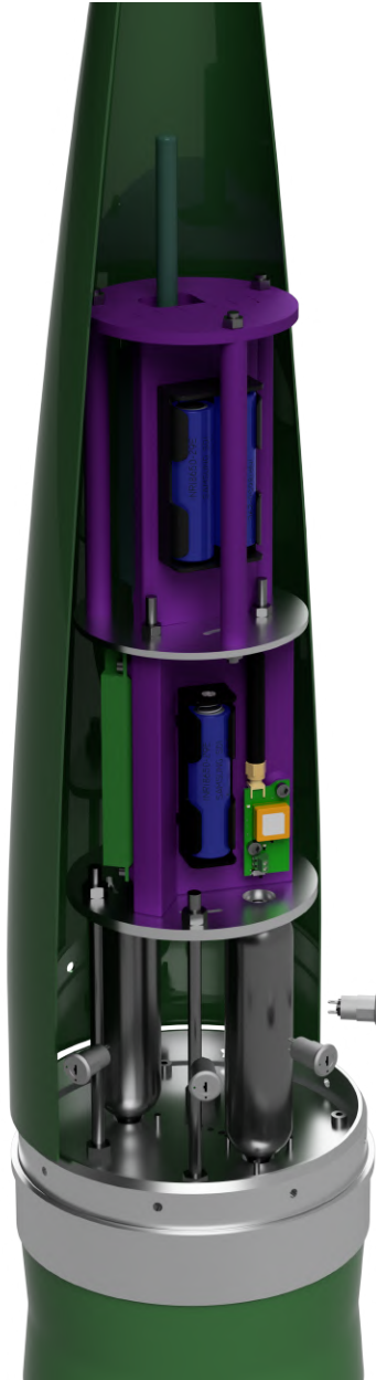
Fig. 55 Schematic view of the Electronic Systems in the nosecone.
