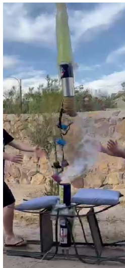
Fig. 75 Vertical ejection system testing: 50g of CO 2 with SRAD altimeters on ground test mode.
