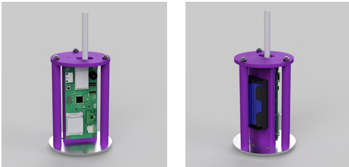
Fig. 65 Telemetry module with SRAD telemetry board and two Li-Ion batteries.
