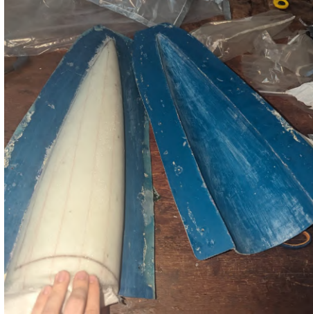
Fig. 92 Fiberglass nosecone demolding after initial curing. Vacuum consumables are still inside the piece.
