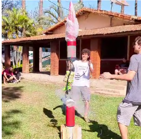
Fig. 76 Vertical ejection system testing: 50g of CO 2 with SRAD altimeters on ground test mode.
