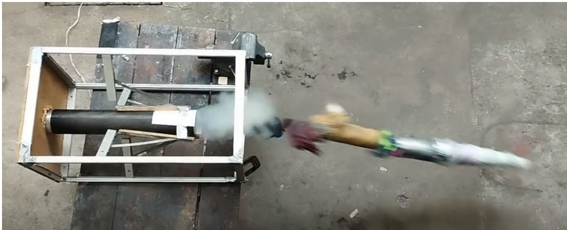
Fig. 70 Horizontal ejection system testing: 90g of CO 2 in a 5" diameter module.
