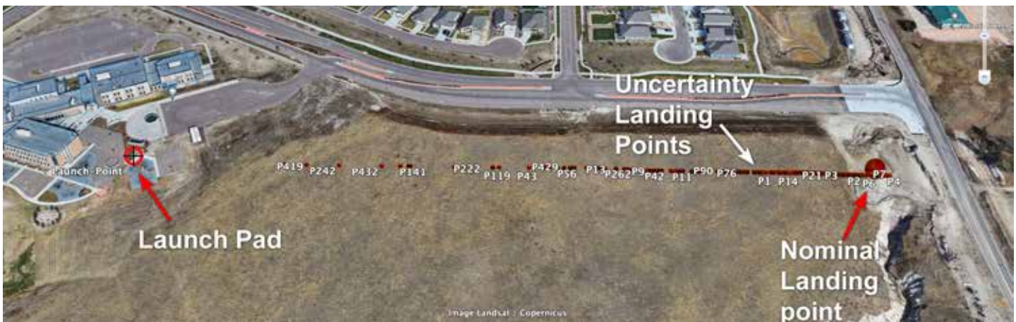
Figure 8 - The same landing point plot, but this time overlaid on a Google aerial photo.
