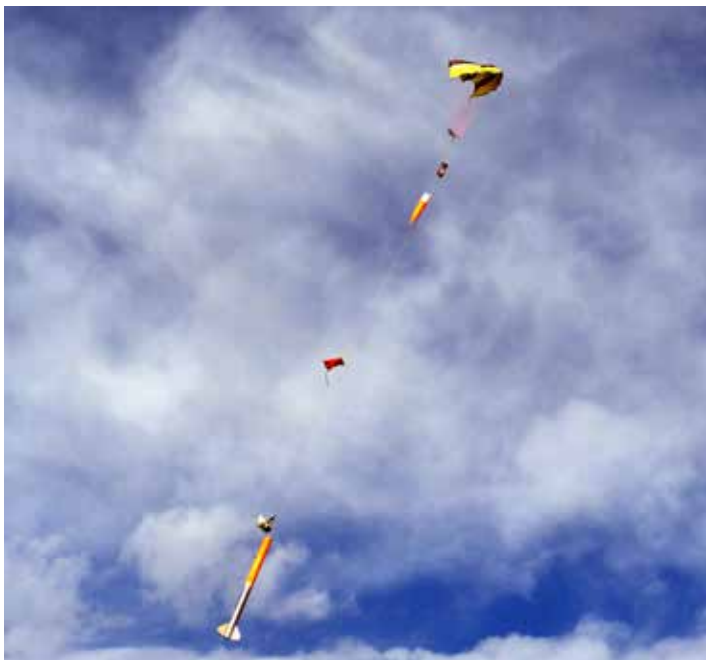
Figure 5 - Apogee's gliding parachute system allows you to control the flight of the rocket, so you can land it exactly where you wish.
