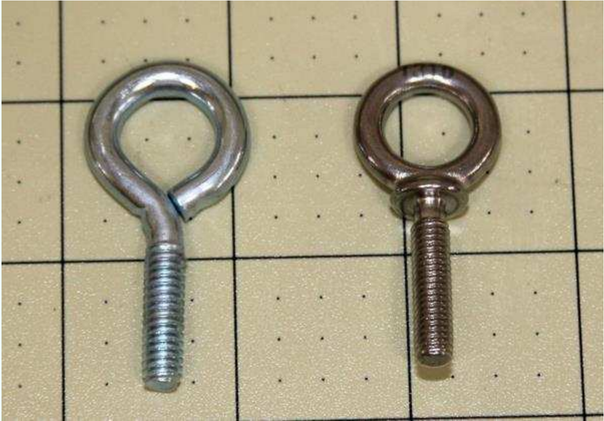
Figure 6-31. An open eye bolt on the left, and a forged eye bolt on the right.
