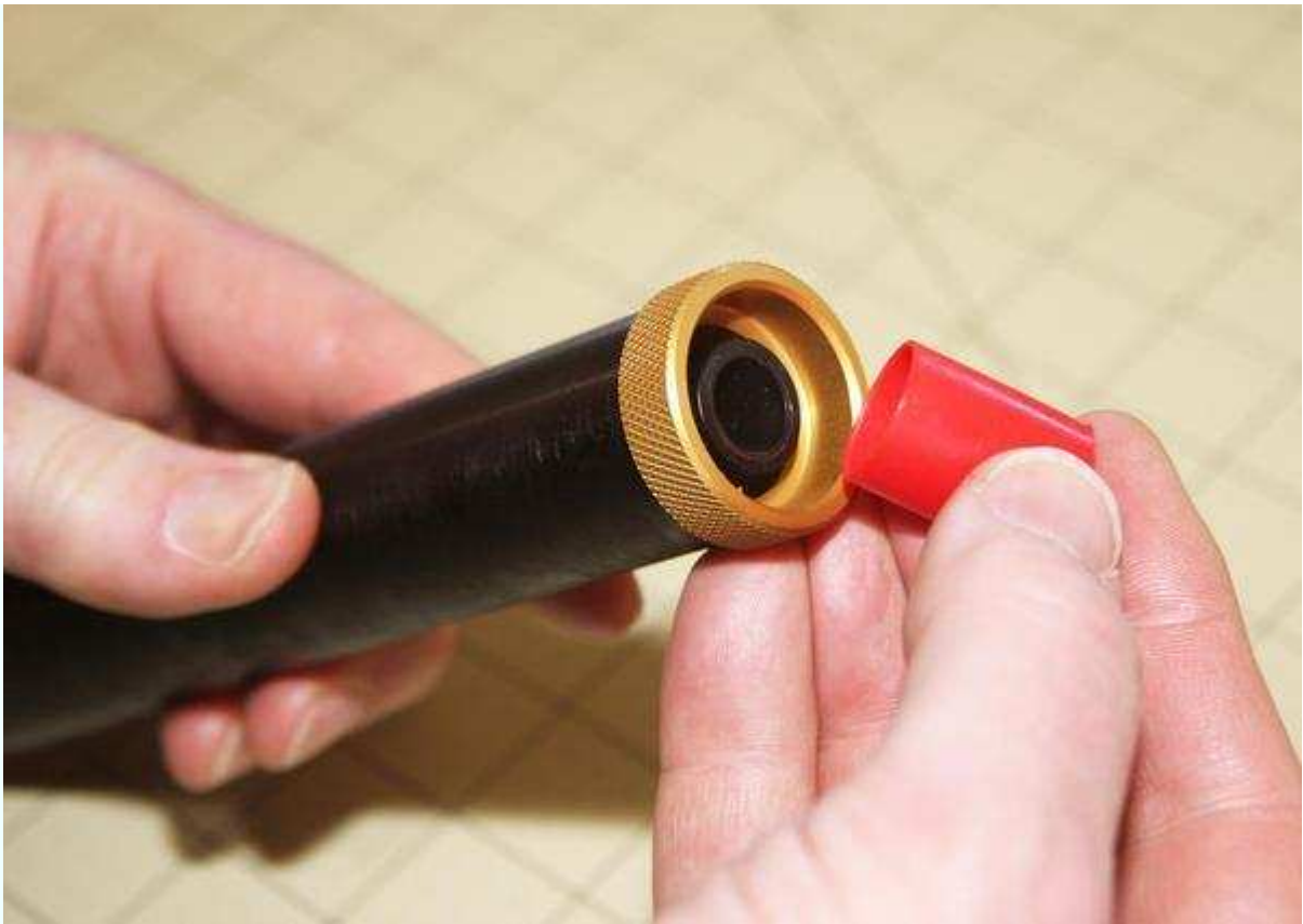
Figure 4-26. Cover the nozzle with the smaller plastic cup.
