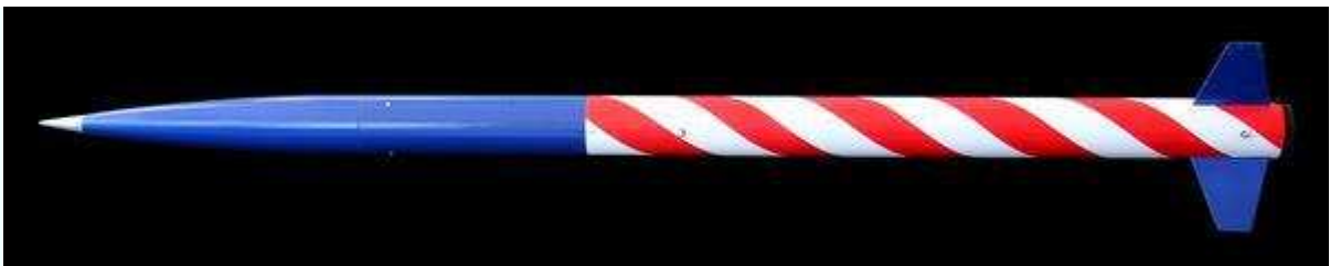
Figure 6-24. Phobos is a sturdy fiberglass Level 2 rocket, built for supersonic flight.
