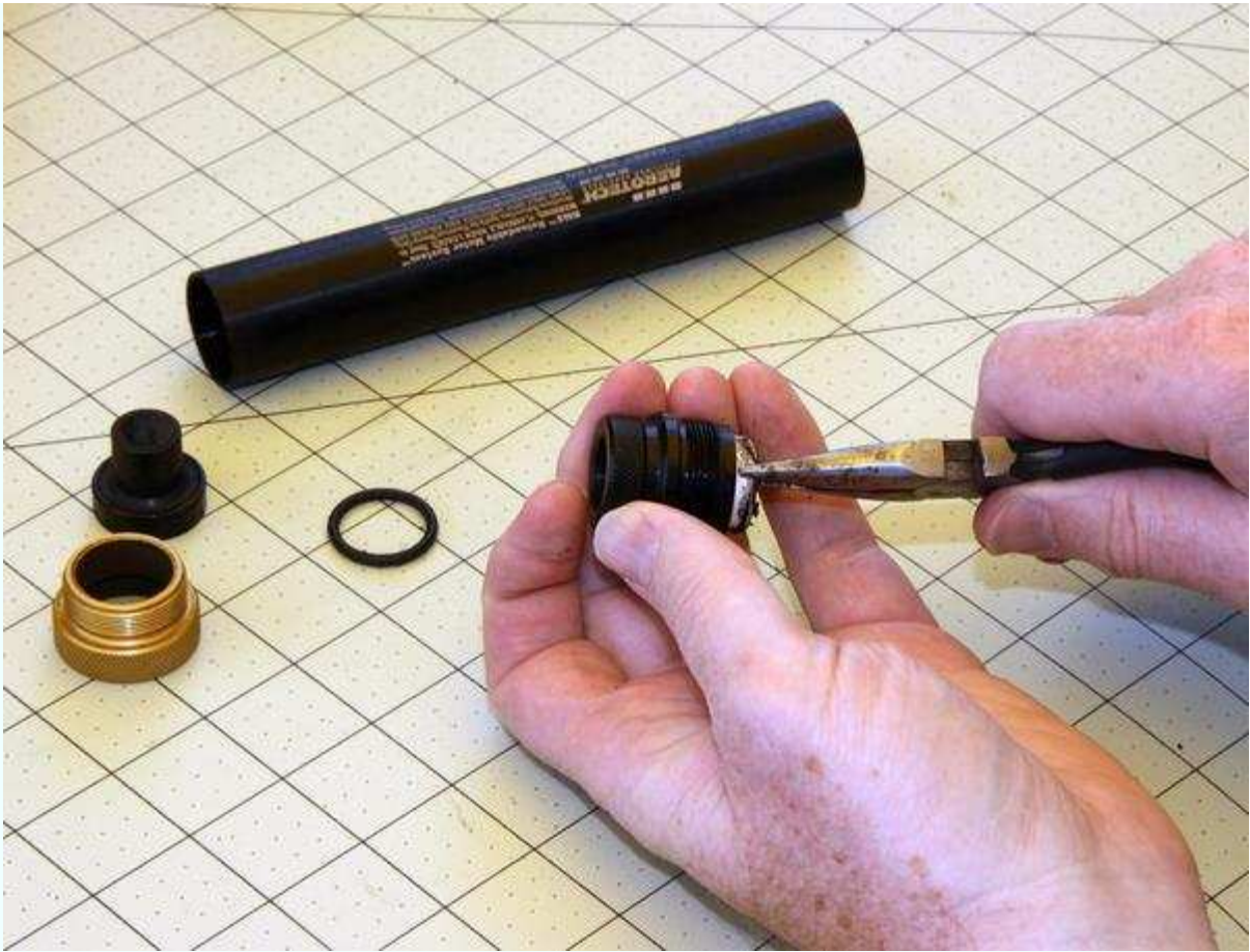
Figure 5-14. Push out the motor liner.
