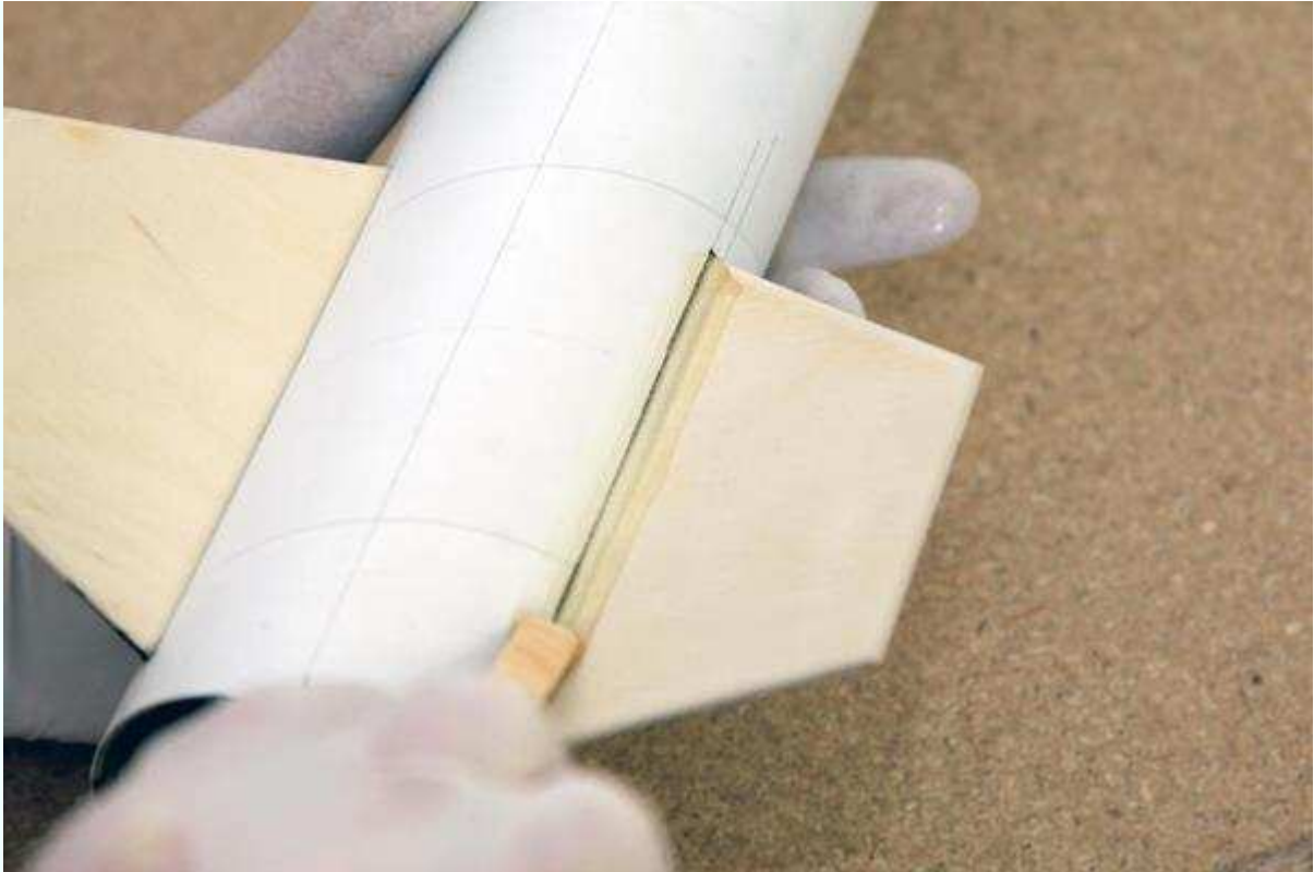
Figure 3-46. Use a popsicle stick or other curved surface to apply a smooth fillet to the two outside locations.
