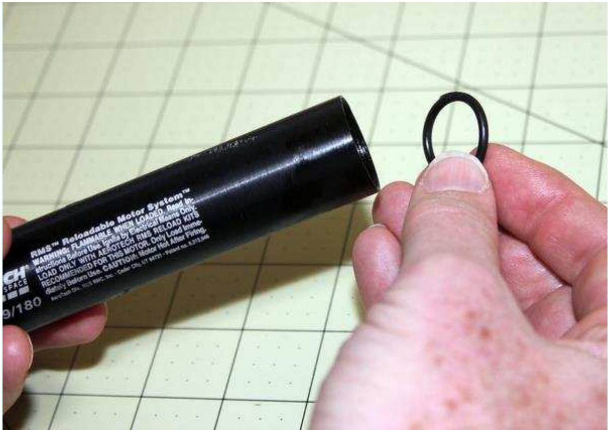
Figure 4-20. Insert the thicker O-ring; this is the forward O-ring.
