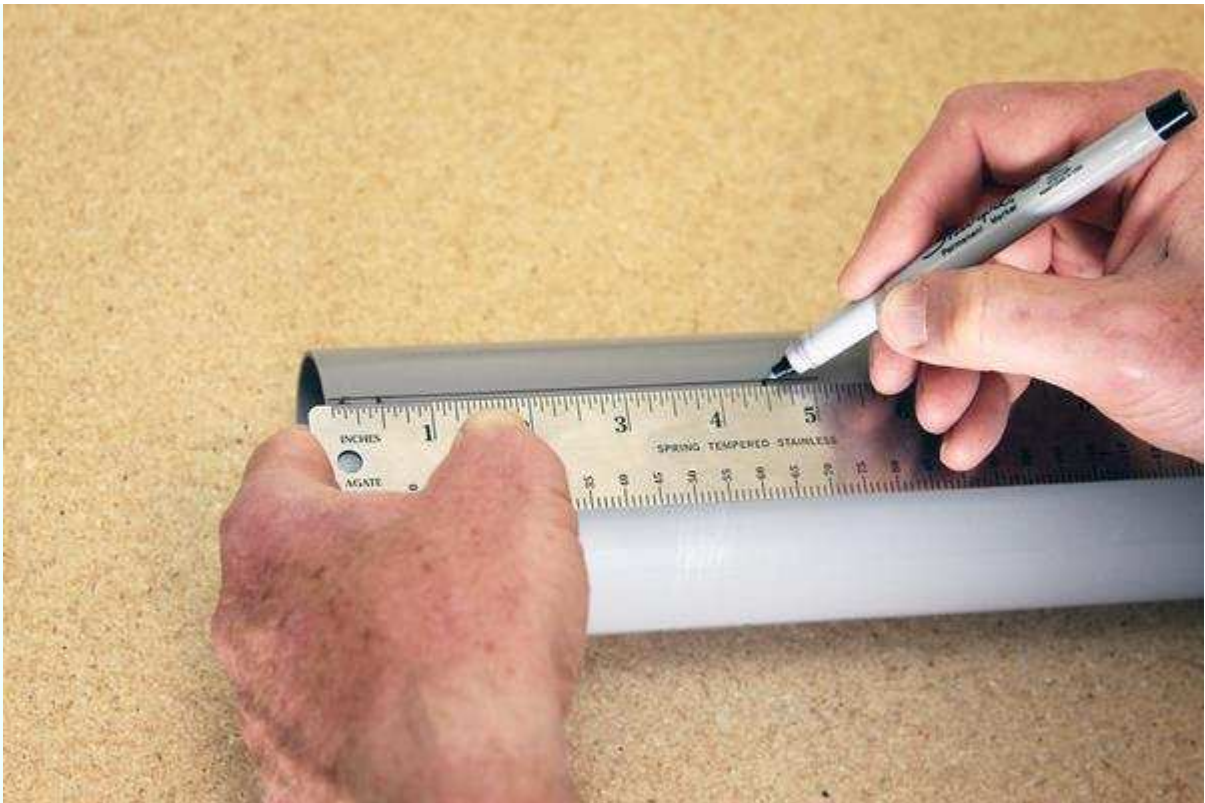
Figure 6-6. Use a fine-tip marker to mark the sides of the fin slots and the locations of the rail buttons.
