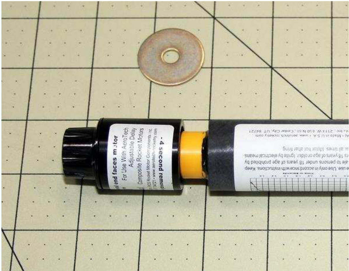
Figure 4-39. Remove the brass washer. Insert the drill bit so the -4 second label is on the side the drill sticks out of. Drill out the excess delay material.
