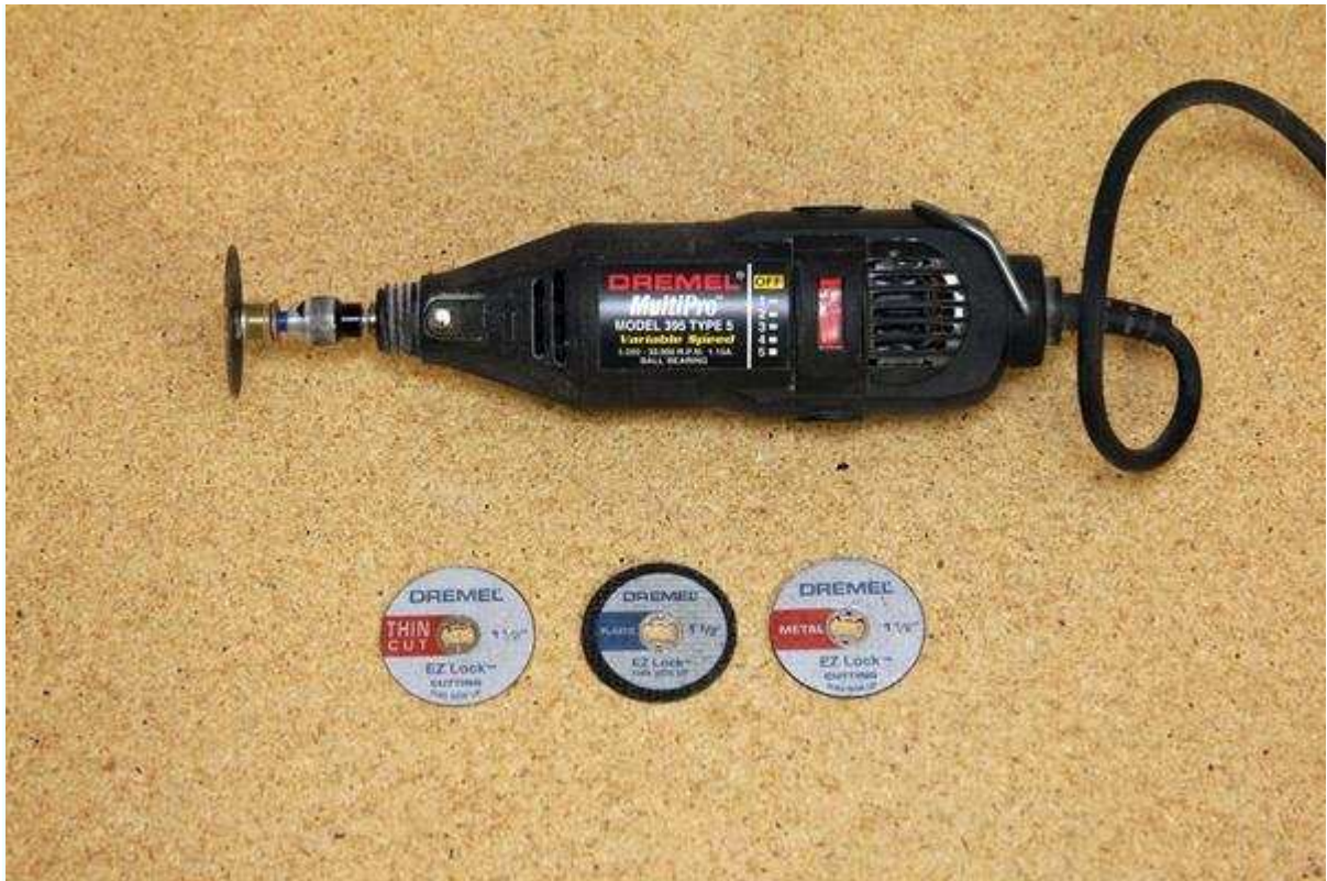
Figure 3-18. Dremel tools can cut pretty much anything the hobby knife cannot.
