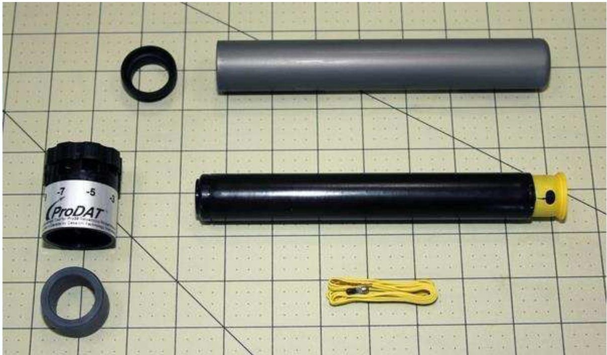
Figure 4-27. You need a motor case, aft retainer, reload, and Delay Adjustment Tool to prepare and fly the H163-14A.
