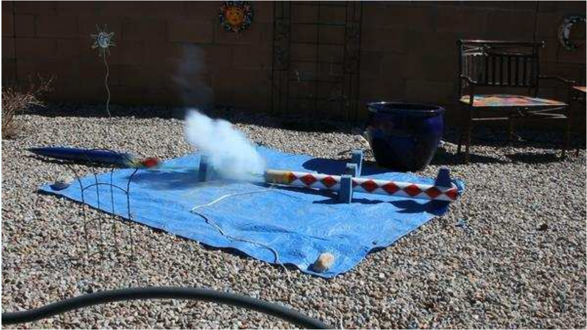
Figure 8-19. Upper bay ejection charge test for Deimos. The parts are still very much in motion in this frame, taken from a movie of the test.
