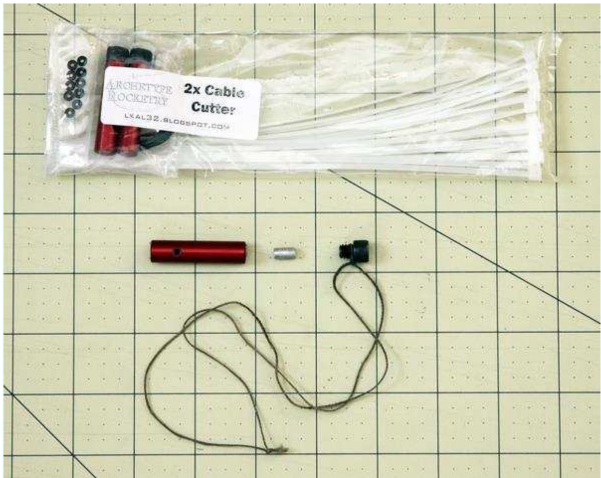
Figure 7-8. A pyrotechnic cable cutter holds a small black powder charge. This drives a piston that cuts a cable.
