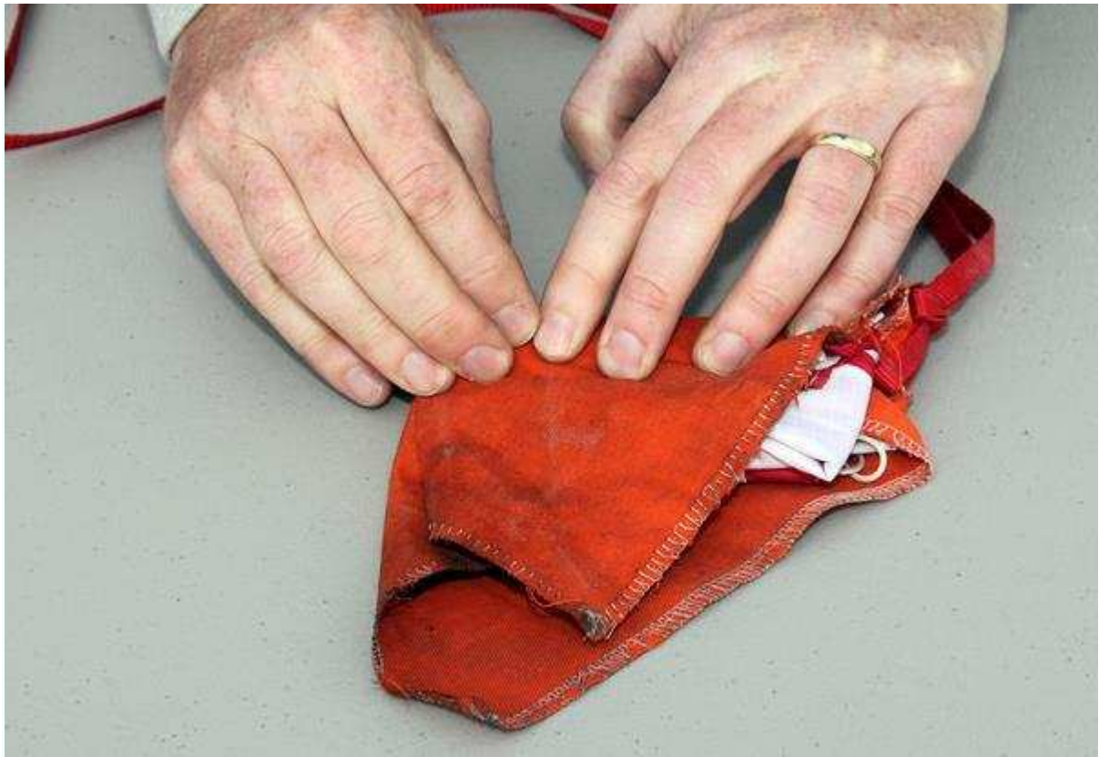
Figure 5-6. Fold one corner across the parachute bundle.
