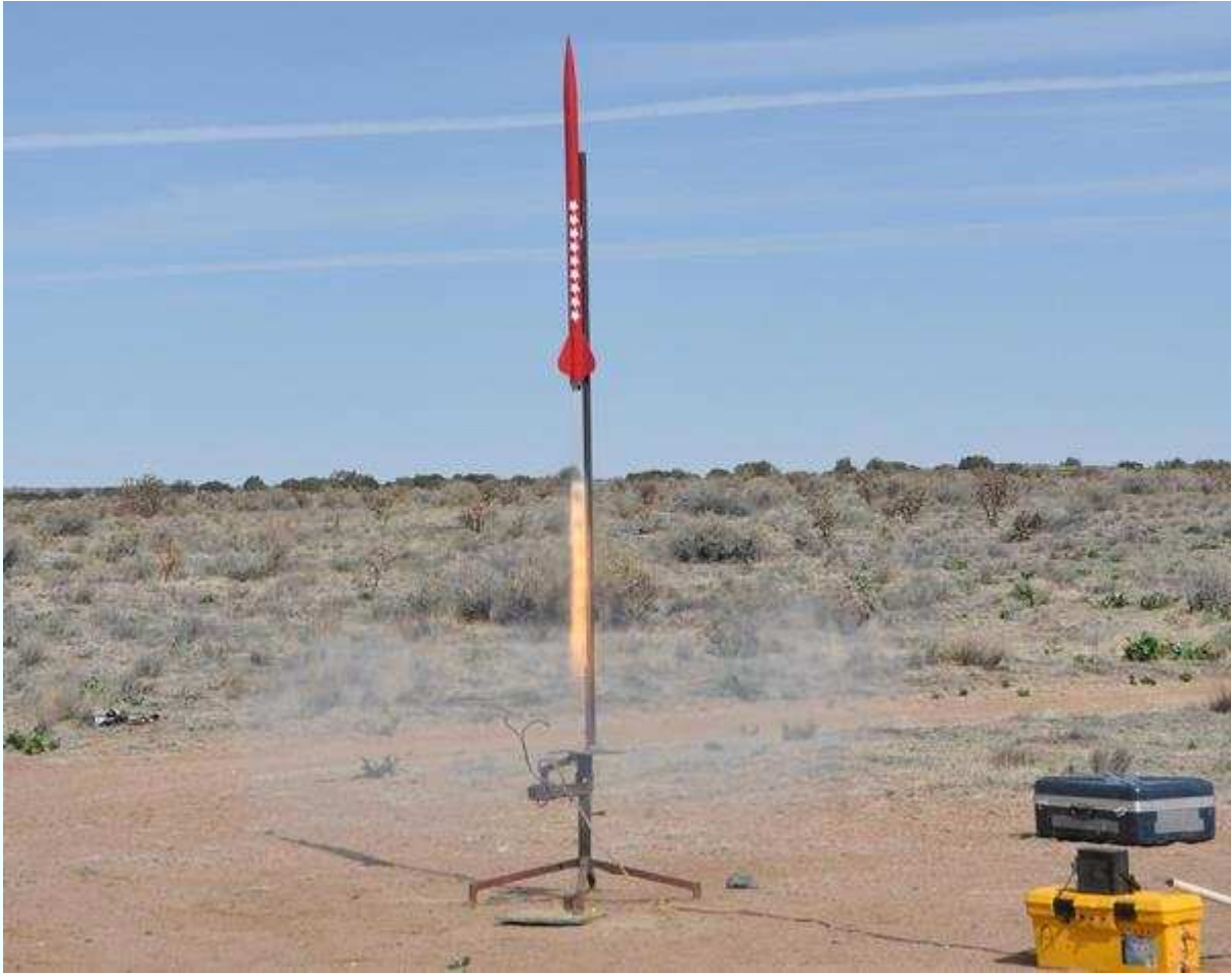
Figure 1-1. Todd Kerns's Space Cowboy lifts off. The exhaust plume clearly shows Mach diamonds, a standing wave that can appear in supersonic exhaust plumes. Photo by Jim Jewell.
