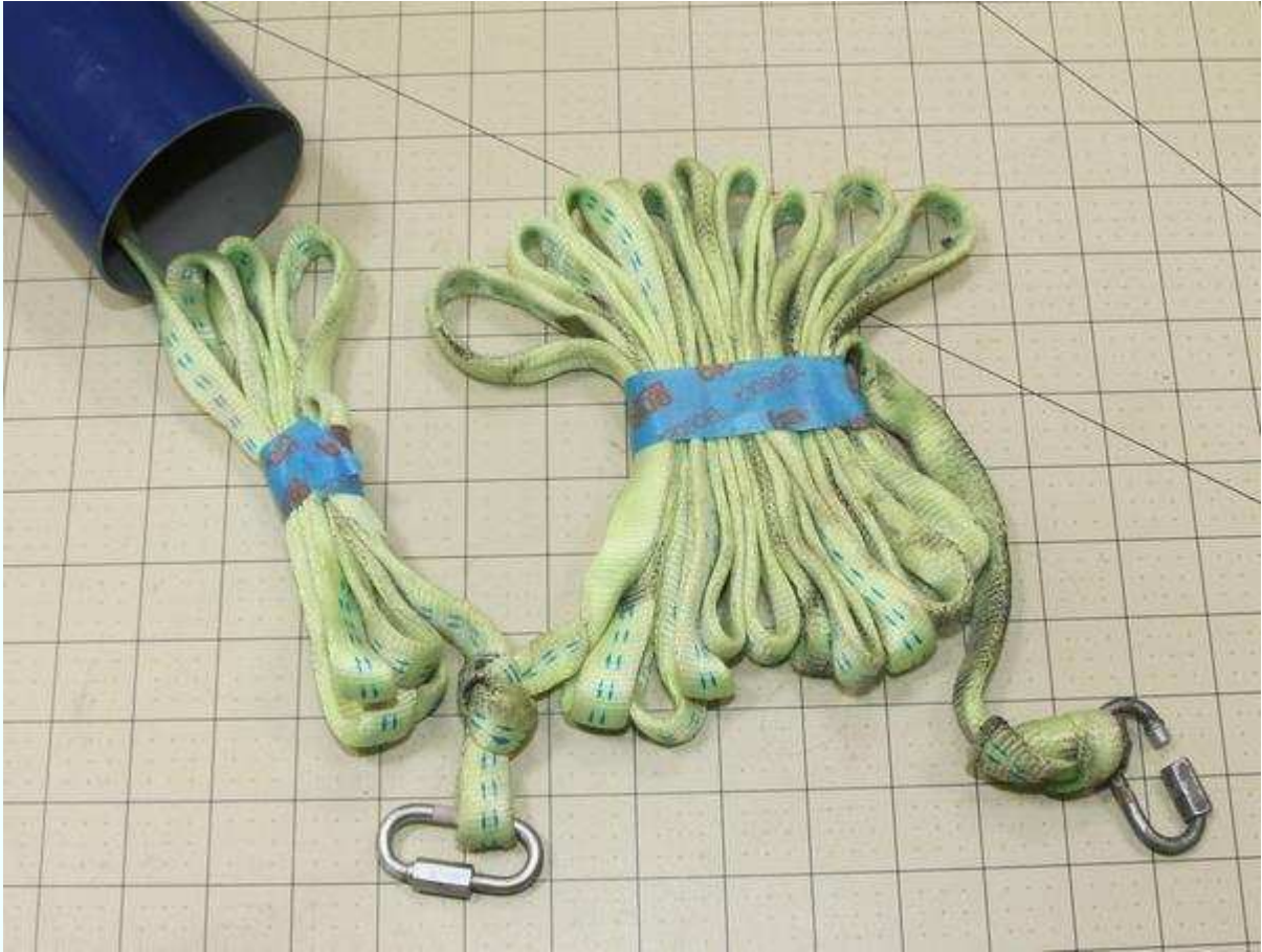
Figure 9-1. Z-folding is a common and effective way to pack a shock cord.
