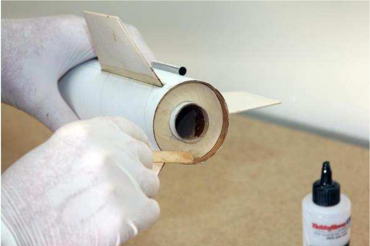
Figure 3-54. Apply a glue fillet where the centering ring touches the airframe, but not where it touches the motor mount.
