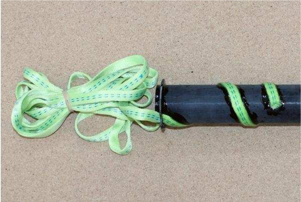
Figure 6-36. Cut a notch in the forward centering ring large enough for the shock cord, then glue the centering ring and shock cord in place.
