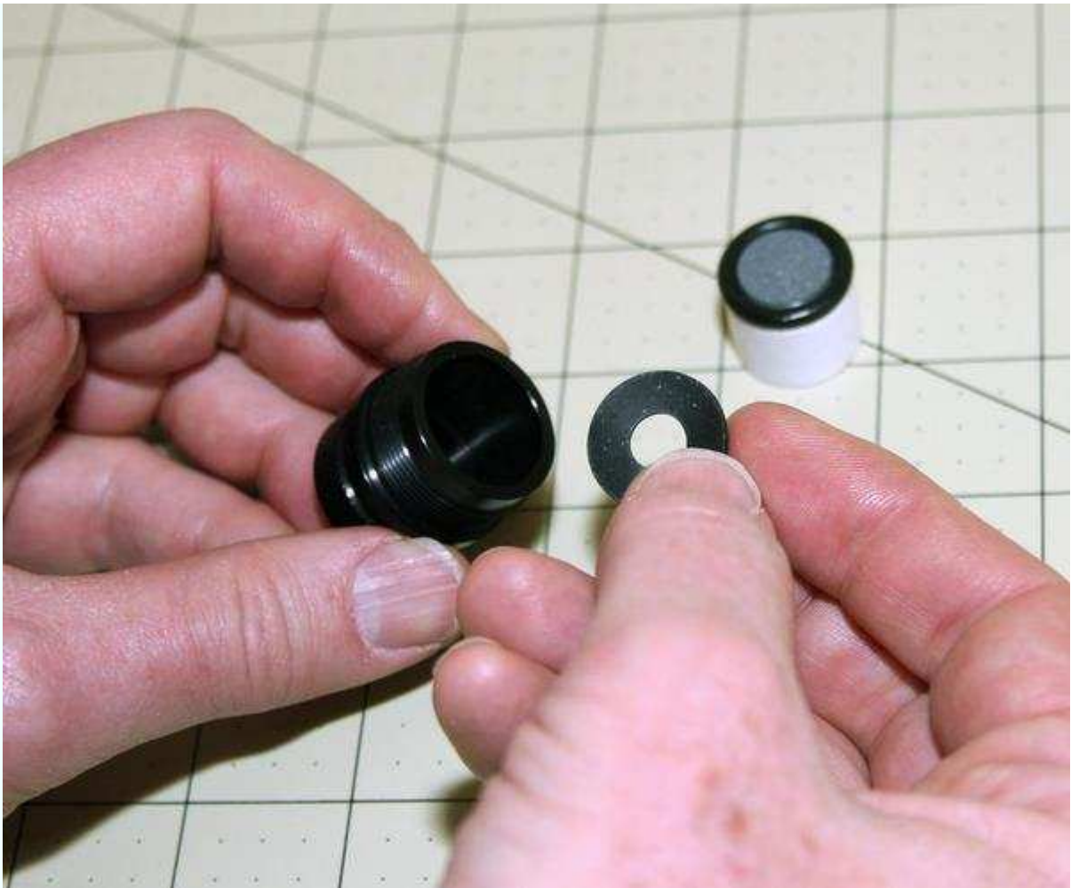
Figure 4-15. Insert the forward spacer, apply a light coat of grease to the walls of the forward closure, and slide the delay assembly into the forward closure, O-ring first.
