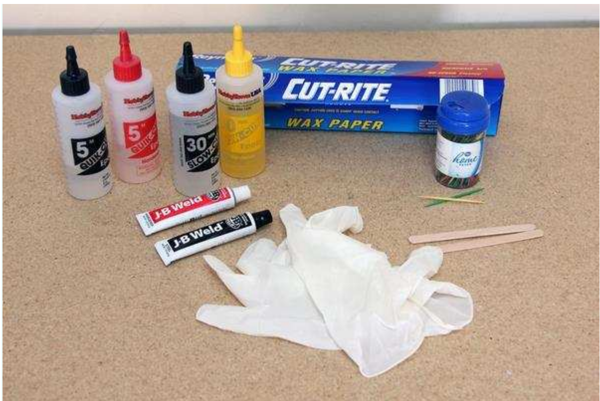
Figure 3-21. Most high-power rockets are built with epoxy glue, but paper and wood rockets like Callisto can also be built using wood glue.
