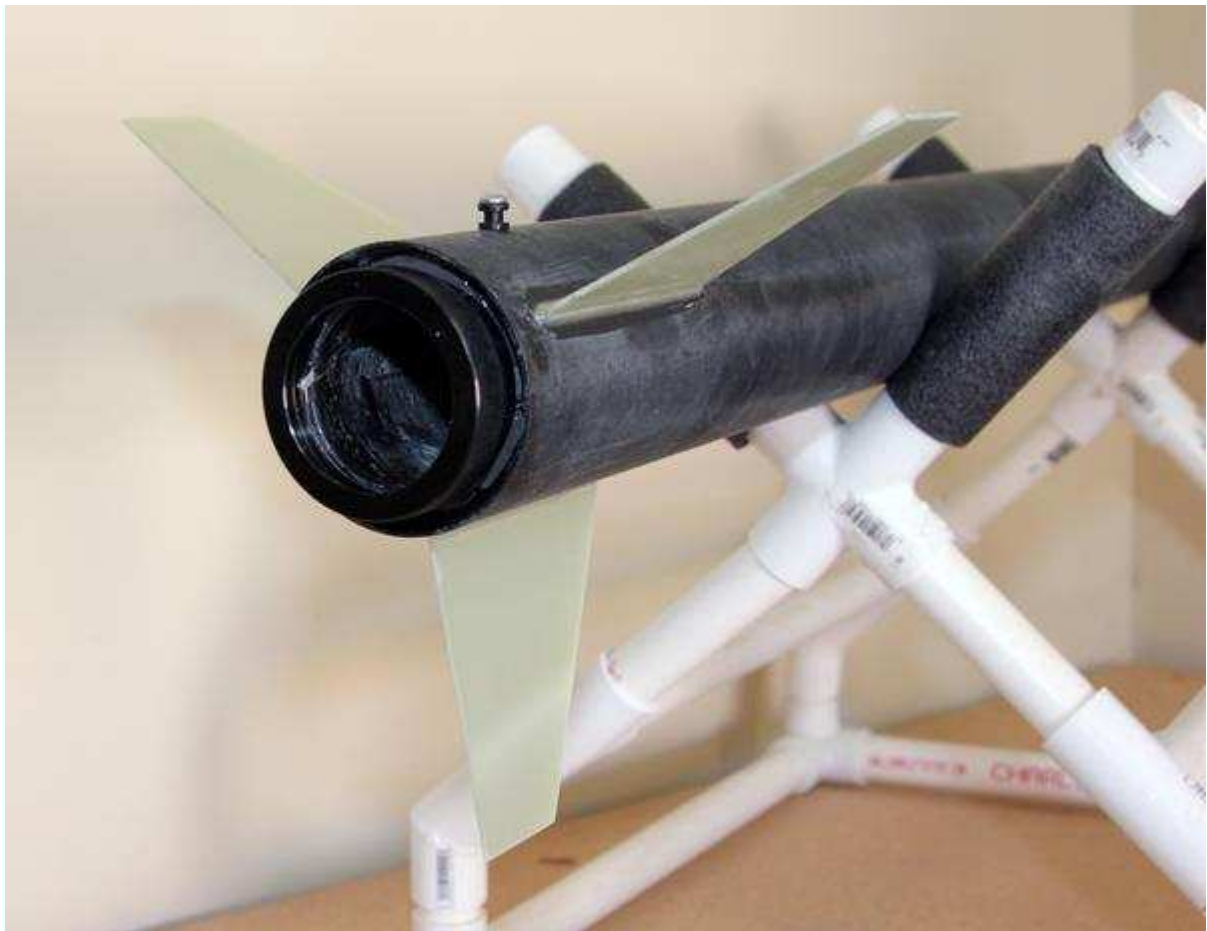
Figure 6-39. Glue the aft centering ring and motor retainer in place.
