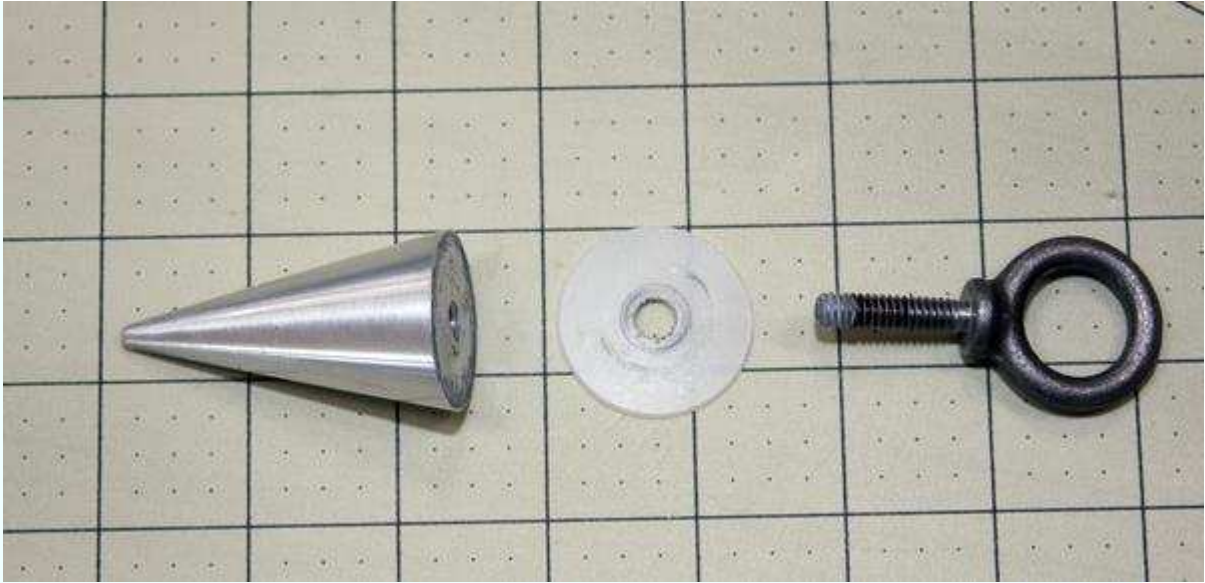
Figure 13-6. Replace the standard 1/4-20 bolt with a 1/4-20 eye bolt.
