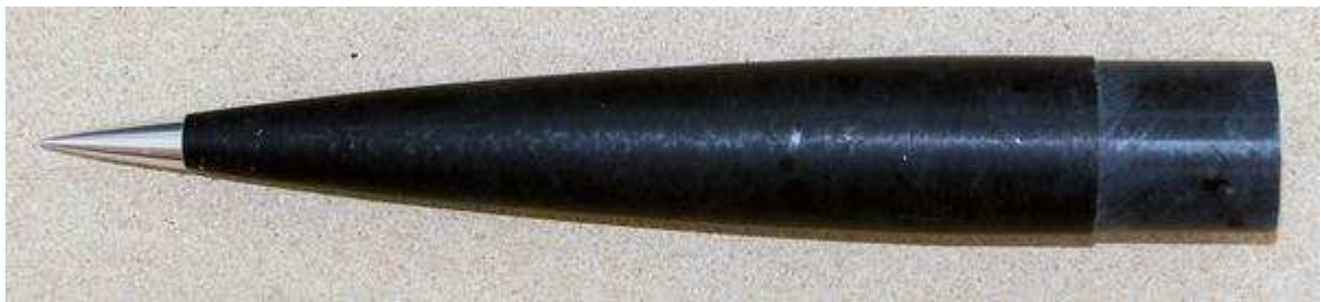
Figure 6-30. Rough up the inside of the nose cone and the outside of the tube coupler, and then glue the tube coupler into the nose cone.
