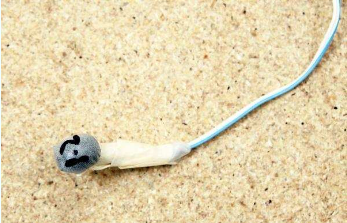
Figure 7-19. Use the finger from a disposable glove, the corner from a Doritos bag, or whatever your personal favorite happens to be to make two 1.2 g squibs.
