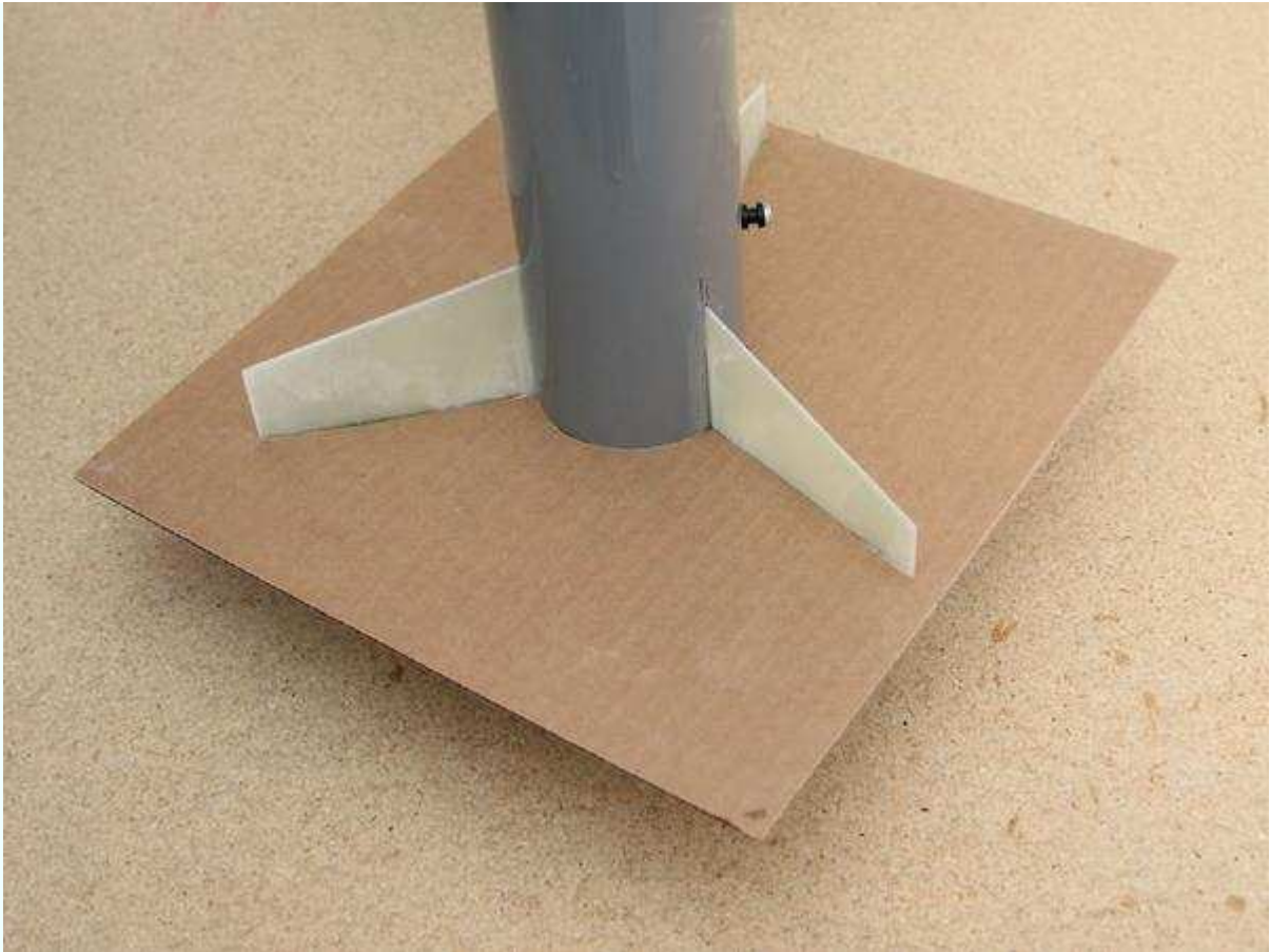
Figure 6-17. Glue the fins and forward centering ring in place.
