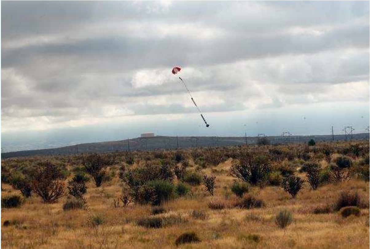
Figure 5-12. Just as the rocket lands, pick out a landmark far in the distance. Walk toward the landmark to find the rocket.
