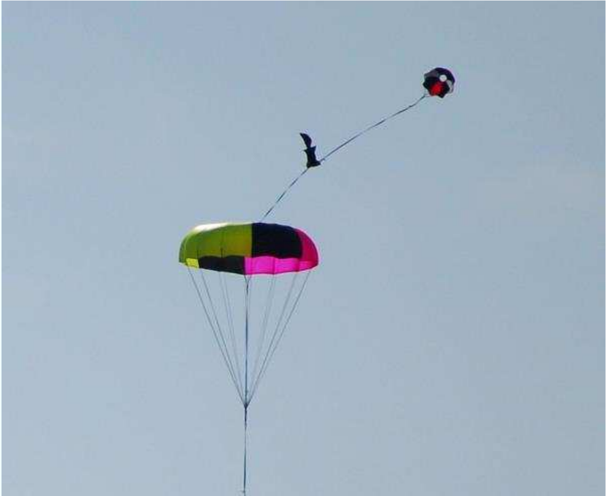
Figure 9-7. Shape does matter. While an inexpensive flat parachute has a coefficient of drag of about 0.75, this Iris Ultra from Fruity Chutes has a drag coefficient of 2.2, making it three times as efficient for the same size parachute. Photo by Fruity Chutes, used with permission.
