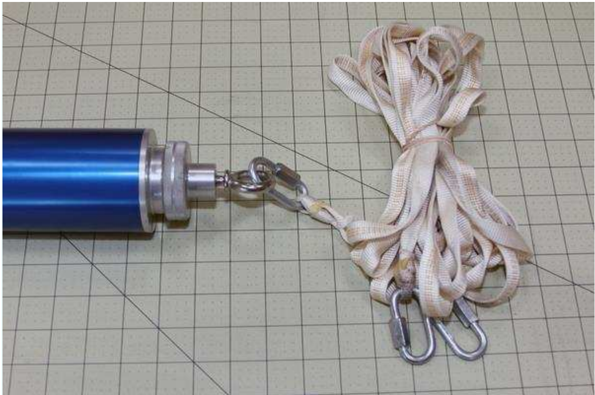
Figure 13-4. Many larger motors have a forward closure that allows a shock cord to be attached directly to the motor.
