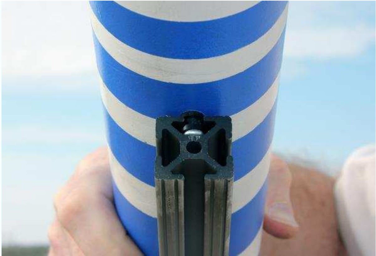
Figure 3-48. Rail buttons are designed to slide into the launch rail.
