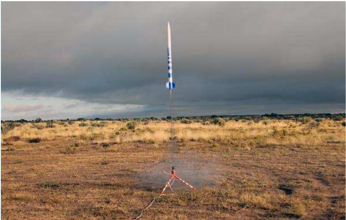
Figure 3-8. Launch lugs and rail buttons are used to guide the rocket in the first few feet of flight. This gives the rocket time to pick up speed so it is traveling fast enough for the fins to work.
