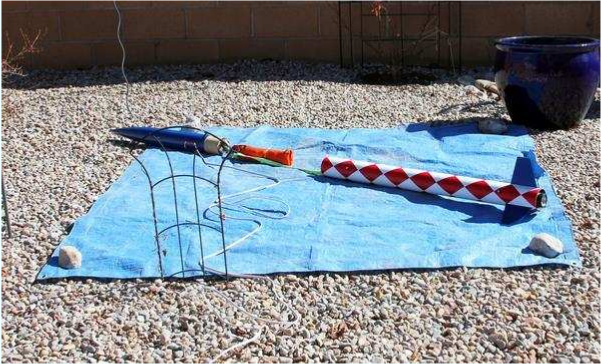
Figure 7-21. Deimos after a successful ejection charge test. The parachute is still bound in the flame blanket, wrapped in a zip tie, just as it would be for flight. The cable cutter would cut the zip tie later in the flight.
