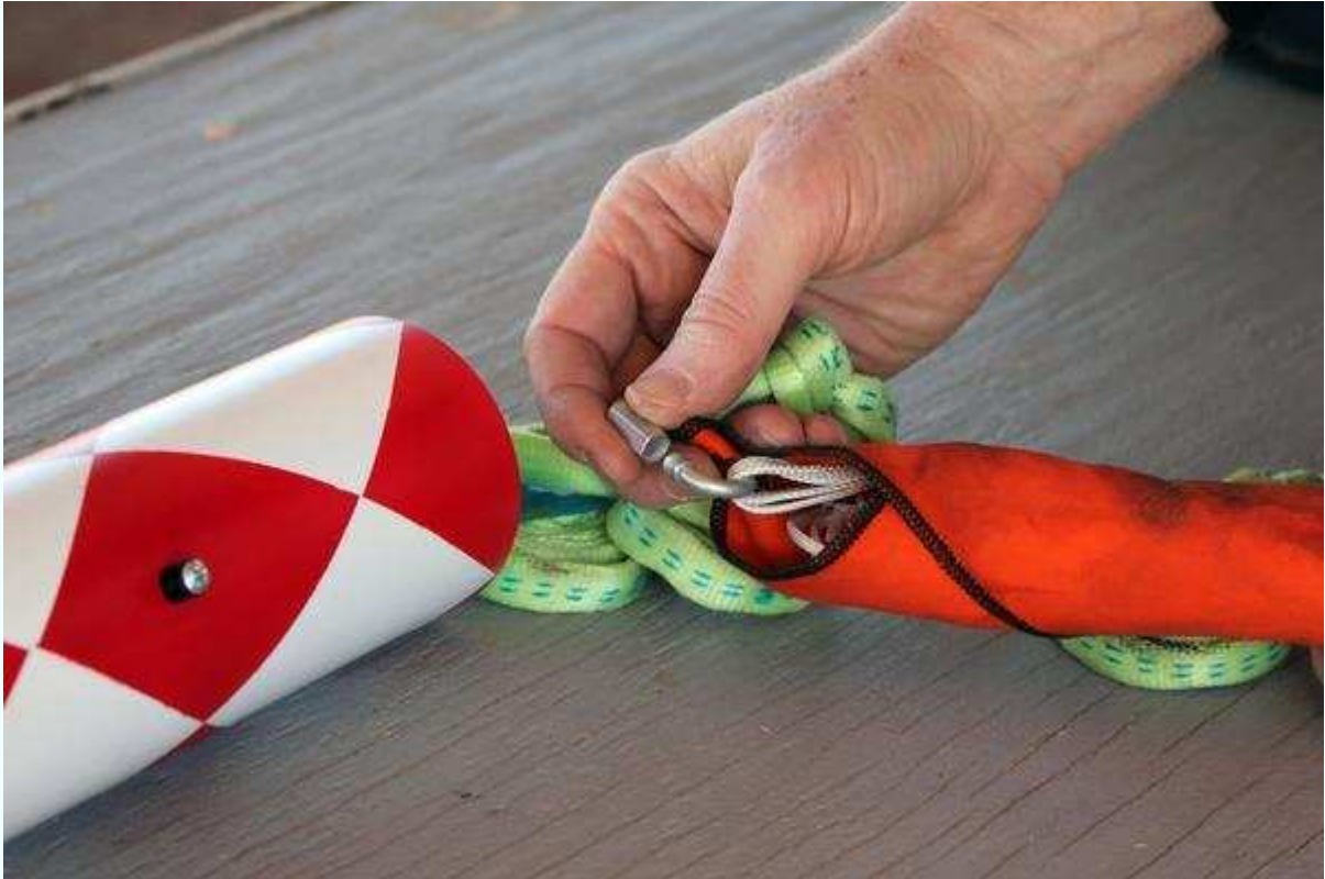
Figure 8-22. Prepare the drogue parachute.
