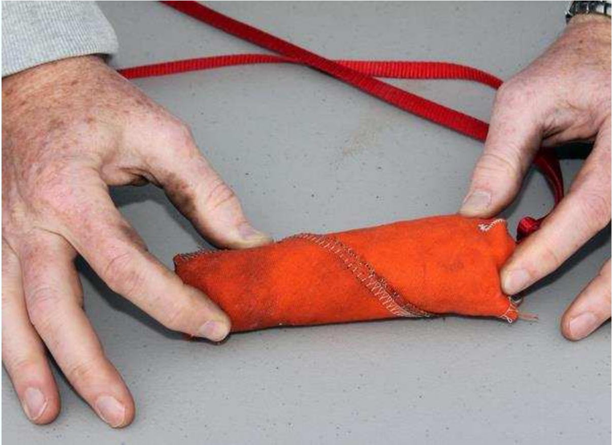
Figure 5-7. Roll the parachute to form a tight bundle that completely covers that parachute and shroud lines.
