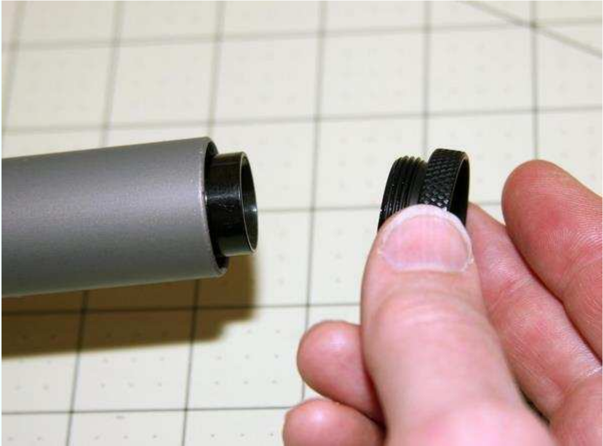
Figure 4-36. Screw the rear closure into place.
