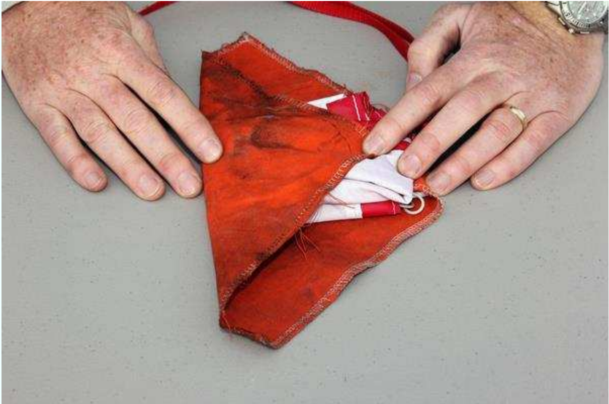
Figure 5-5. Place the parachute at the corner of the chute protector with the quick link, then fold the opposite corner across the parachute.
