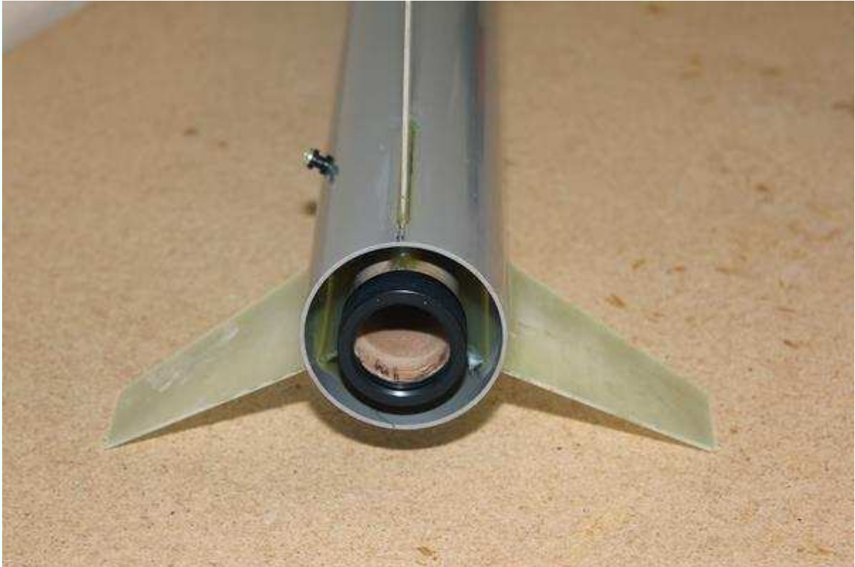
Figure 6-19. Glue the motor retainer in place with JB Weld.
