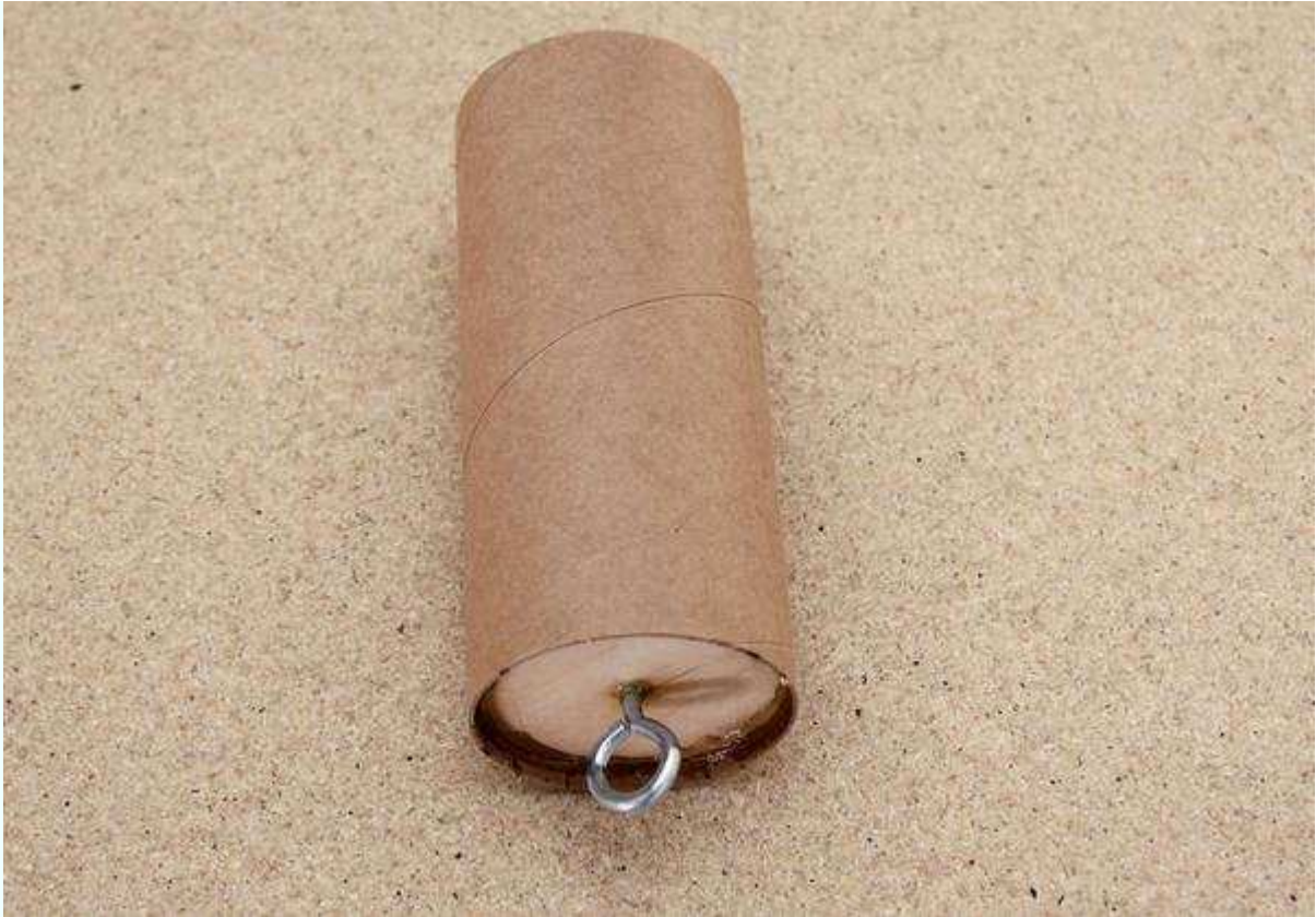
Figure 3-58. Attach the eye bolt, then glue the bulk plate 1/4" from the bottom of the tube coupler.
