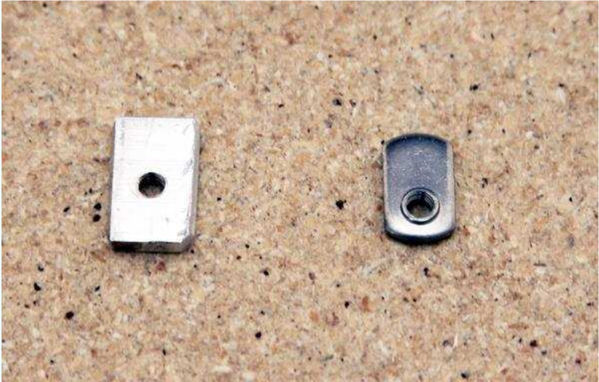
Figure 3-49. Two launch button nuts, one homemade and one commercial.
