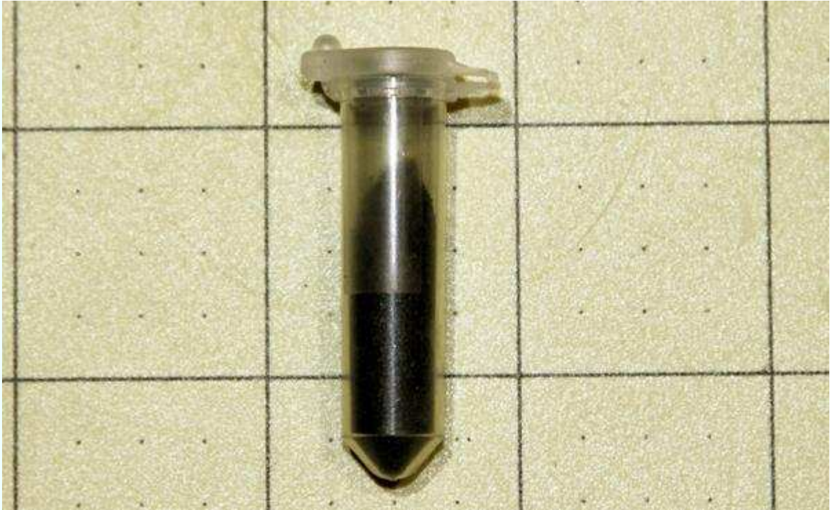
Figure 7-18. Save some vials from AeroTech ejection charges to measure black powder.
