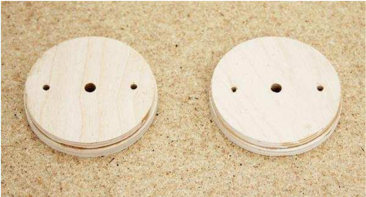
Figure 8-5. Glue the bulk plates together. Drill a 1/4" hole in the middle, and two 5/32" holes 15/16" from each center hole.
