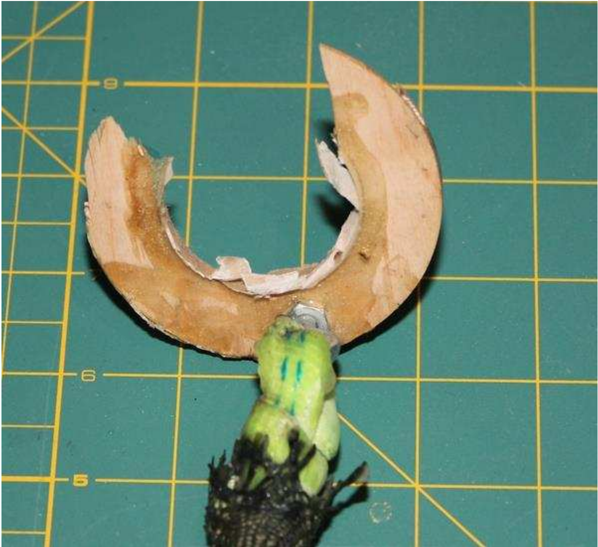
Figure 7-1. It may be called rip-stop nylon, but parachutes are not indestructible. This 48" chute ejected at about 100 ft/s.
