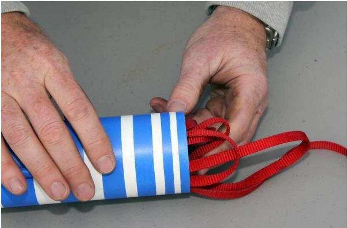
Figure 5-9. Put the shock cord in after the parachute. Seal the recovery system with the payload bay.
