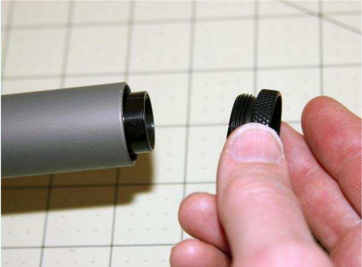
Figure 4-34. Insert the nozzle.
