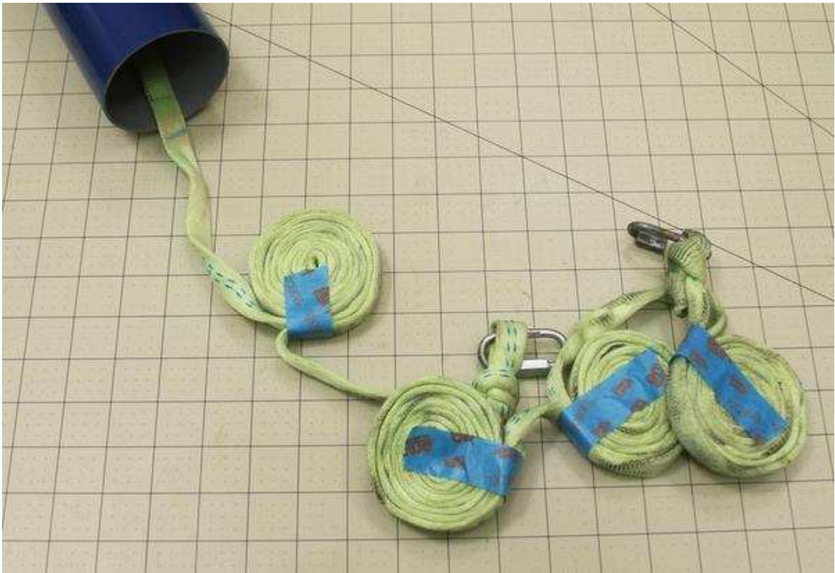
Figure 9-2. Rolling is a compact way to pack tubular nylon shock cord.
