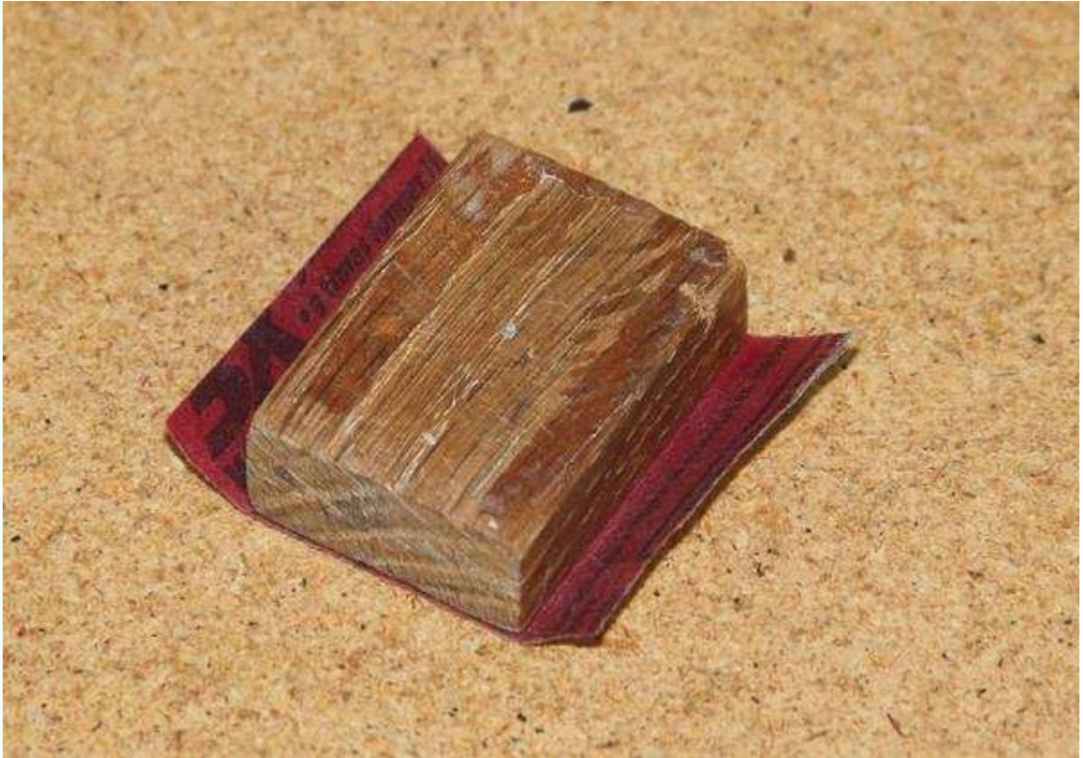
Figure 3-23. Use a sanding block to sand flat surfaces.
