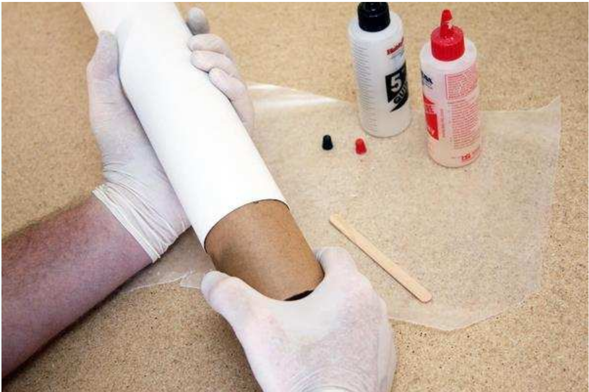
Figure 3-59. Glue the tube coupler into the 10" payload bay tube so 3" of the tube coupler sticks out.
