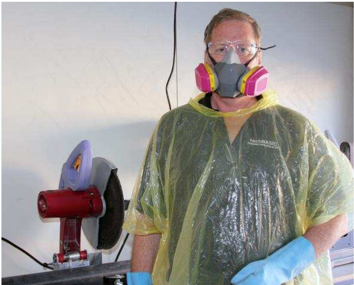
Figure 6-27. The height of fashion for working with fiberglass. Here the author is decked out in safety glasses, an OV/AG/P100 respirator, clothing protection, and hand protection. The hood of the poncho is generally up when sanding and cutting, but is down in the photo so the respirator is more visible.
