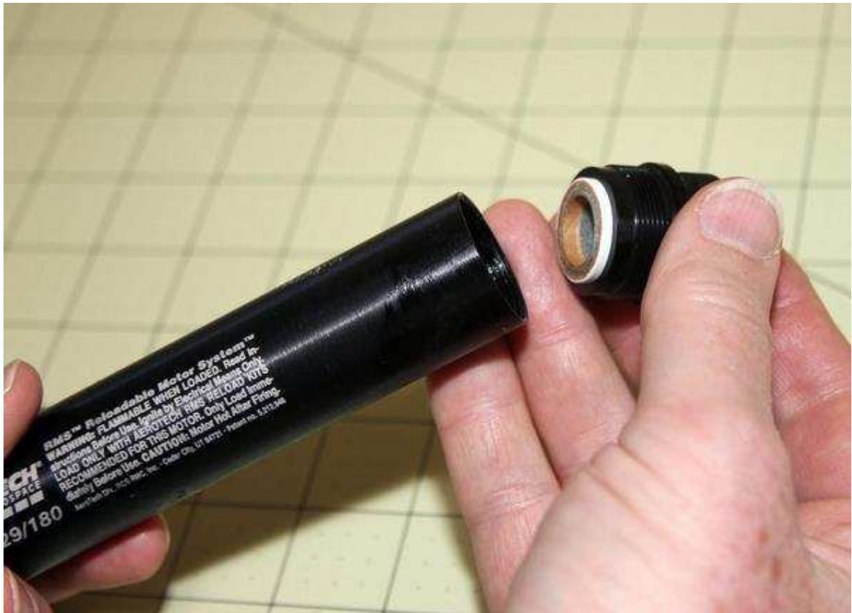
Figure 4-21. Grease the threads if they need it, then screw the forward seal into place.
