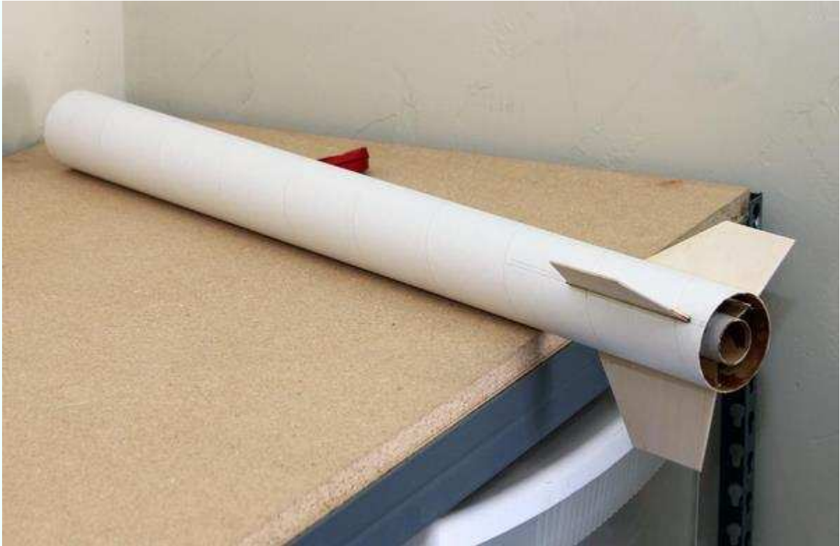
Figure 3-47. Place the rocket somewhere flat while the glue stiffens.
