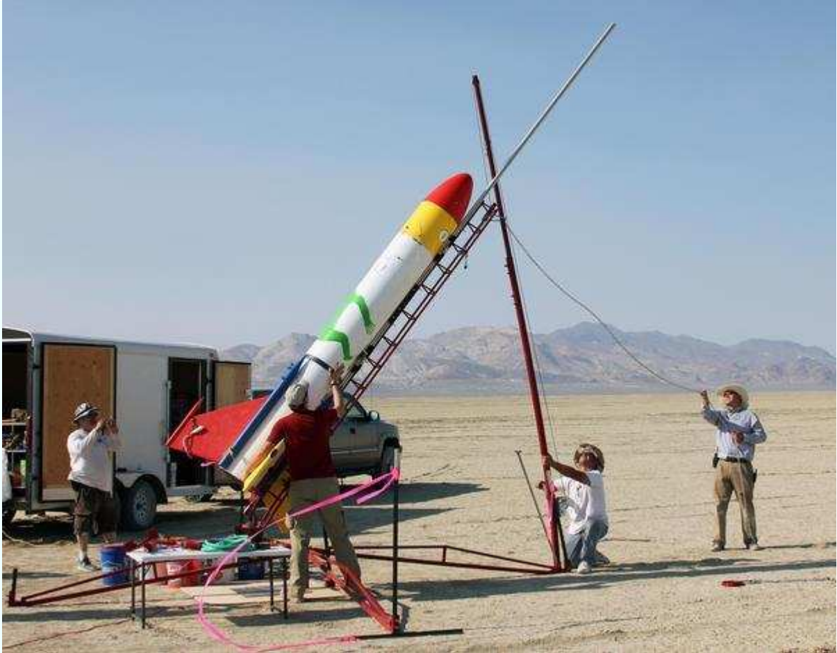
Figure 3-11. The Baby Q weighed nearly 600 pounds at liftoff, but was guided through its first moments of flight by this sturdy launcher using a launch rail reinforced with a steel tower.
