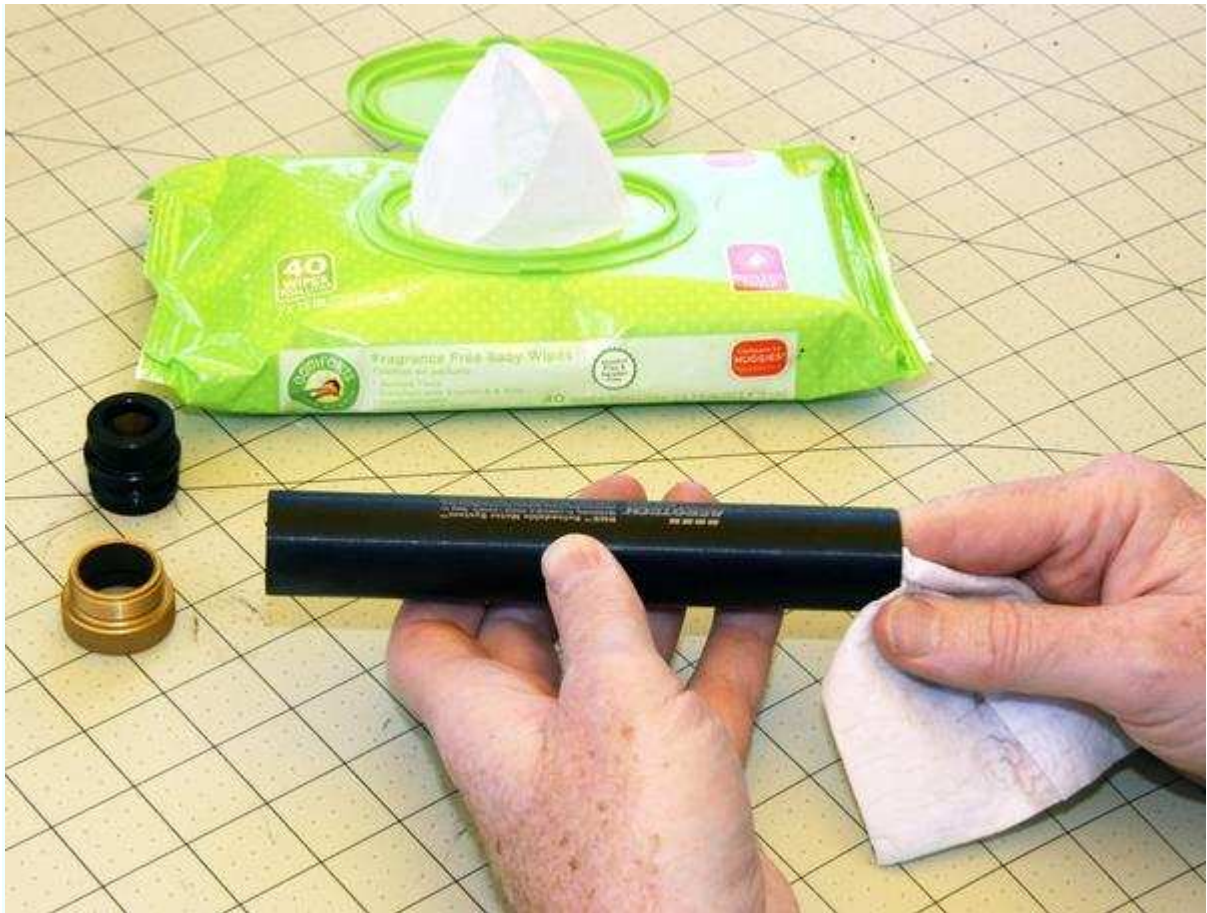
Figure 5-16. Clean the parts of all residue.
