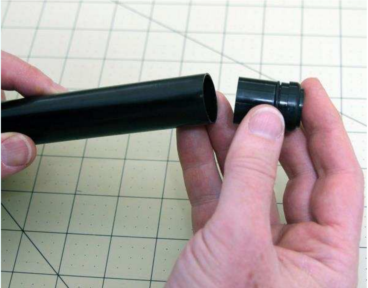
Figure 4-31. Insert the delay and ejection charge assembly.
