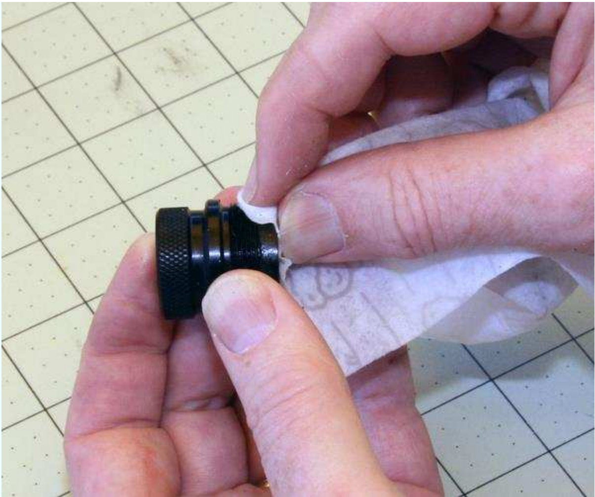
Figure 5-17. Clean threads by pressing a wipe into the thread groove and turning the part like you are unscrewing it.
