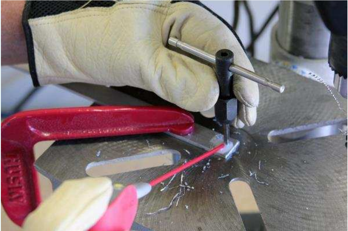
Figure 3-50. Using lubricant, drill and tap a hole near the end of an aluminum rod.
