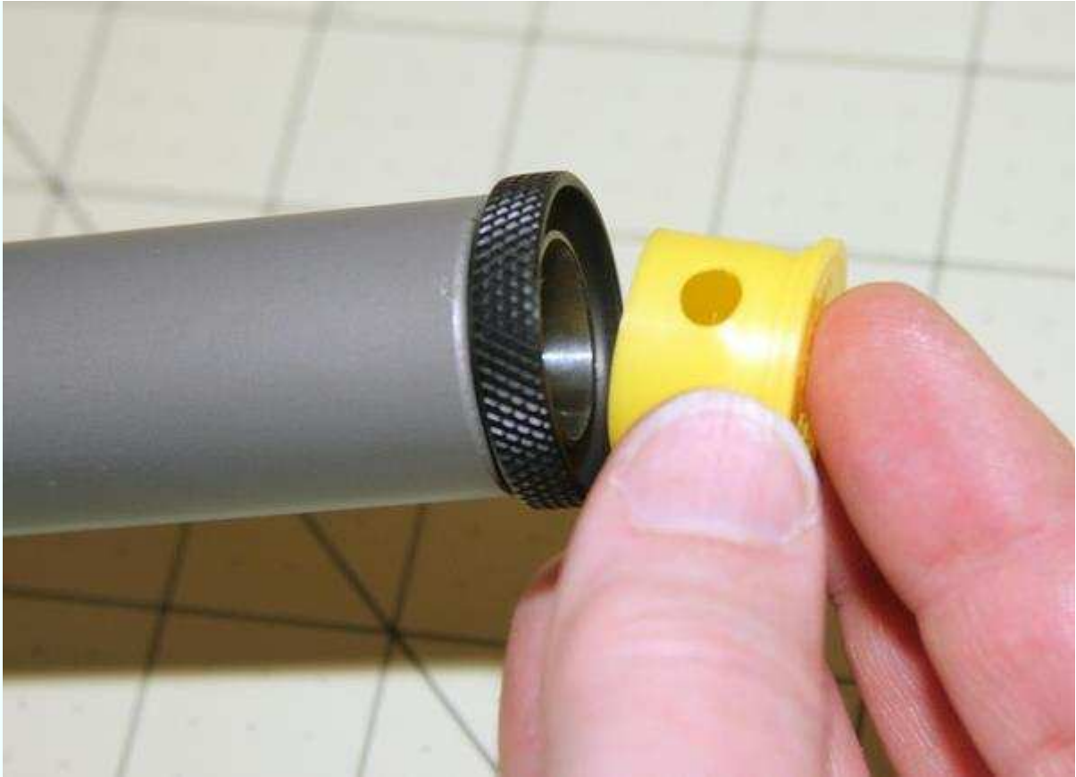
Figure 4-37. Push the plastic cap in place over the nozzle.
