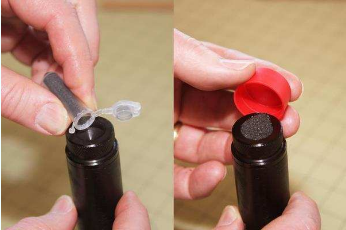
Figure 4-25. Pour 3/4 of the black powder into the top of the motor, then cap the front with the provided red plastic cup.
