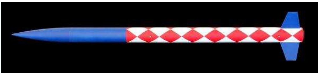
Figure 6-2. Deimos is an impressive 3"-diameter, 5-foot-long rocket that is perfect for a Level 1 or 2 certification flight.
