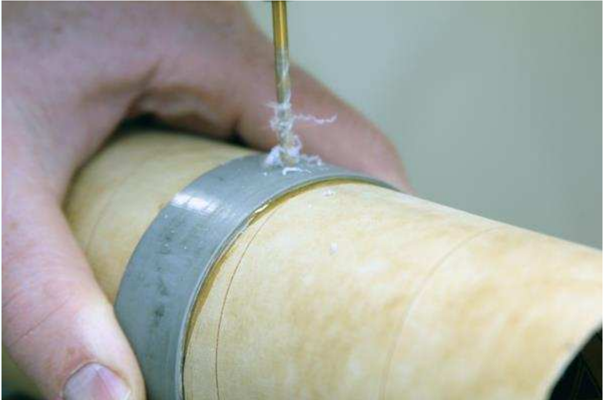
Figure 8-7. Drill three altimeter vent holes.
