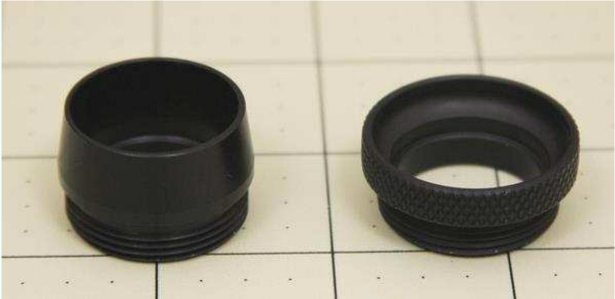
Figure 4-29. CTI uses two kinds of aft closure. On the left is the tapered closure, suitable for high-performance minimum diameter rockets. On the right is the standard closure.
