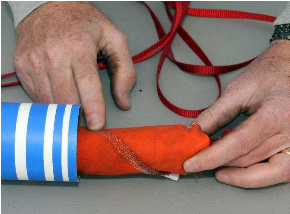
Figure 5-8. Insert the parachute bundle first.
