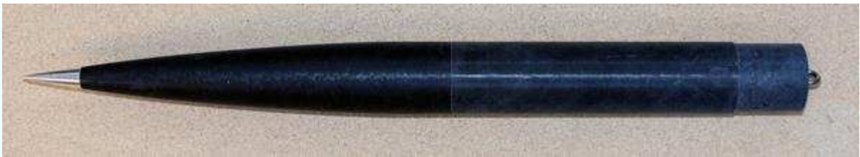
Figure 6-32. Fasten an eye bolt to a bulk plate. Roughing up all surfaces before gluing, glue the bulk plate 1/4" inside the tube coupler. Glue the tube coupler into the payload bay so 3" sticks out. Slide the nose cone into place to complete the payload section.
