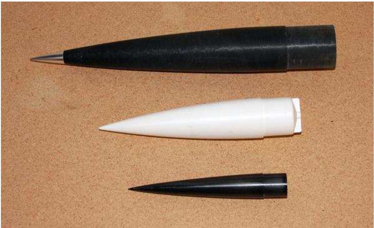
Figure 3-4. Nose cones are typically plastic, fiberglass, or carbon fiber. From top to bottom, a wound fiberglass nose cone with a metal tip, a molded plastic nose cone, and a molded fiberglass nose cone. Fiberglass and Carbon Fiber Colors
