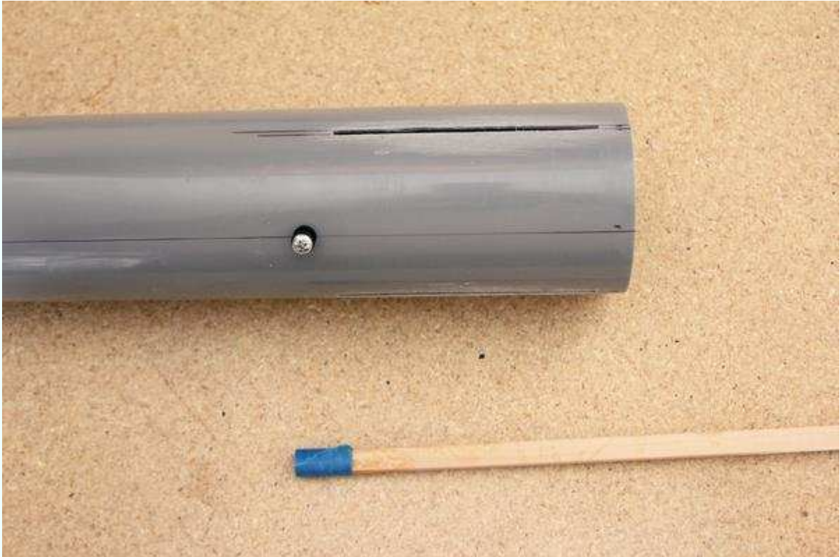
Figure 6-16. Glue the rail button nut in place on the inside of the airframe and install the rail button.
