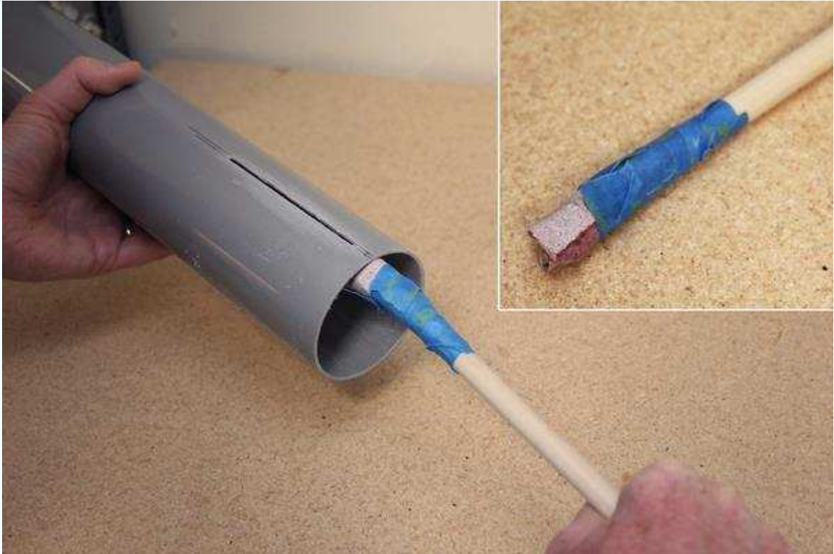
Figure 6-13. Scuff all areas of the tube where glue will be applied. Don't forget the inside of the rocket, especially the area where the centering rings will be glued.
