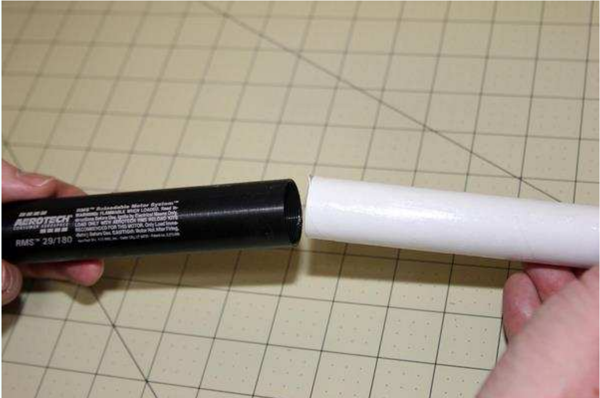
Figure 4-18. Slide the motor liner and fuel grains halfway into the motor case.
