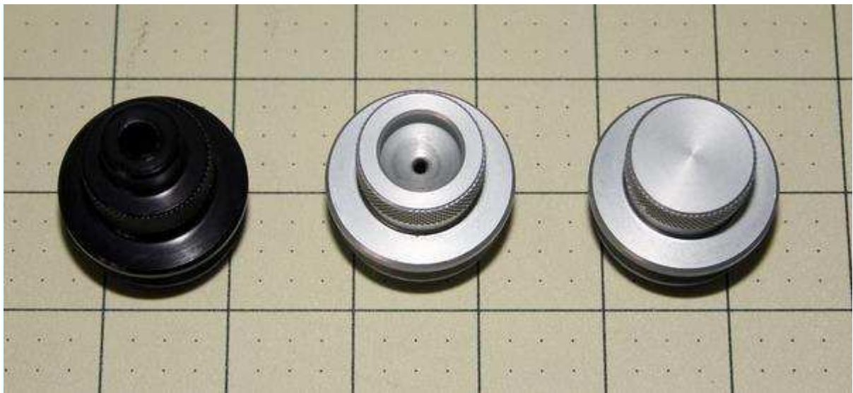
Figure 4-7. There are three closure styles for most AeroTech motor sizes. From left to right are the tapped forward closure, a closure used with ejection charges, and a sealed forward closure.
