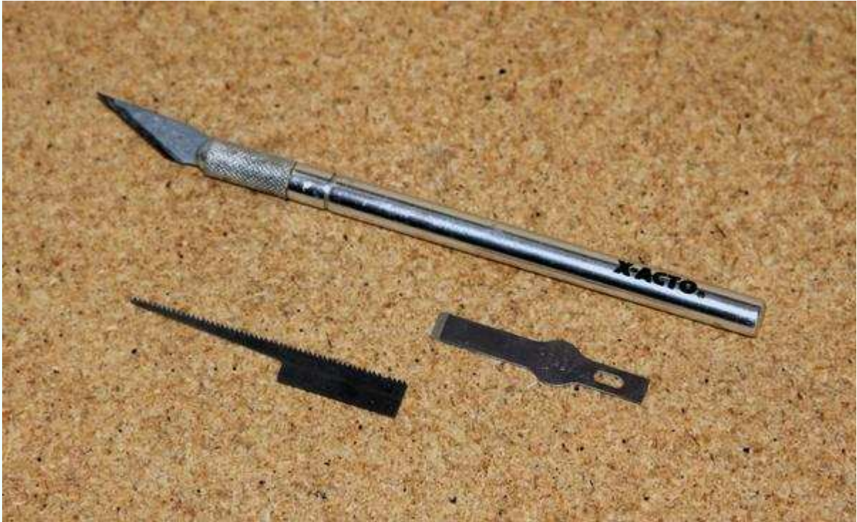
Figure 3-17. A hobby knife is essential. A nice set is very handy. Shown here are a standard #11 blade in the knife handle, a keyhole saw blade, and a scraper blade.
