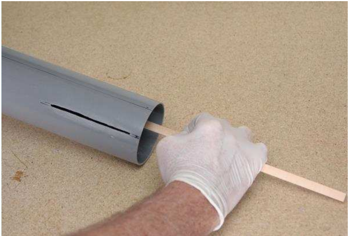
Figure 6-14. Apply glue so the forward centering ring will slide through the glue as you push it into place, forming a nice fillet.
