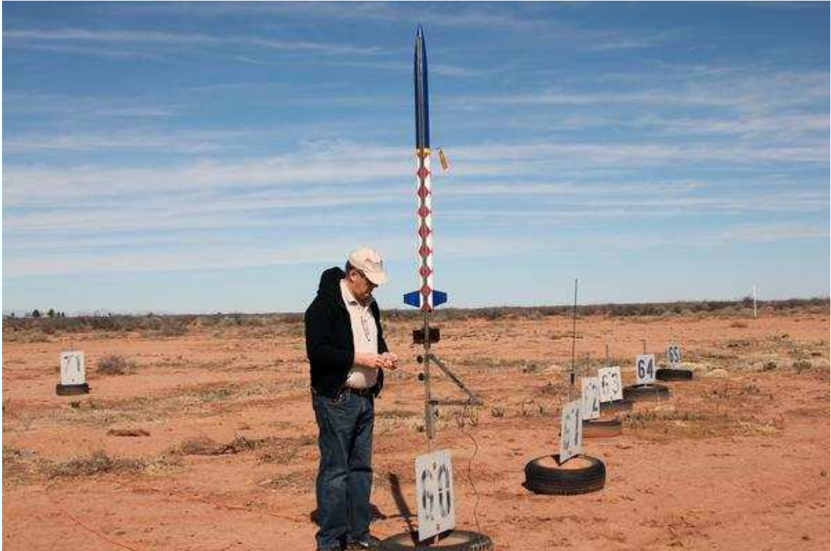
Figure 8-15. The author installing an igniter in a J350 motor before the first dual-deploy flight of Deimos.
