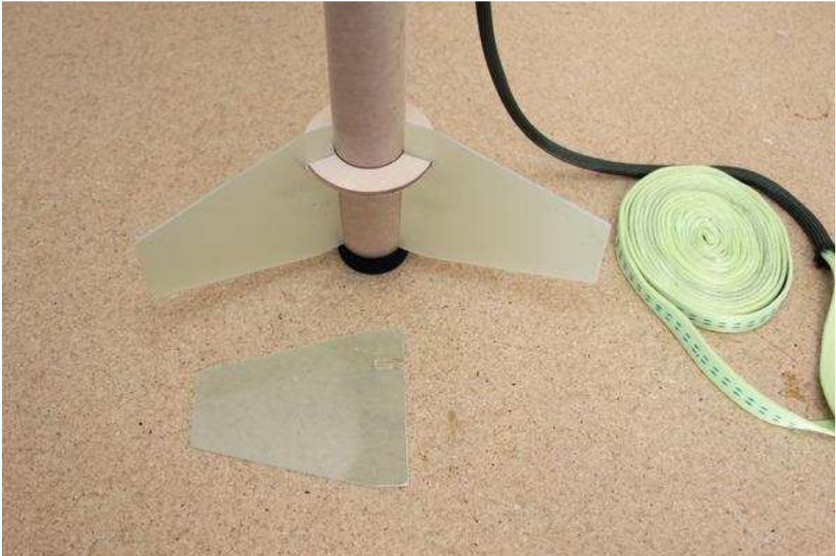
Figure 6-12. Here's how the fins and centering ring will be positioned in the finished rocket.
