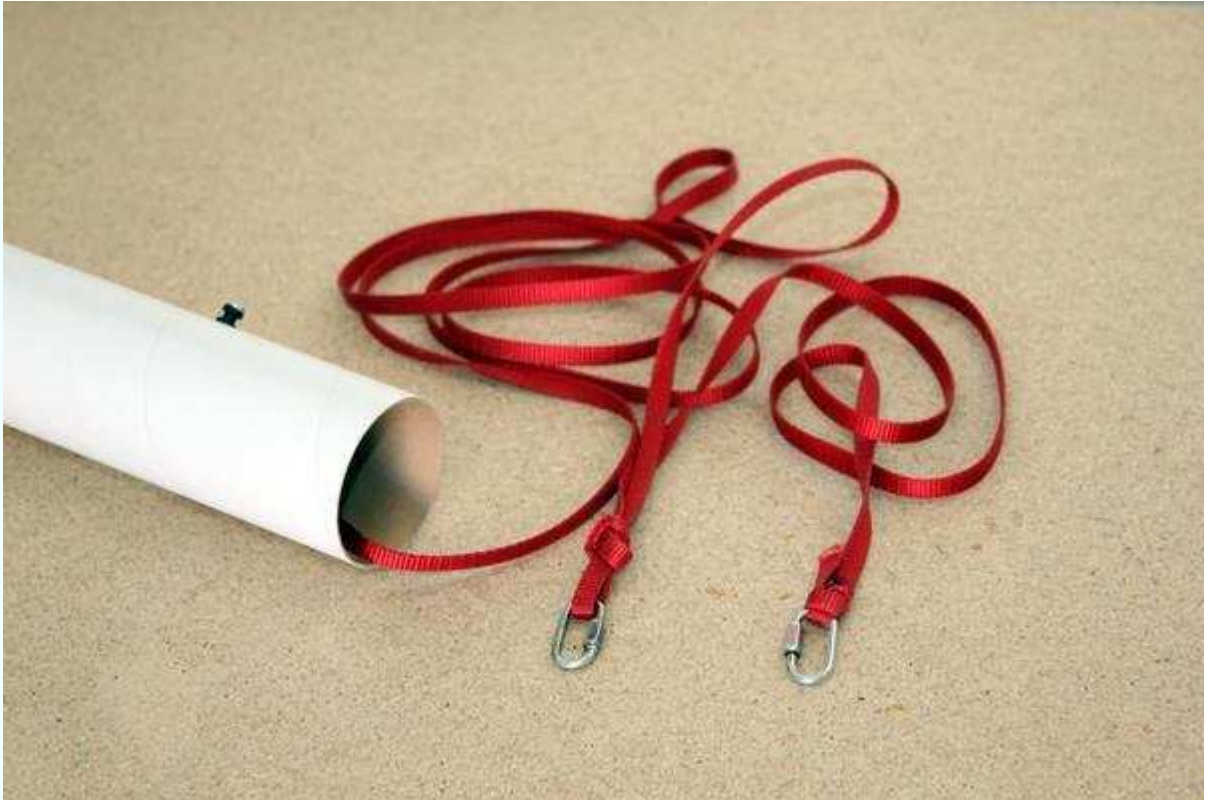
Figure 3-57. Attach one quick link to the end of the shock cord and the other about 1/3 of the way from the end.
