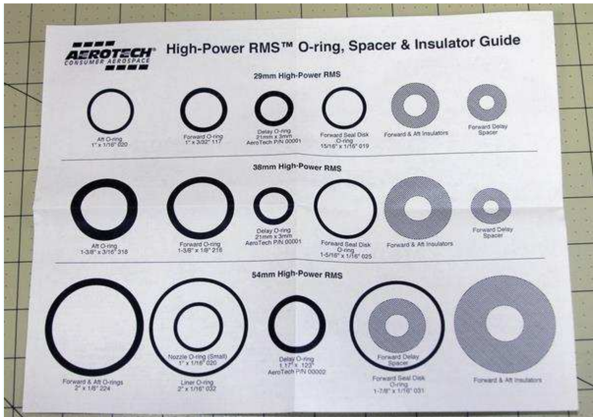
Figure 4-9. Lay the O-rings and disks on the provided guide to make it clear which part is which.
