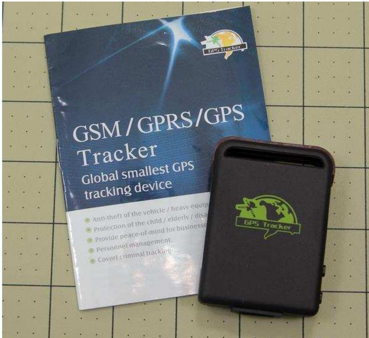
Figure 10-21. Many GPS devices can be repurposed for use in rocketry.
