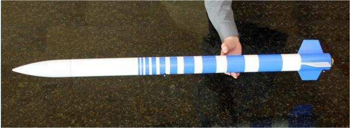
Figure 3-62. Measure the actual center of gravity by balancing the rocket on your finger.
