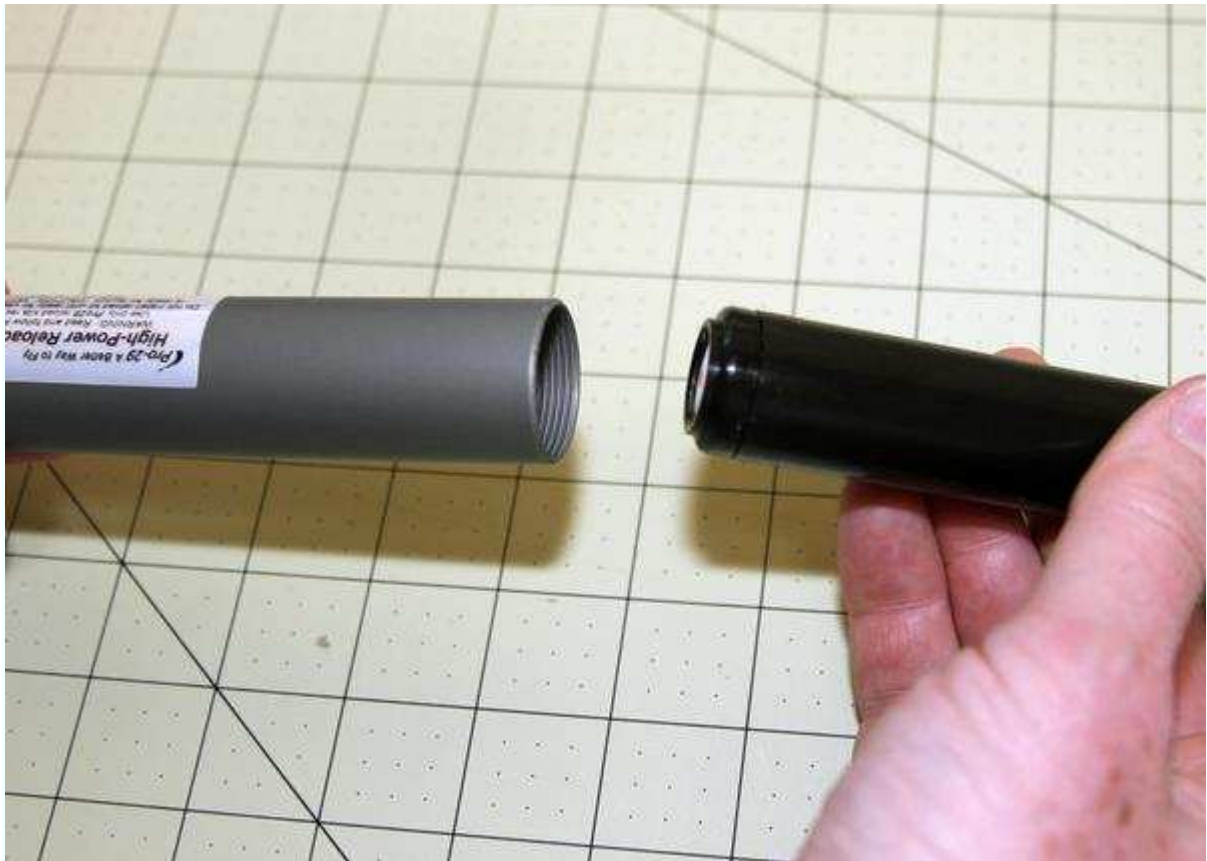
Figure 4-35. Insert the reload in the motor case, ejection charge first.
