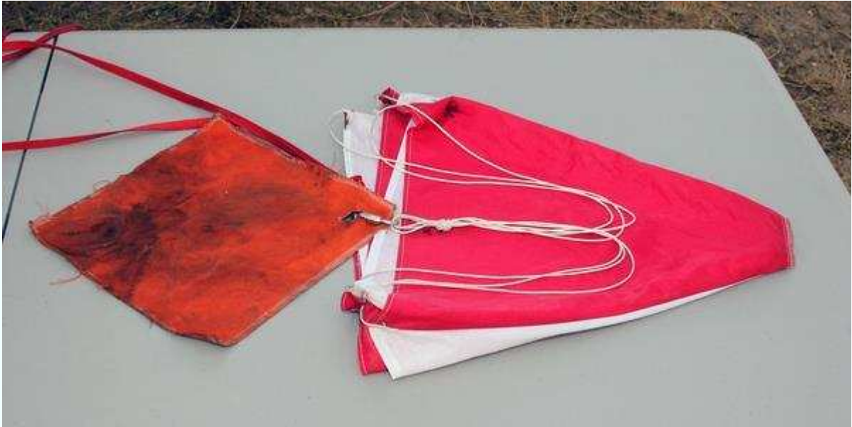
Figure 5-3. Fold the parachute and shroud lines. Connect the parachute protector, shock cord, and parachute using the middle quick link.
