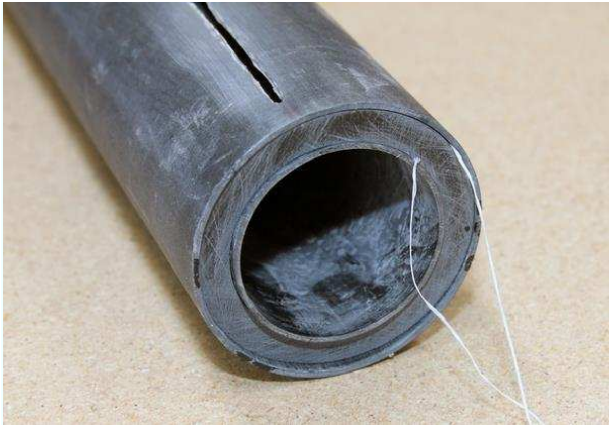
Figure 6-37. Glue the forward centering ring in place, using the aft centering ring to guarantee perfect alignment. Notice that the centering ring and fin slot have been roughened with sandpaper so the glue holds better.
