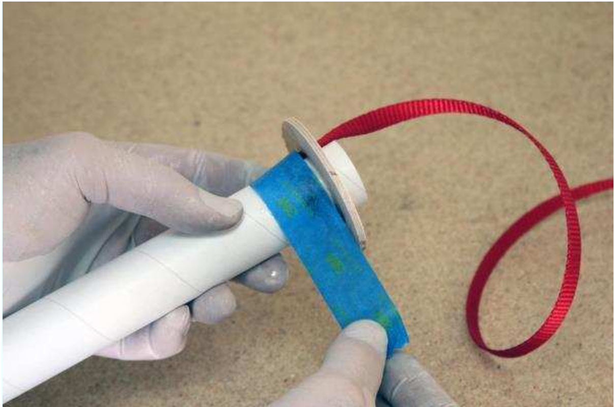
Figure 3-38. Wrap tape around the shock cord to hold it in place while the glue dries.
