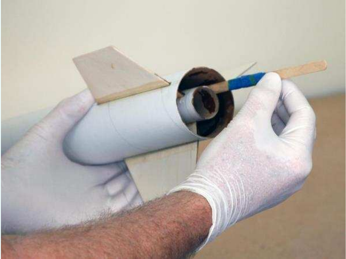
Figure 3-45. Work copious amounts of 30-minute epoxy into the interior fillet locations, tipping the rocket to help it flow into place.
