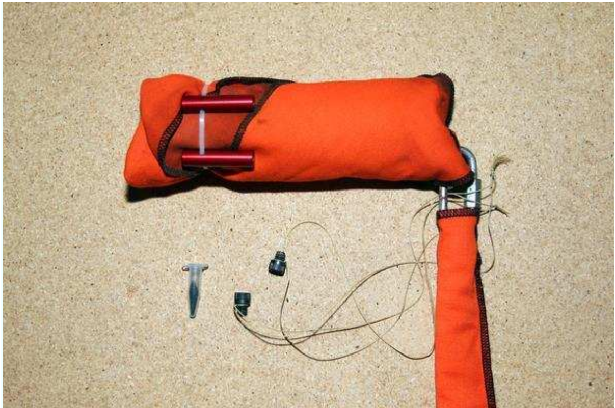
Figure 7-23. Attach the cable cutters so either one can cut the zip tie holding the parachute closed.
