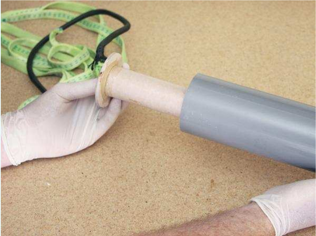
Figure 6-15. Slide the motor mount through the glue, then push the aft centering ring just inside the bottom of the rocket to keep the motor tube centered while the glue sets.
