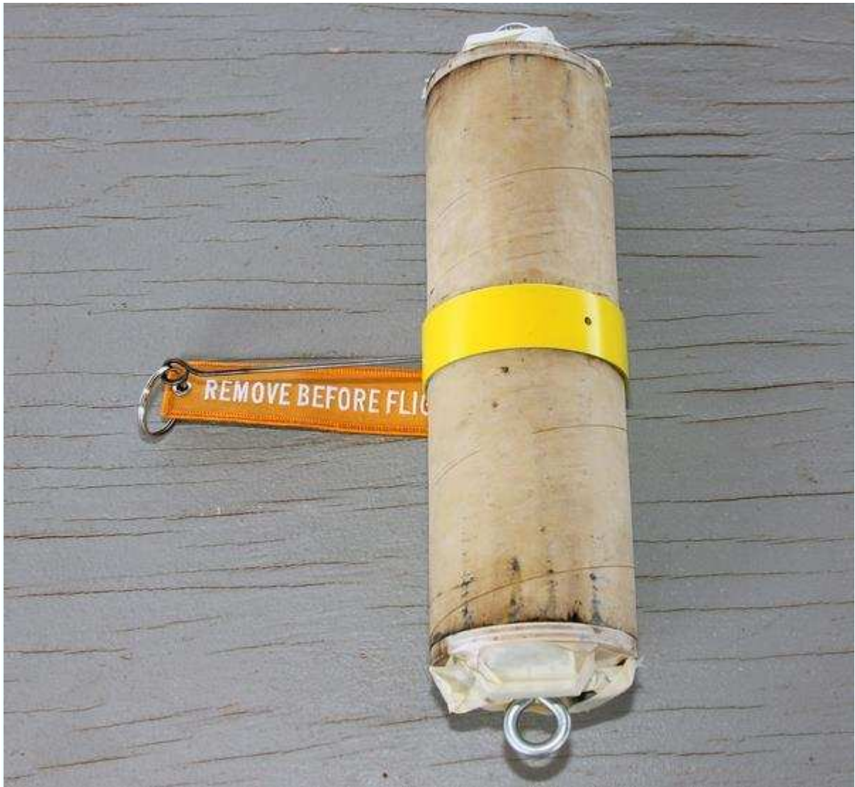
Figure 8-20. Connect the electronics and insert the arming pin first, then install the black powder charges.
