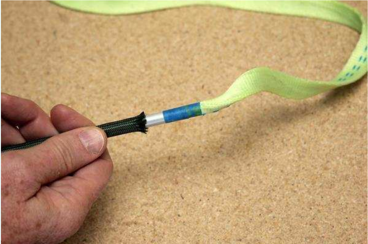
Figure 6-10. Cut a 20-foot length of tubular nylon and a 2-foot length of Nomex. Using an aluminum tube or dowel, push the Nomex tubing onto the tube. Tape the tube to the tubular nylon, and then slide the Nomex onto the tubular nylon.
