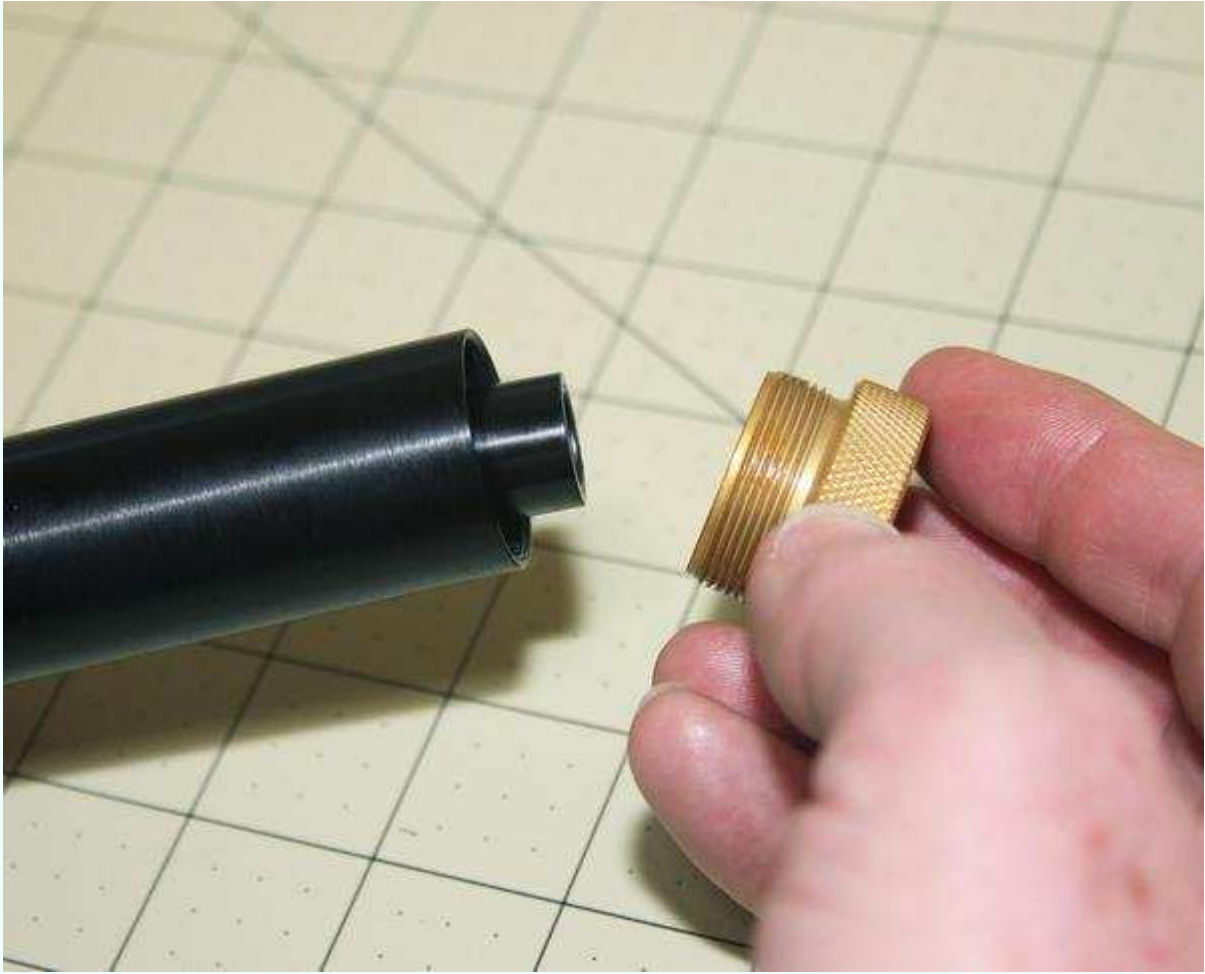
Figure 4-24. Screw the aft seal into place.
