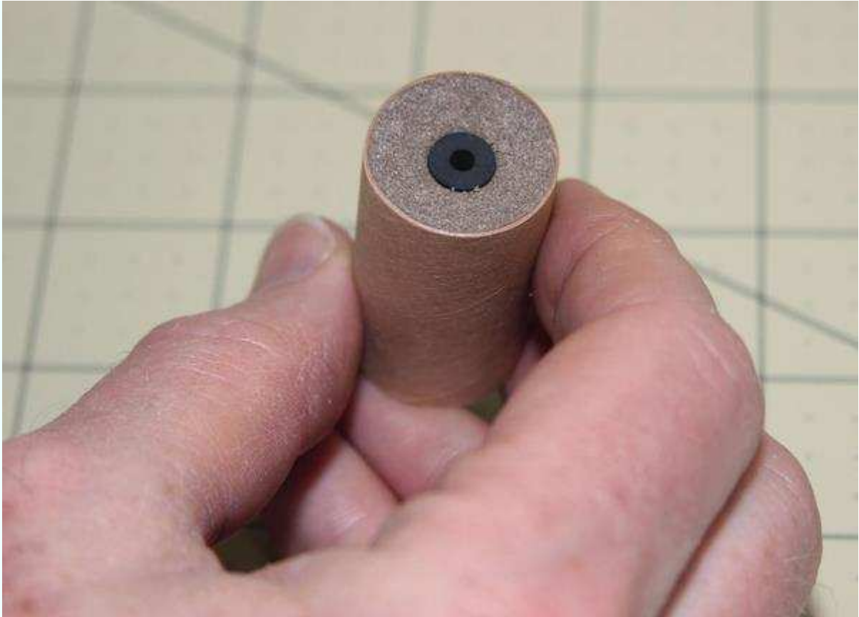
Figure 4-32. Insert the grain with the Pyrodex pellet first, with the pellet facing the delay charge.
