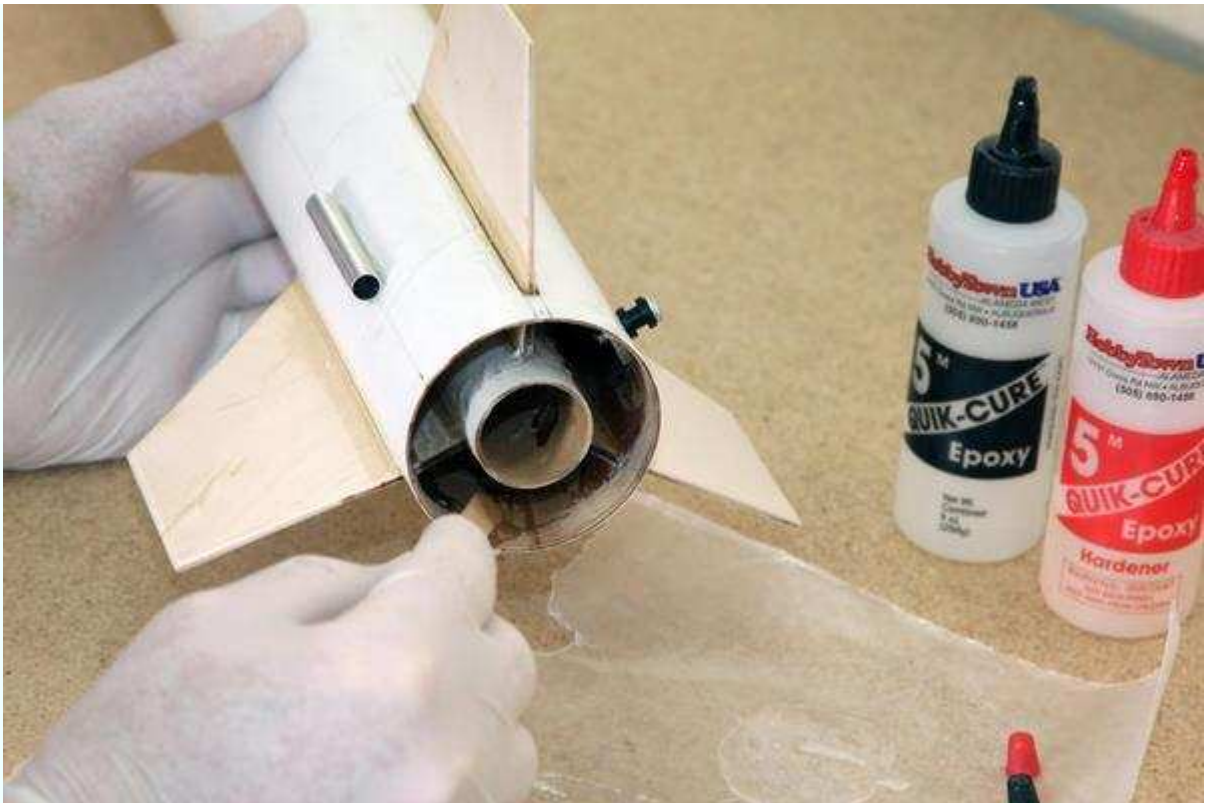
Figure 3-53. Smear a generous amount of glue inside the airframe tube, then slide the centering ring all the way against the fins.
