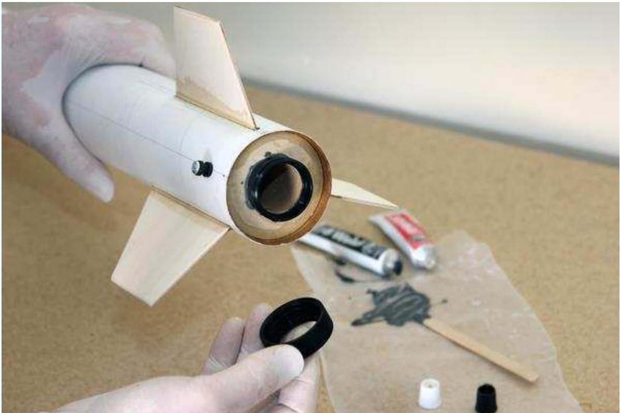
Figure 3-55. Install the motor retainer using JB Weld or some other heat-resistant epoxy.
