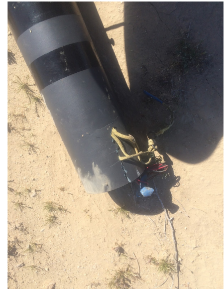
Figure 27: Zippering on Main Deployment
