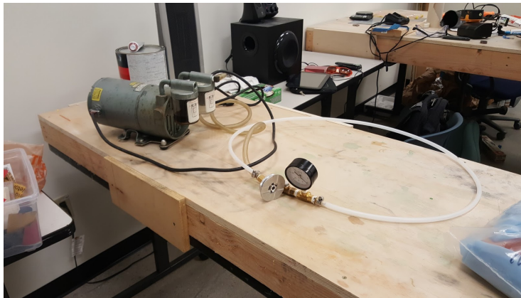
Figure 22. Pump used for the altimeter testing
