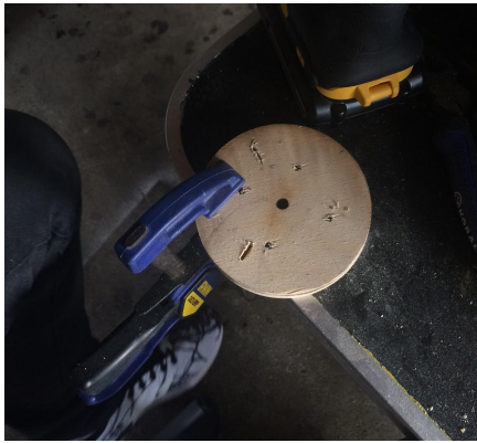
Figure 9. Bulkplate for Fin Mounting System
