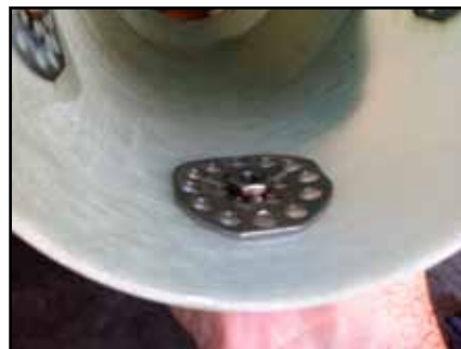
Figure 4: Bend so the curve matches the inside of the tube.
