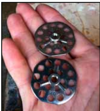
Figure 1: Welded nut plates with holes for epoxy.
