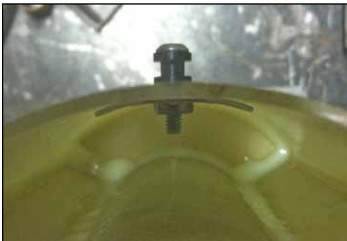
Figure 2: A rail button installed into a fiberglass tube using a welded nut plate.
