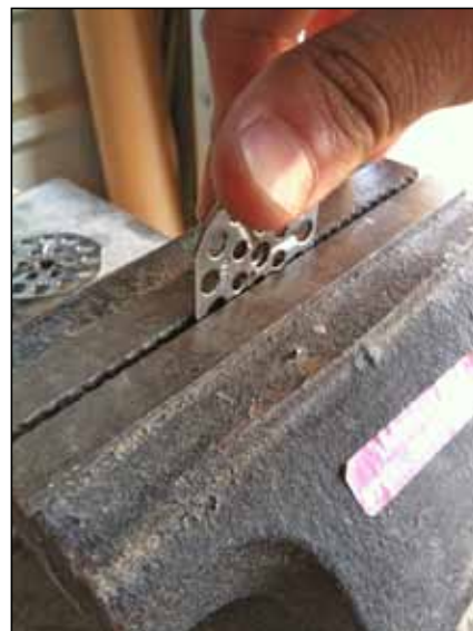
Figure 3: Bend lightly. It is easy to over bend the metal.
