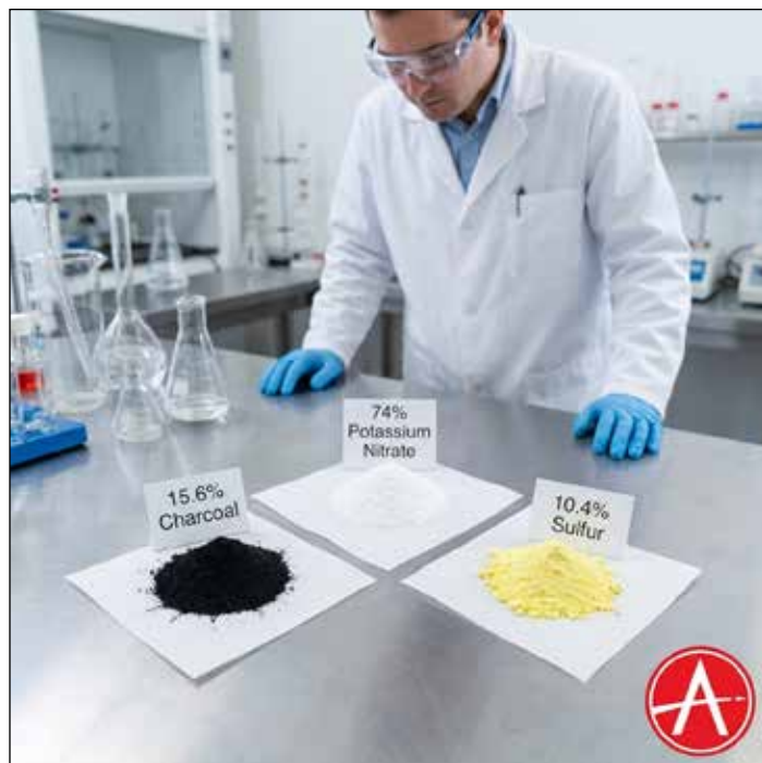
Figure 2 - Chemical components of black powder.
