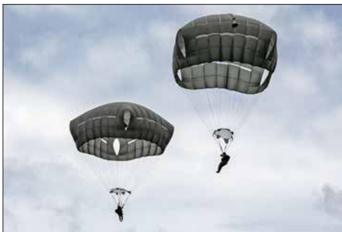
Figure 5. The T-11 paratrooper parachute has a complex canopy structure. What is the reference area here? The square top? The total “wetted” area? The reference area must be specified when providing a drag coefficient of a parachute (DoD photo).
