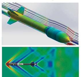
With competition scoring placing an enormous achieving emphasis on the exact specified objective altitude of 10,000 feet, accurate altitude prediction for the rocket is crucial. Incorporating fluid dynamics computational into the design process allows for accurate altitude more predictions under variable flight conditions, and has been instrumental in providing quantitative performance metrics during the development of this year's new aerobraking mechanism.
