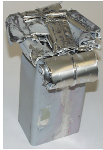
Aluminum double-chamber after dynamic impact
