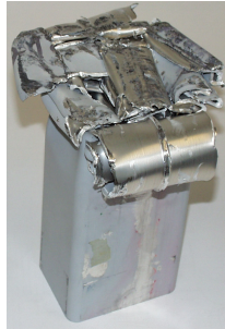
Aluminum double-chamber after dynamic impact
