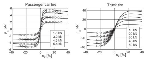
Figure 3.8: Longitudinal force: o Meas., - TMeasy
