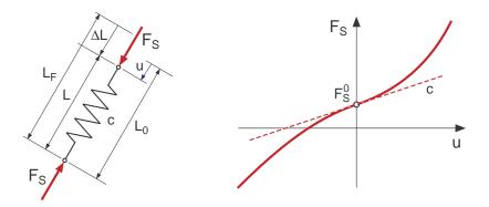
Figure 6.2: Linear coil spring and general spring characteristics
