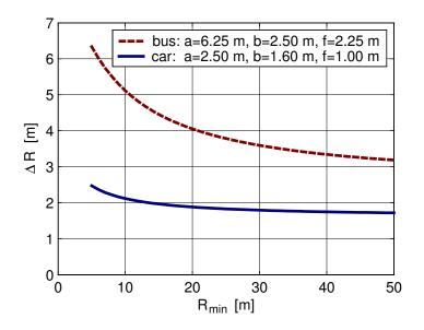
Figure 9.3: Space requirement of a typical passenger car and bus
