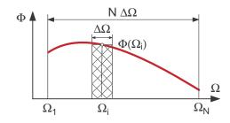
Figure 2.5: Power spectral density in a finite interval
