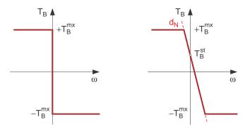
Figure 4.5: Coulomb Dry Friction Model and Enhanced Brake Torque Model
