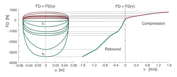
Figure 6.6: Damper characteristics generated from measurements, [12]
