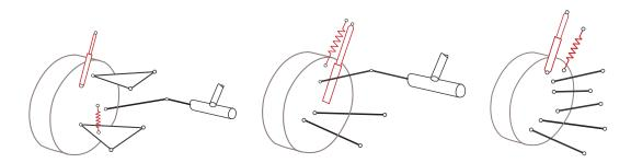
Figure 5.1: Double wishbone, McPherson and multi-link suspension
