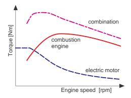
Figure 4.12: Hybride drive torque characteristics
