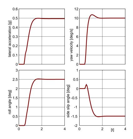
Figure 10.3: Step Steer: Passenger Car at  $v = 100 \ km/h$
