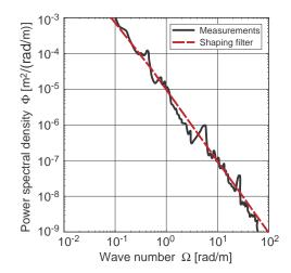
Figure 2.8: Shaping filter as approximation to measured psd
