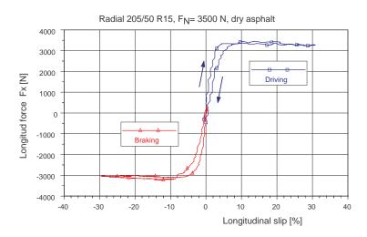
Figure 3.5: Typical results of tire measurements
