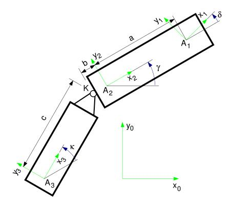
Figure 9.4: Kinematic model with trailer
