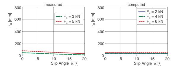
Figure 3.47: Measured [12] and computed bore torque relaxation length:  $c_{\varphi} = 1200 Nm/rad$ ,  $d_{\varphi} = 1.2 Nm/(rad/s)$ ,  $r_D |\Omega| = 60 km/h$
