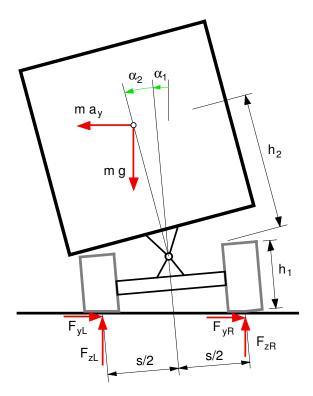
Figure 9.7: Overturning hazard on trucks
