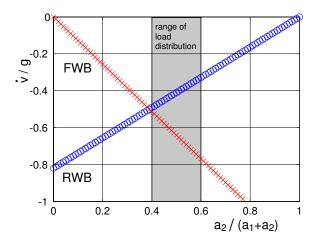
Figure 8.5: Single axle braked passenger car:  $\mu = 1$ , h = 0.55 m,  $a_1 + a_2 = 2.5 m$
