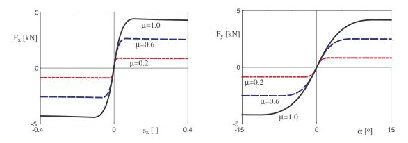
Figure 3.35: Force characteristics at different friction coefficients,  $\mu = \mu_L/\mu_0$
