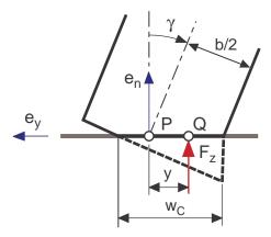
Figure 3.17: Lateral deviation of contact point at partial contact
