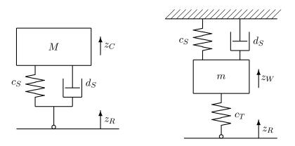
Figure 7.3: Simple Vertical Vehicle Models
