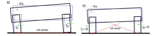
Figure 9.10: Roll behavior at cornering: a) without and b) with camber compensation
