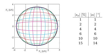
Figure 3.42: Combined forces,  $F_z = 3.5 \ kN$
