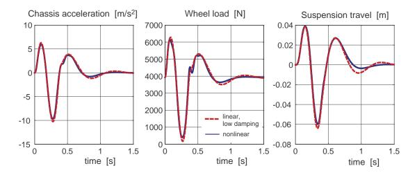
Figure 7.14: Results for low damping compared to nonlinear model
