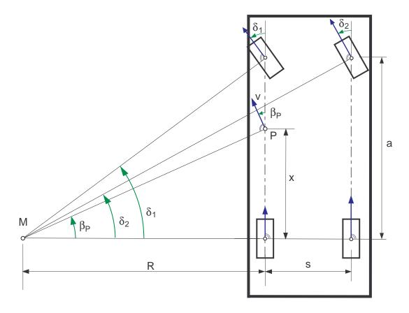
Figure 9.1: Ackermann steering geometry at a two-axled vehicle
