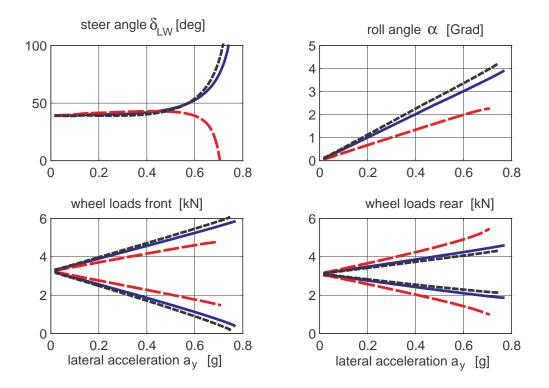
Figure 10.10: Steady state cornering, — semi-trailing arm, - - single wishbone,  $\cdots$  trailing arm
