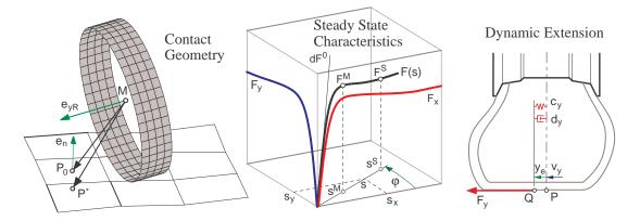
Figure 3.7: Handling tire model: TMeasy [8]
