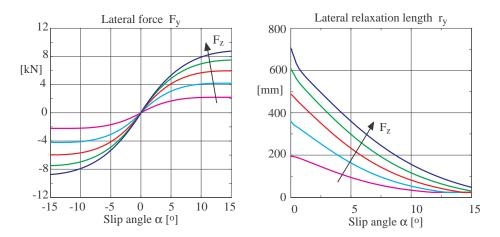
Figure 3.45: Lateral force characteristics and relaxation length, computed with  $c_y = 180\,000N/m$ ,  $d_y = 250N/(m/s)$ ,  $r_D|\Omega| = 60km/h$  at different wheel loads  $F_z = 1.75, 3.50, 5.25, 7.00, 8.75 \ kN$
