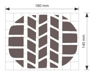
Figure 3.1: Footprint of a test tire of size 205/55 R16 at  $F_z = 4700 N$  and p = 2.5 bar
