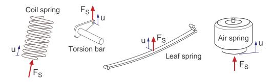
Figure 6.1: Vehicle suspension springs
