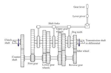
Figure 4.8: Manual transmission
