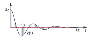
Figure 7.7: Evaluating a damped vibration
