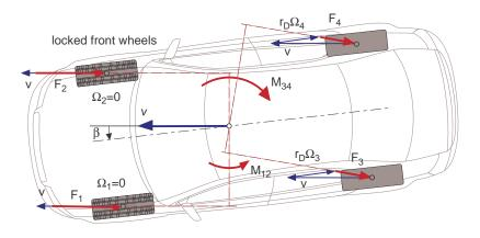
Figure 8.6: Locked front wheels
