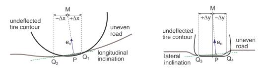
Figure 3.13: Inclination of local track plane in longitudinal and lateral direction
