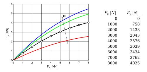
Figure 9.16: Lateral force  $F_y$  over wheel load  $F_z$  at different slip angles
