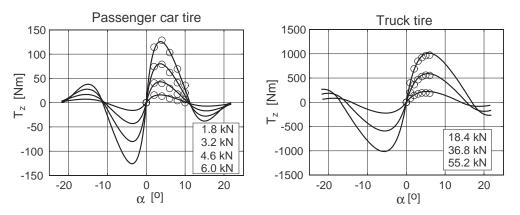
Figure 3.10: Self aligning torque: • Meas., - TMeasy
