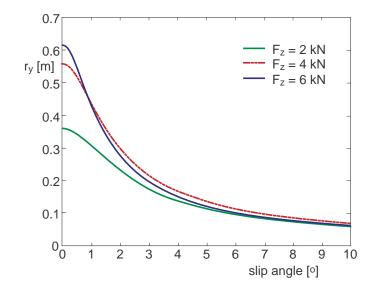
Figure 3.43: Measured lateral force relaxation length for a typical passenger car tire, [12]
