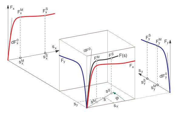
Figure 3.39: Generalized tire characteristics
