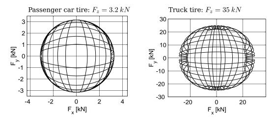
Figure 3.11: Two-dimensional characteristics:  $|s_x| = 1, 2, 4, 6, 10, 15\%;; |\alpha| = 1, 2, 4, 6, 10, 14^{\circ}$
