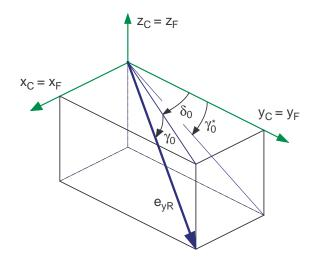
Figure 5.6: Design position of wheel rotation axis
