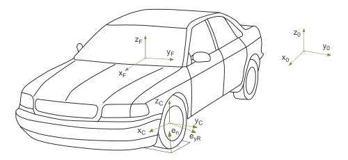
Figure 1.3: Frames used in vehicle dynamics
