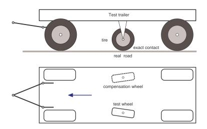
Figure 3.3: Layout of a tire test trailer
