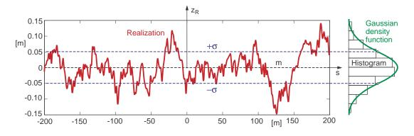
Figure 2.4: Road profile and statistical properties
