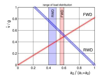
Figure 8.4: Single axle driven passenger car:  $\mu = 1$ , h = 0.55 m,  $a_1 + a_2 = 2.5 m$
