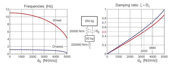
Figure 7.9: Quarter car model with standard damper
