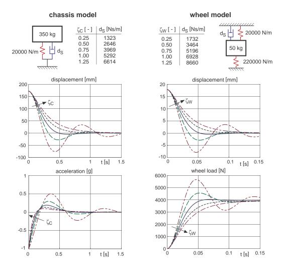
Figure 7.6: Time response of simple vehicle models to initial disturbances
