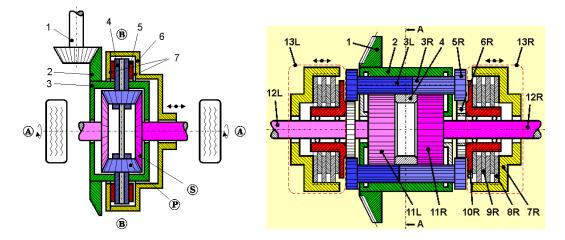
Figure 4.7: Active differentials with friction cage and multi-plate clutch
