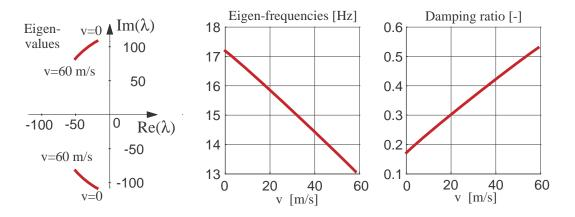
Figure 4.3: Wheel tire eigendynamics:  $\Theta = 1.2 \ km^2$ ,  $r_S = r_D = 0.3 \ m$ ,  $dF_0 = 100\ 000\ N/-$ ,  $c_x = 160\ 000\ N/m$ ,  $d_x = 500\ N/(m/s)$
