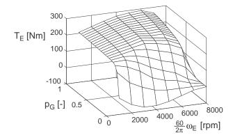
Figure 4.11: Example for a combustion engine torque:  $T_E = T_E (\omega_E, p_G)$
