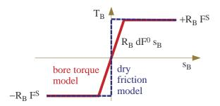
Figure 3.32: Simple nonlinear bore torque model
