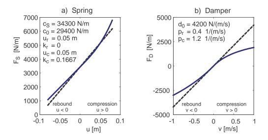
Figure 7.12: Spring and damper characteristics: - - - linear, — nonlinear
