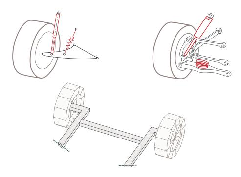
Figure 5.3: Specific wheel/axles suspension systems
