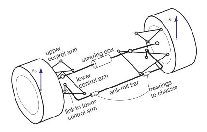
Figure 6.3: Axle with anti-roll bar attached to lower control arms
