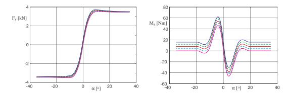
Figure 3.38: Camber influence on lateral force and torque:  $\gamma = 0, 24, 6, 8^{\circ}$
