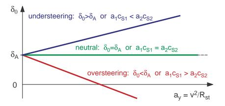
Figure 9.14: Steering angle versus lateral acceleration
