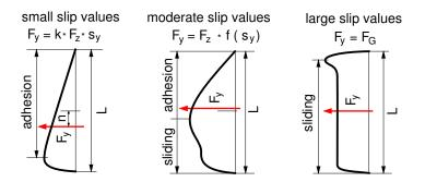
Figure 3.28: Lateral force distribution over contact patch
