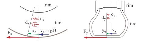
Figure 3.44: Tire deflection in longitudinal and lateral direction
