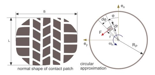
Figure 3.31: Bore torque approximation
