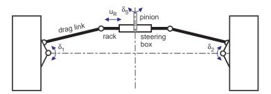
Figure 5.10: Rack and pinion steering
