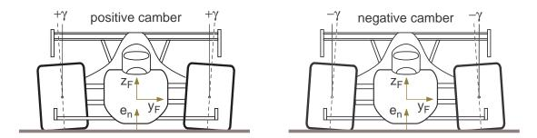
Figure 5.5: Positive camber angle
