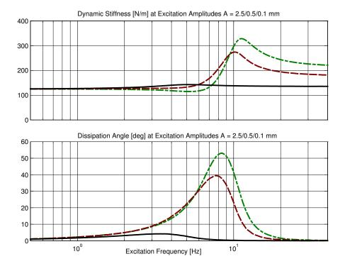
Figure 6.12: Dynamic Stiffness [N/mm] and Dissipation Angle [deg] for a Hydro-Mount
