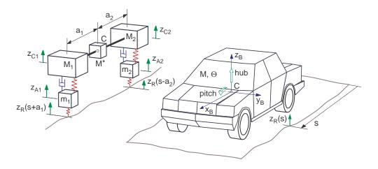
Figure 7.2: Vehicle Model for Basic Comfort and Safety Analysis
