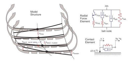
Figure 3.6: Complex tire model (FTire)
