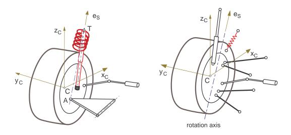
Figure 5.8: McPherson and multi-link wheel suspensions
