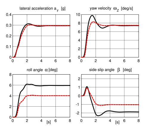
Figure 10.8: Step steer input: -- coach empty, -- coach fully occupied
