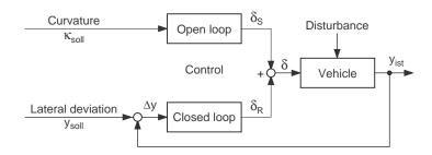
Figure 1.1: Two-level control driver model [16]
