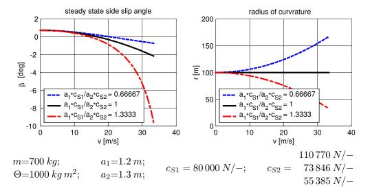
Figure 9.15: Side slip angle at steady state cornering
