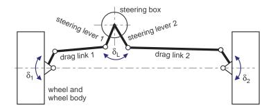
Figure 5.11: Lever arm steering system
