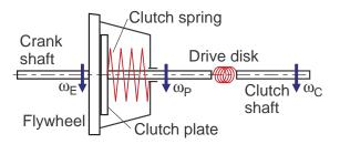
Figure 4.9: Clutch model without clutch pedal mechanism
