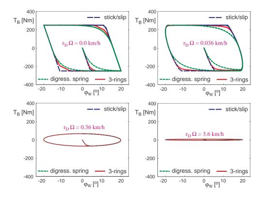
Figure 3.49: Parking torque at different driving velocities
