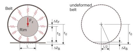
Figure 3.18: Length of contact patch
