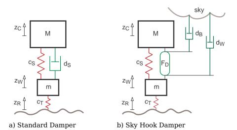
Figure 7.8: Quarter Car Model with Standard and Sky Hook Damper
