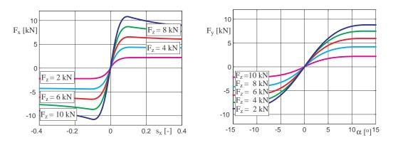
Figure 3.33: Tire characteristics at different wheel loads
