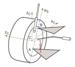
Figure 5.7: Double wishbone wheel suspension
