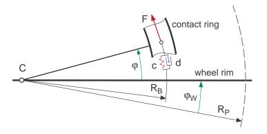
Figure 3.46: Simple bore torque model
