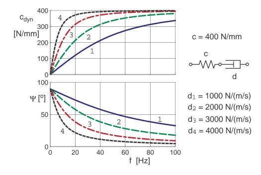
Figure 6.9: Frequency response of a spring damper combination
