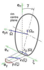
Figure 3.36: Velocity state of tread particles at cambered tire
