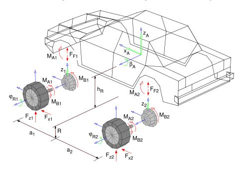
Figure 8.11: Planar Vehicle Model
