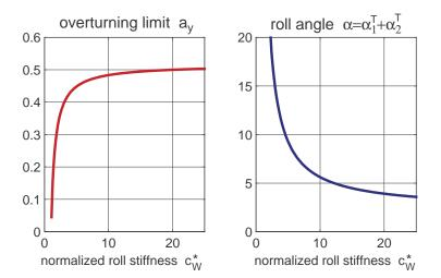
Figure 9.8: Tilting limit for a typical truck at steady state cornering
