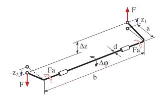
Figure 6.4: Anti-roll bar loaded by vertical forces
