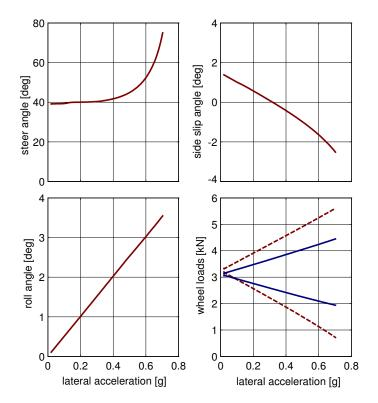
Figure 10.1: Steady state cornering: rear-wheel-driven car on R = 100 m
