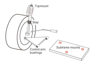
Figure 6.7: Rubber elements in vehicle suspension
