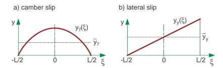
Figure 3.37: Displacement profiles of tread particles
