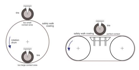
Figure 3.4: Drum and flat bed tire test rig
