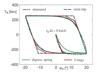
Figure 3.48: Measured [12] and computed parking torque at stand still
