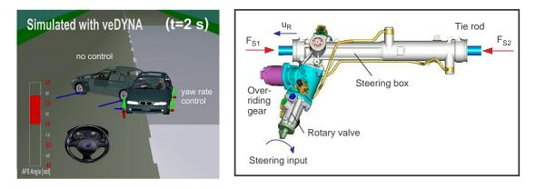
Figure 9.18: Braking on  $\mu$ -split with a standard and an active steering system
