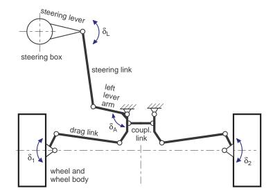
Figure 5.13: Typical bus steering system
