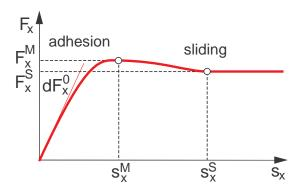
Figure 3.27: Typical longitudinal force characteristics
