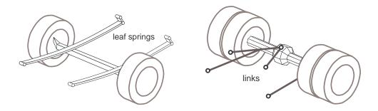
Figure 5.2: Solid axles guided by leaf springs and links
