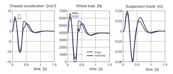
Figure 7.13: Quarter car model driving with  $v = 20 \ km \ h$  over a single obstacle
