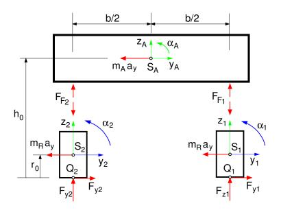
Figure 9.9: Simple vehicle roll model
