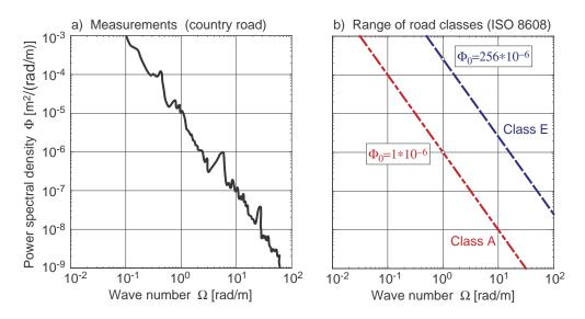
Figure 2.6: Road power spectral densities: a) Measurements [2], b) Classification
