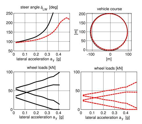
Figure 10.7: Steady State Cornering: Coach -- empty, -- fully occupied
