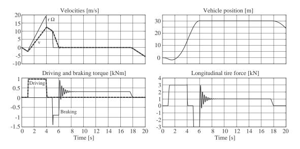
Figure 4.4: Driving and braking on a grade
