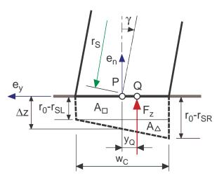
Figure 3.16: Lateral deviation of contact point at full contact
