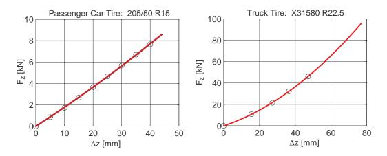
Figure 3.21: Tire radial stiffness: o Measurements, - Approximation
