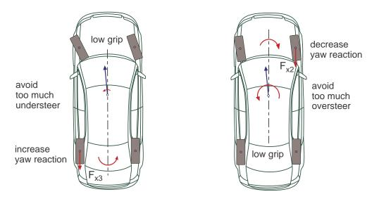
Figure 9.17: ESP braking concepts
