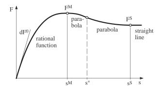
Figure 3.40: Approximation of generalized tire characteristics
