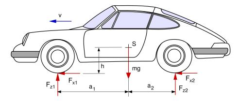
Figure 8.1: Simple vehicle model
