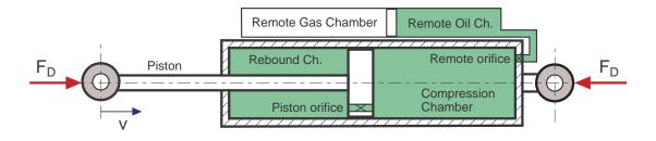
Figure 6.5: Principle of a mono-tube damper
