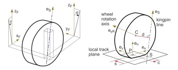
Figure 5.9: Kingpin inclination and caster and steering offset
