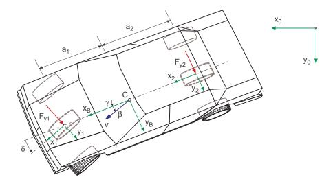
Figure 9.13: Simple handling model
