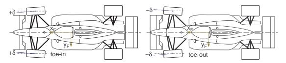
Figure 5.4: Toe-in and Toe-out
