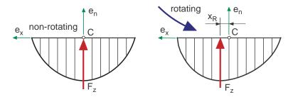
Figure 3.23: Pressure distribution at a non-rotation and rotation tire
