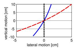
Figure 10.9: Rear axle: — semi-trailing arm, - - single wishbone, … trailing arm
