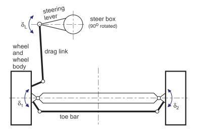
Figure 5.12: Toe bar steering system
