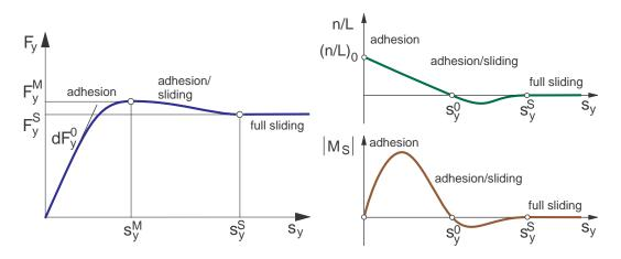
Figure 3.29: Typical plot of lateral force, tire offset and self aligning torque
