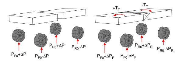
Figure 9.12: Wheel loads for a flexible and a rigid chassis
