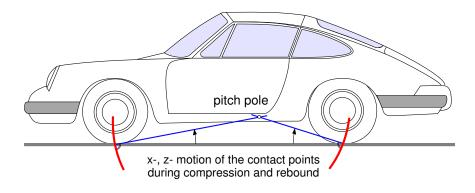
Figure 8.12: Brake Pitch Pole
