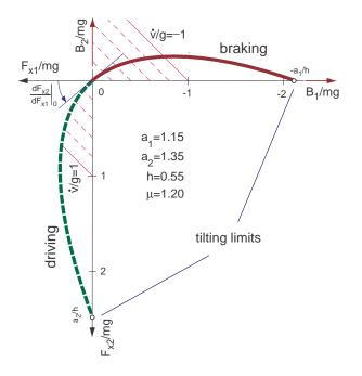
Figure 8.8: Optimal distribution of driving and braking forces
