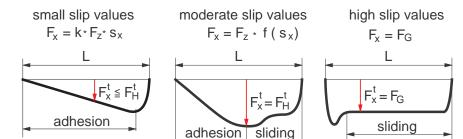
Figure 3.26: Longitudinal force distribution for different slip values
