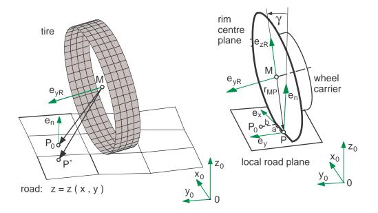
Figure 3.12: Contact geometry
