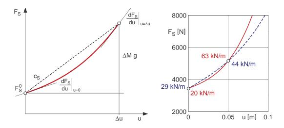
Figure 7.5: Principle and realizations of nonlinear spring characteristics
