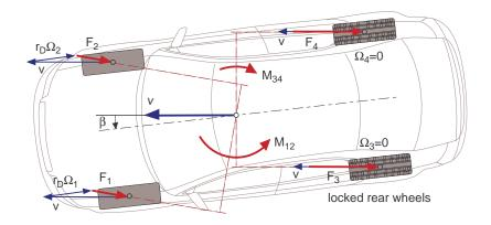
Figure 8.7: Locked rear wheels
