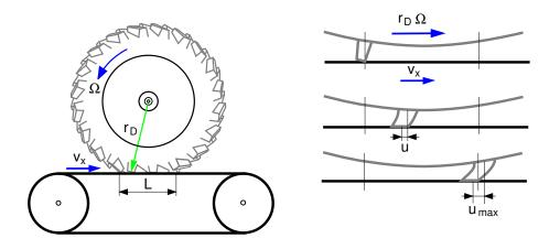
Figure 3.24: Tire on flat bed test rig
