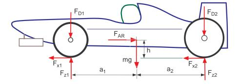
Figure 8.3: Vehicle with aerodynamic forces
