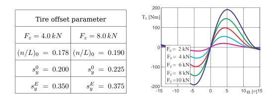
Figure 3.34: Self aligning torque  $T_z$  at different wheel loads
