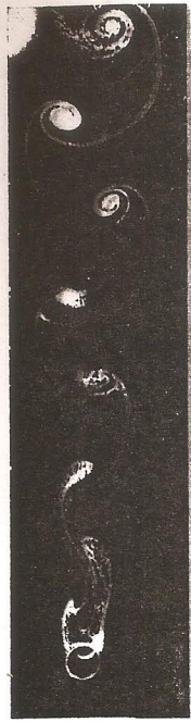
Figure 4.12.6. Streak lines in the wake behind a circular cylinder in a stream of oil. (From Homann 1936a.)
