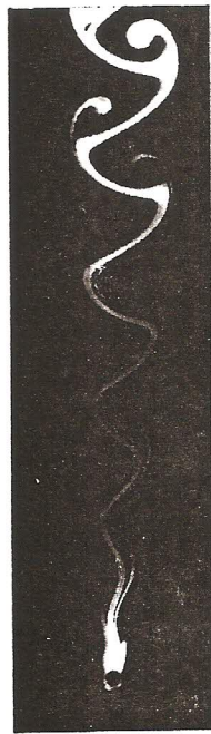
Figure 4.12.6. Streak lines in the wake behind a circular cylinder in a stream of oil. (From Homann 1936a.)
