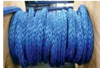
CROSS WINDING Level Layer
