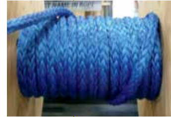
CROSS WINDING First Cross
