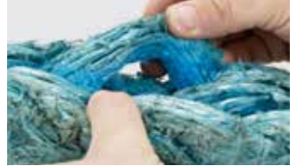
Inspect for pulled strands
