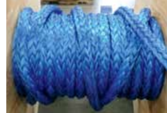
CROSS WINDING Second Cross
