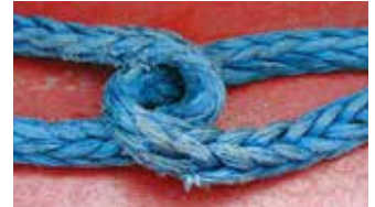
Eye-to-eye splice connection.
