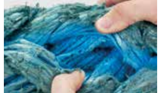
Inspect for internal abrasion
