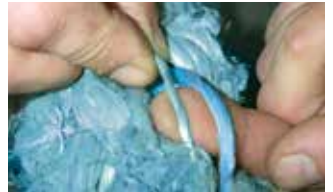
Compare surface yarns with internal yarns
