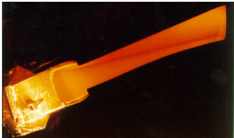
Figure 5 Preheating process observation through one of the wide-angle viewports
