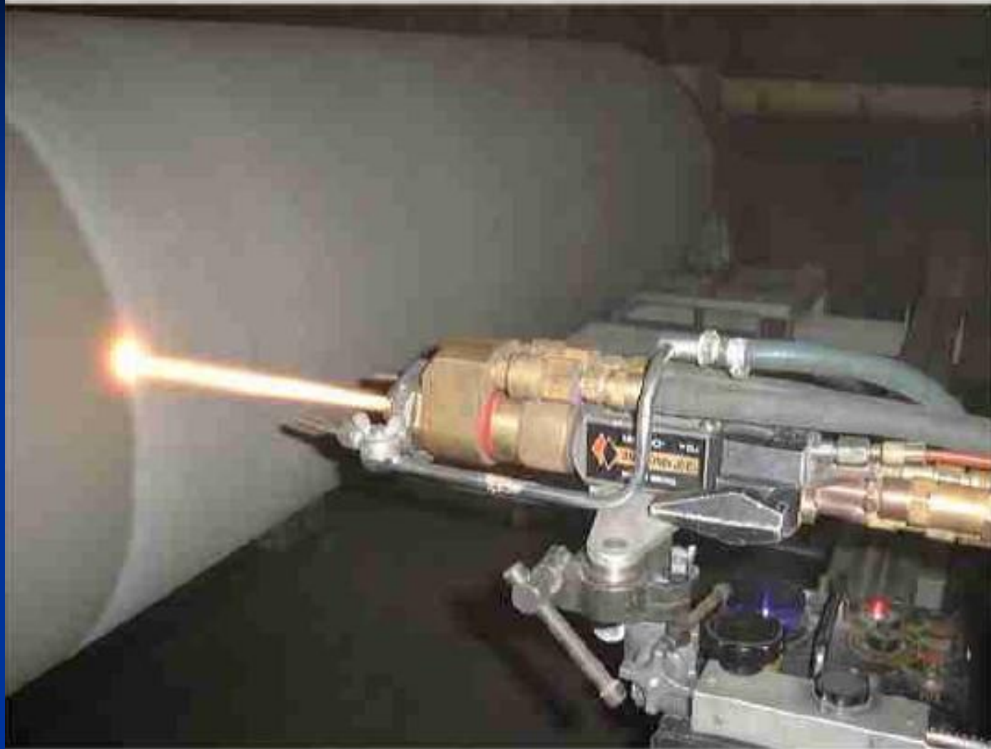
HVOF spraying Tungsten Carbide / Cobalt Chromium Coating (WC/10Co4Cr) onto Roll for the Paper Manufacturing Industry
