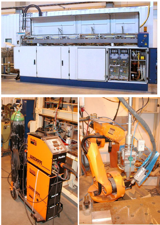
Figure 1. Welding equipment used in the experiments. On the top: 3 kW Nd:YAG-laser, On the left: Kemppi Pro MIG-welding machine, On the right: Hybrid welding head mounted in KUKA KR 15 robot.
