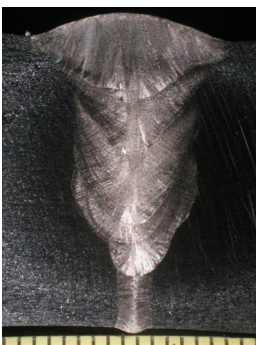
Figure 9. Weld H3 from the test series A.
