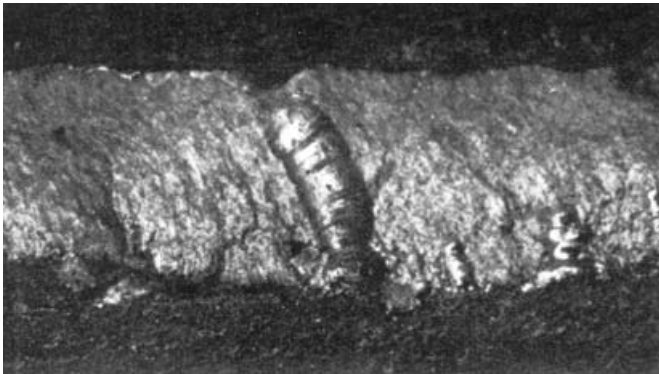
Figure 3.25 Wormhole porosity in weld metal. From Jackson (55).
