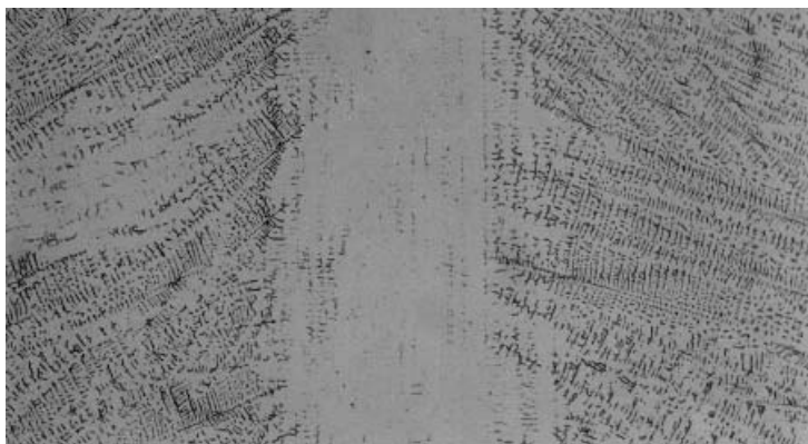
Figure 9.19 Weld centerline austenite in an autogenous gas–tungsten arc weld of 309 stainless steel solidified as primary ferrite. From Kou and Le (9).
