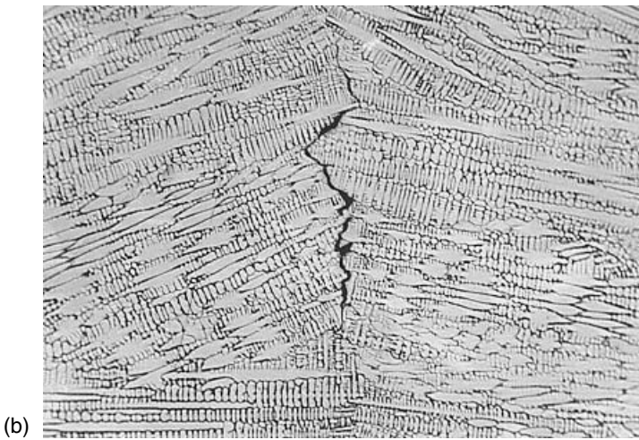
Figure 11.23 Effect of grain structure on solidification cracking: (a) aluminum alloys; (b) centerline cracking in a coarse-grain 310 stainless steel weld. (a) From Nakata and Matsuda (16). (b) From Kou and Le (65).
