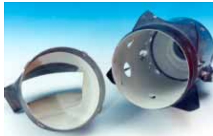
Combustion chamber with APS thermal barrier coating, bond coat NiCrAlY, topcoat ZrO_2 + Y_2O_3
