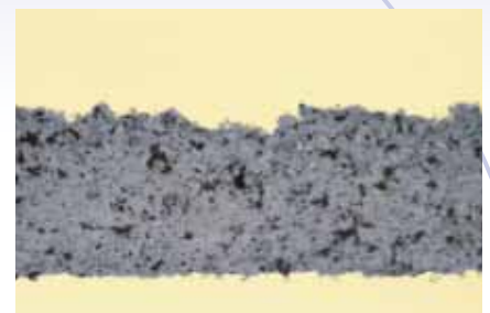
Fig. 2: Same coating as Fig. 1, polished correctly
