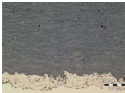
Fig. 6: APS coating with NiCr bond coat and titanium oxide top coating
