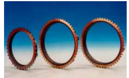
Brass synchronising rings flame-sprayed with molybdenum for wear resistance
