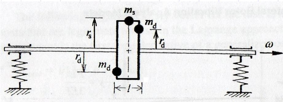
$$[M]\{\ddot{q}\} + [C + G(\Omega)]\{\dot{q}\} + [K]\{q\} = \begin{Bmatrix} 0 \\ 0 \\ m_s r_s \cos \omega t \\ m_s r_s \sin \omega t \\ m_d r_d l \cos(\omega t + \phi) \\ m_d r_d l \sin(\omega t + \phi) \\ 0 \\ 0 \end{Bmatrix}$$
