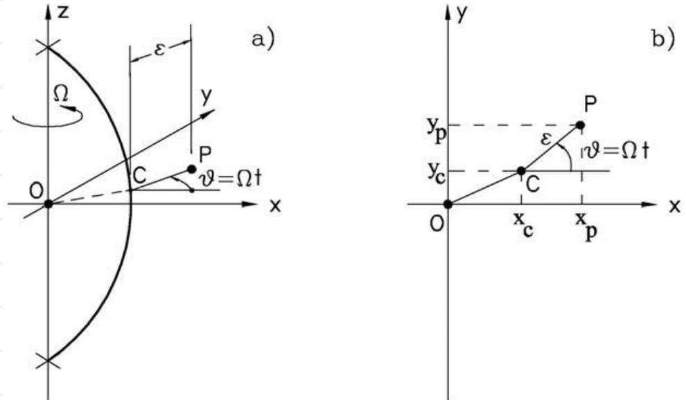
$$\overline{P-O} = r_P(t) = \begin{Bmatrix} x_P(t) \\ y_P(t) \end{Bmatrix} = \begin{Bmatrix} x_C(t) + \varepsilon \cos(\Omega t) \\ y_C(t) + \varepsilon \sin(\Omega t) \end{Bmatrix}$$
