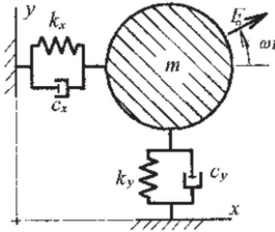
$$\begin{cases} m\ddot{x} + c_x\dot{x} + k_x x = F_0 \cos(\omega t) \\ m\ddot{y} + c_y\dot{y} + k_y y = F_0 \sin(\omega t) \end{cases}$$
