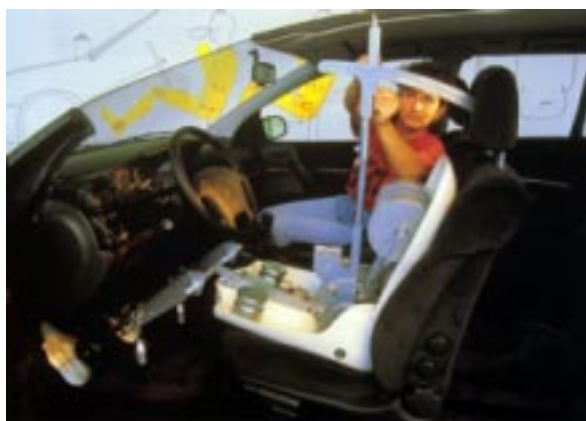
Figure 2: A mechanical test manikin (source Opel)
