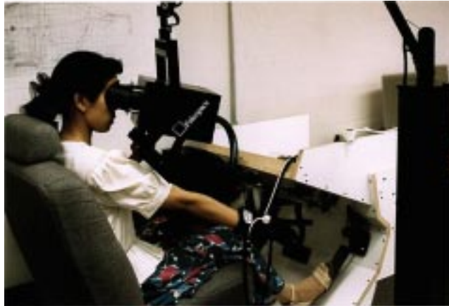
Figure 3: Sit box: User with Boom and data-gloves (source Fakespace)
