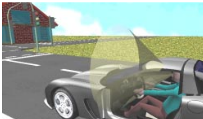
Figure 7. Ramsis' viewing cone seen by an external observer
