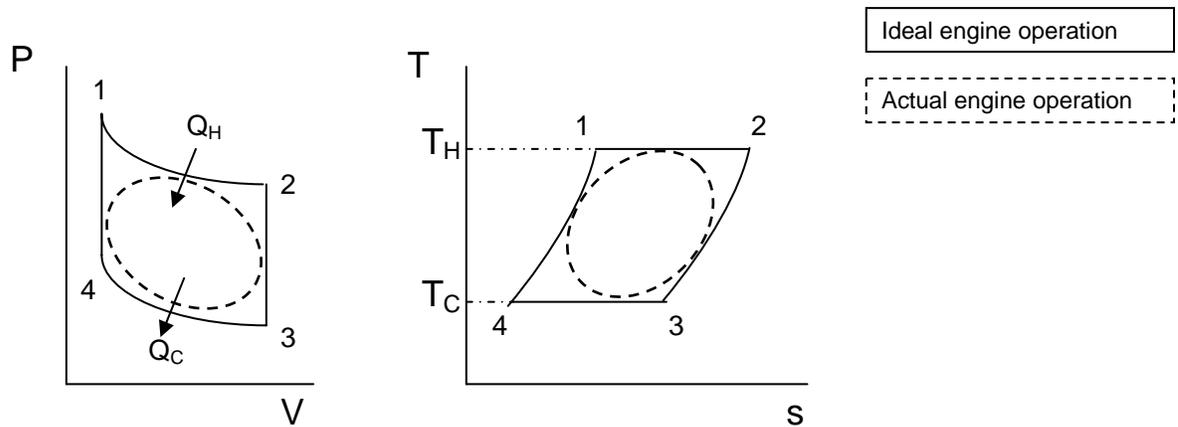
**Figure 1.4.1:** Stirling cycle Pressure-Volume and Temperature-Entropy diagrams
