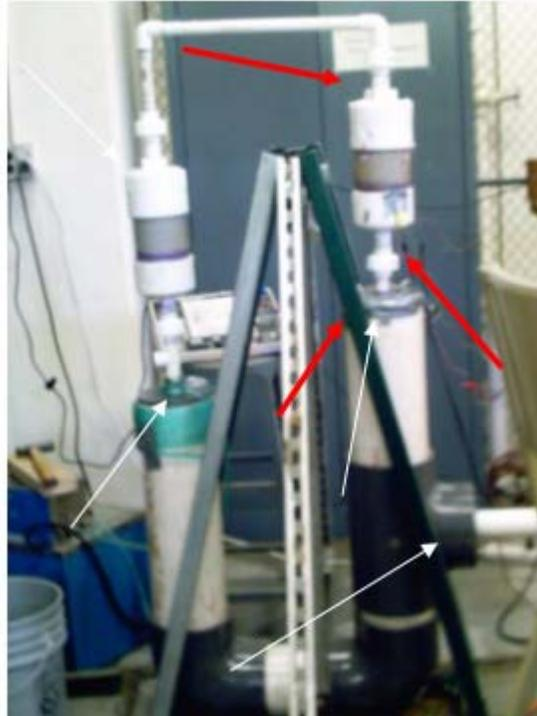
*Figure 5.1 Picture of system; the red arrows show where leakage occurred; the white arrow show where frictional losses were observed.*
