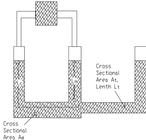
**Fig 2.4.1: Tuning column configuration with merged cylinders**
