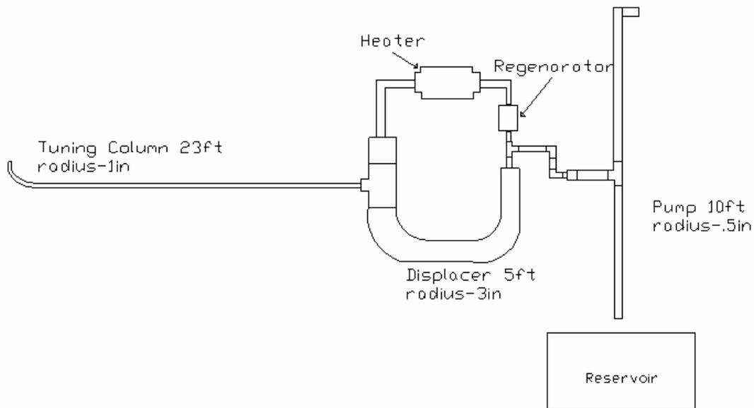
Fig 3.1.1: Design diagram of our fluidyne pump
