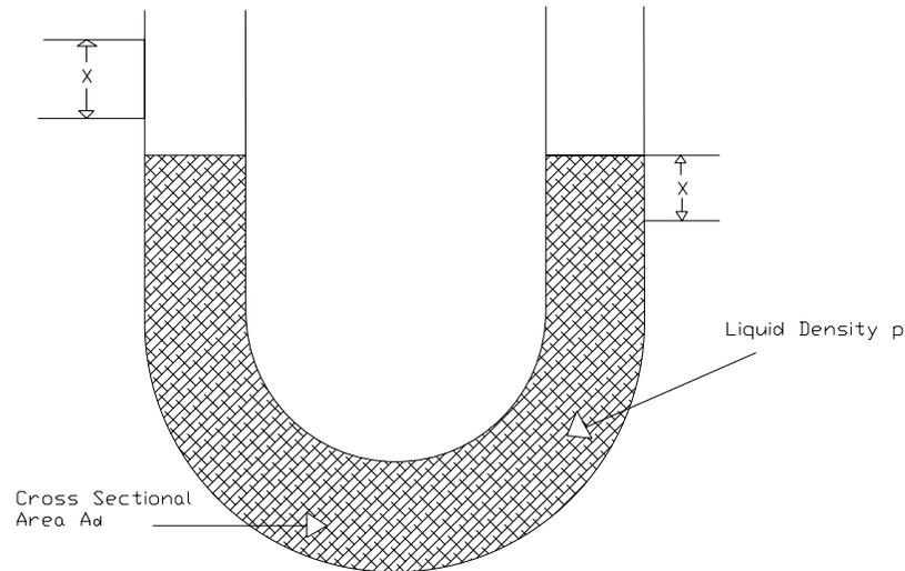
**Fig.2.3.1 Simple Displacer U-Tube**
