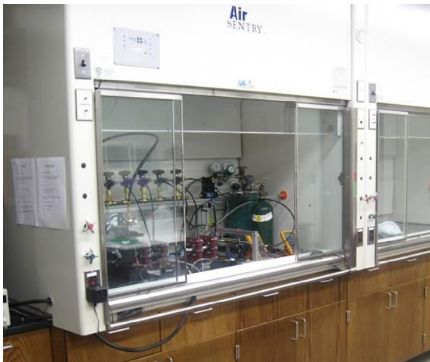
Figure 4.13: Fuel cell test station.
