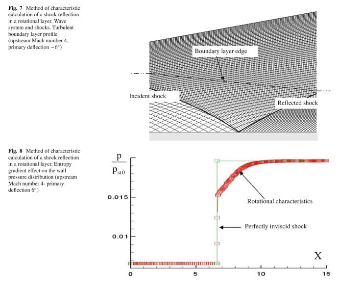
description of the complex wave pattern which is generated when a shock traverses a boundary layer considered as a rotational inviscid stream. However, the above scenario does not take into account the upstream transmission through the subsonic part of the boundary layer with the subsequent generation of compression waves, which coalesce to produce the reflected shock.
