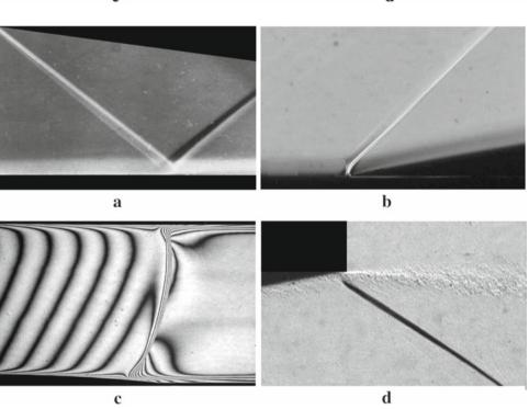
a supersonic air-intake of the mixed compression type or at the impact of the shock generated by any obstacle on a nearby surface.
