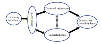
Fig. 18 A diagrammatic representation of shock boundary layer interactions
