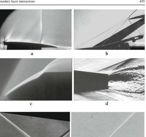
Fig. 2 Basic shock wave/boundary layer interactions (Onera documents). a oblique shock reflection, **b** ramp induced shock wave, c normal shock wave, **d** adaptation shock at a nozzle exit
