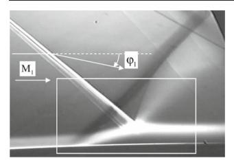
Fig. 10 Schlieren visualisation of an incident-reflecting shock at Mach 2 (Onera document)
