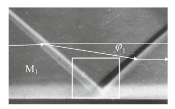
Fig. 4 Schlieren photograph of a shock reflection at Mach 1.95 (Onera document)
