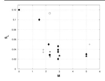
Fig. 19 Dominant frequency in supersonic shock/boundary layer interactions (from [26])
