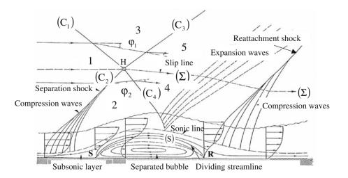
the purely inviscid case and the shock reflection is said to be a *strong viscous-inviscid interaction*. This means that the viscous effects have to be taken fully into account when predicting the flow. They are no longer a simple adjustment to an already nearly-correct inviscid solution, but they play a central role in the establishment of the solution. It is evident that there has been a hierarchy reversal.
