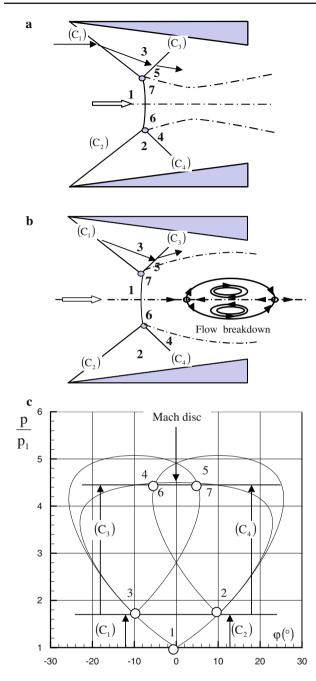
**Fig. 17** Direct and inverse Mach phenomenon. **a** direct Mach phenomenon, **b** inverse Mach phenomenon, **c** inverse Mach phenomenon: Situation in the shock polar plane  $(M_1 = 2, \varphi_1 = 10^\circ, \varphi_2 = -10^\circ)$
