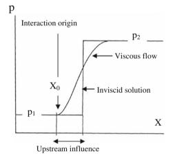
Fig. 6 The corresponding pressure distribution
