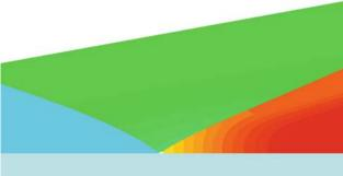
**Fig. 9** Method of characteristic calculation of a shock reflection in a rotational layer. Static pressure contour. Turbulent boundary layer profile (Upstream Mach number 4, primary deflection  $-6^\circ$ )
