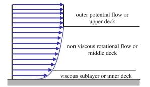
Fig. 3 The interacting flow multi-layer structure or triple deck (Lighthill, Stewartson–Williams)
