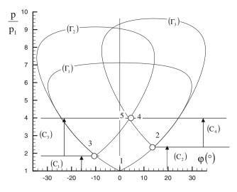
Fig. 13 Shock pattern interpretation in the shock polar diagram. Upstream Mach number 2. Separation shock deflection  $14^{\circ}$ ; incident shock deflection  $-10^{\circ}$
