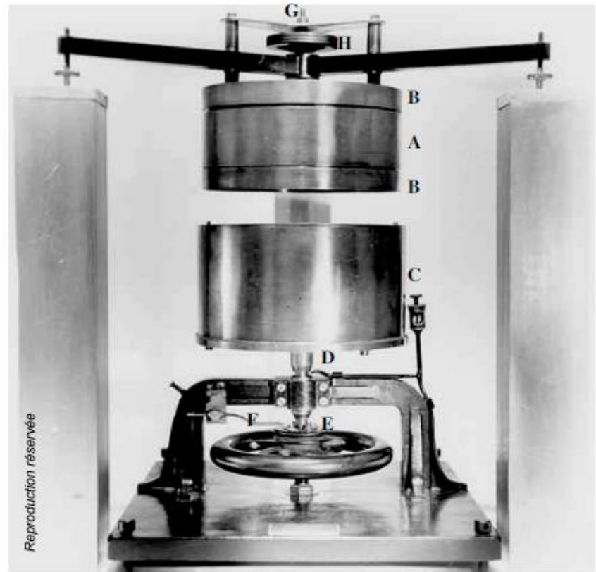
Figure 2. Maurice Couette's concentric cylinder apparatus (viscometer) (1888)
