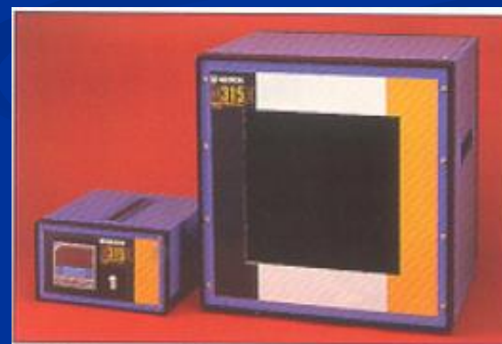
FIGURE 4. For calibrating thermal imaging systems or mapping and surveillance equipment, or for long-path spectrophotometers, a calibration source requires a large target area. Source (on the right) area is 305 mm square; the controller is on the left.
