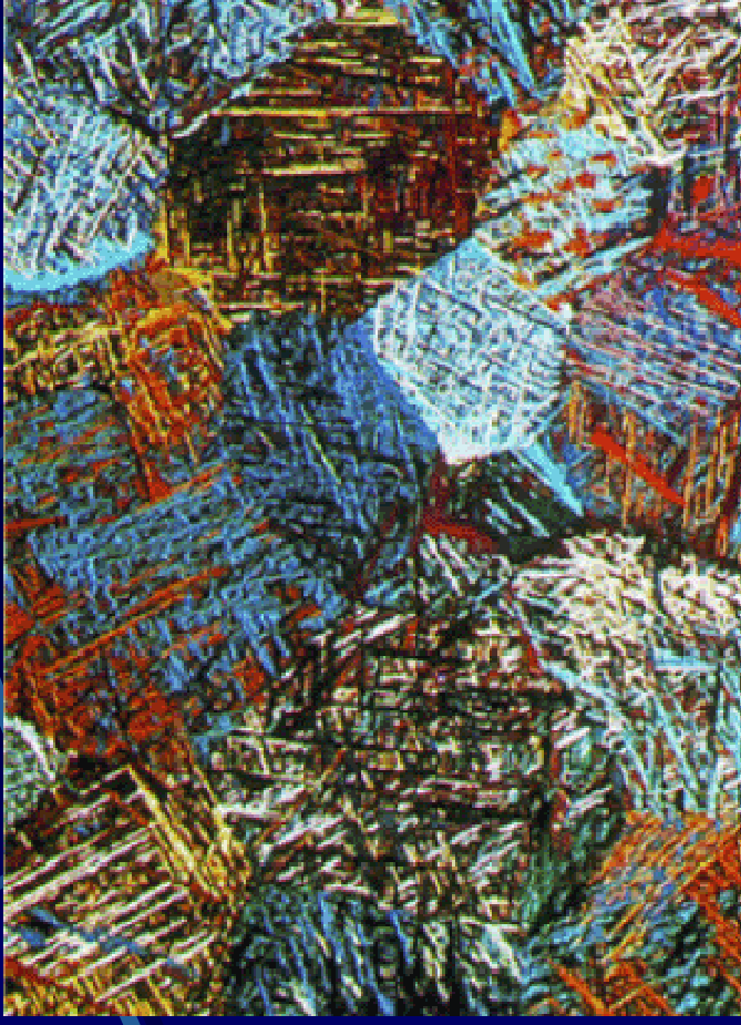
Fig. 4. TI-831-400 alloy containing mannose; needles formed at elevated temperatures, 365 to 400 or 450 °C. Isolates in 450 mL PBS, 3 mL H 2 O, 3 mL HEPES. Polarized light illumination. Original magnification 100x. Courtesy of Dr. Daniel Goulet; Ref. 1
