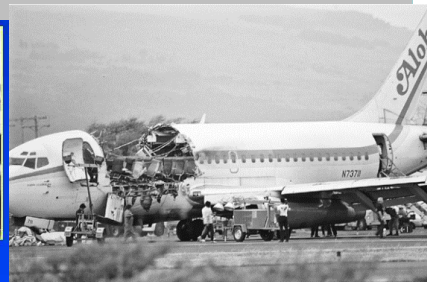
Failed fuselage of the Aloha 737 aircraft in 1988.
