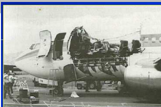
Failed fuselage of the Aloha 737 aircraft in 1988.
