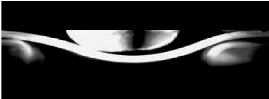
33-percent bead penetration, t = 1.2 mm Sheetmetal movement →
