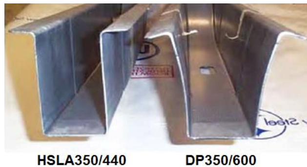
Figure 1. Effects of springback in U-drawbending parts. Adapted from IISI, 2006.
