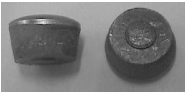
Figure 1. An 8,0 mm sheet slug evidencing the material " blow-out".
