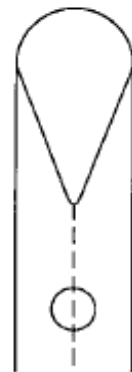
Figure 9.19 Weld centerline austenite in an autogenous gas–tungsten arc weld of 309 stainless steel solidified as primary ferrite. From Kou and Le (9).
