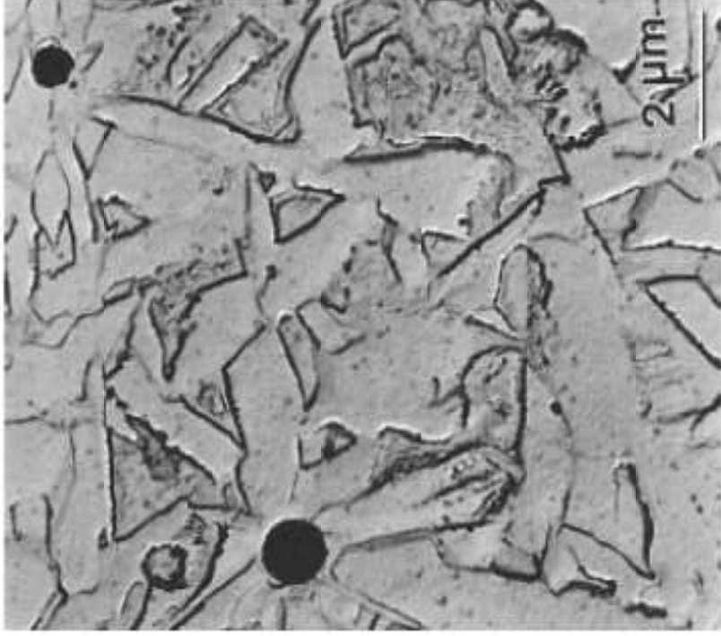
Figure 9.24 Acicular ferrite and inclusion particles in a low-carbon, low-alloy steel weld. Reprinted from Babu et al. (47).
