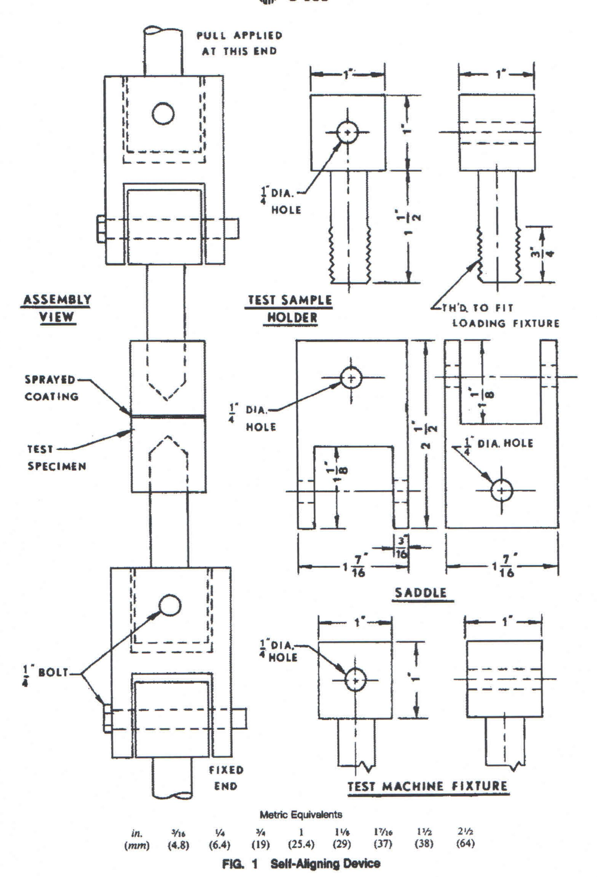
it shall first be compared with a proven bonding agent using this method with the desired flame-sprayed coating.
