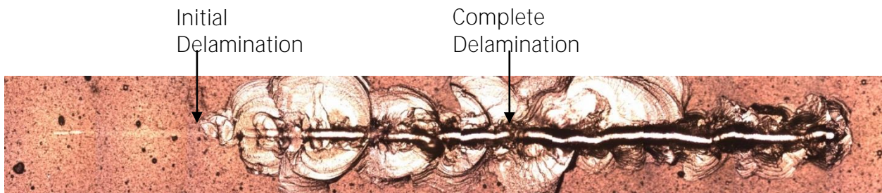
Fig. 8: Micrograph of full scratch of Brittle Ceramic Coating.
