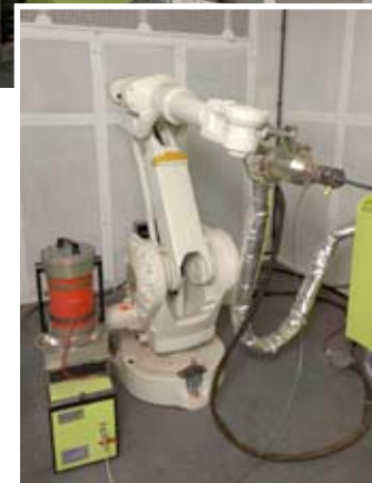
TWI's state-of-the-art cold spray system
