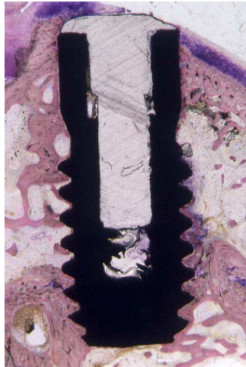
Fig. 9. Test implants. A mature compact bone is present around the implant perimeter. Toluidine blue and acid fuchsin 20 × .
