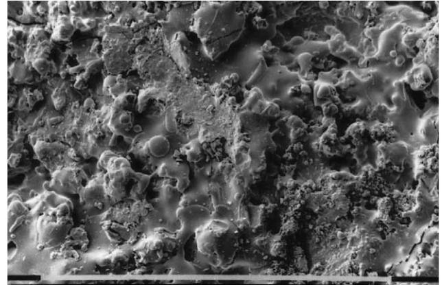
Fig. 1. Scanning electron microscopy of a hydroxyapatite-coated titanium dental implant. The HA surface looks irregular and shows a microporosity which increases the implant surface and plays an important role in favouring early peri-implant osteogenesis. Bar = 100  $\mu\text{m}$ .
