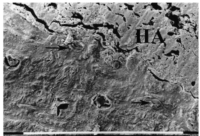
Fig. 2. HA-coated titanium dental implant from human. The newly formed mature lamellar bone is in close contact with the HA-coating surface (HA): no gap or soft tissue are present at the interface. Young osteocytes recognizable in wide lacunae are aligned parallel and next to the implant surface (arrows). Bar = 100  $\mu\text{m}$ .
