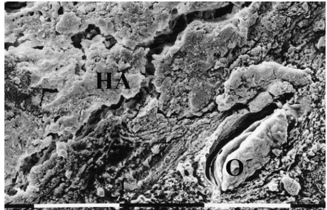
Fig. 4. Scanning electron microscopy of an HA-coated titanium dental implant from human. On the bottom right side, around an osteocyte (O) next to the implant surface, collagen fibrils of a newly formed bone (see enlargement of this picture in Fig. 5) in close contact with the HA surface (HA) are seen. Bar = 10  $\mu\text{m}$ .
