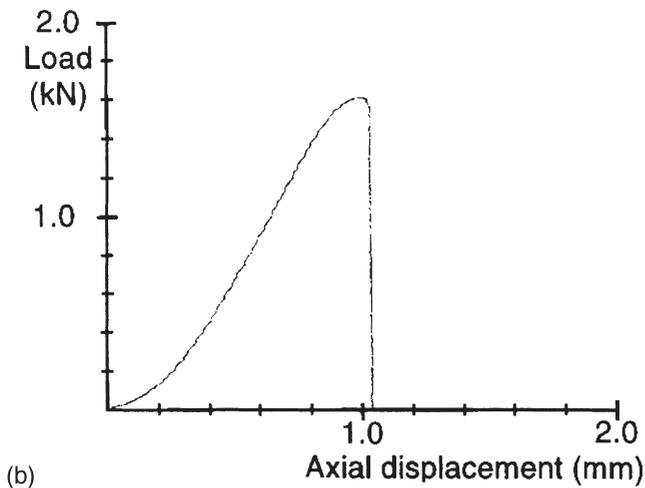
Fig. 3. (a–b) Sample test results obtained with the equipment described herein applied to living (anaesthetized) beagle dogs. (a) Sample torsion test result. Unloading and reloading was done after about 3° of rotation with a remaining irrecoverable angular deformation of about 2°. (b) Sample pull-out test result.
