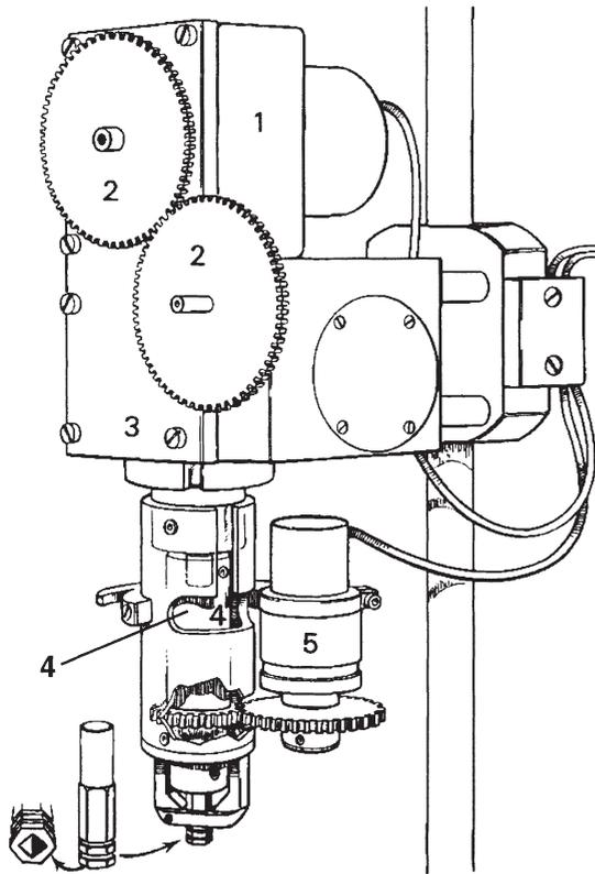
Fig. 2. The motor (1), gear (2), gear train (3) and sensing elements (4,5) used to apply and measure torque and angular displacements.
