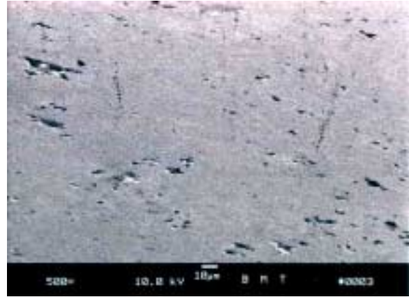
Figure 11 – 0.40 µm (16 µin) Ra Finish HVOF WC-Co-Cr Coating Following Superfinishing to a 0.05 µm (2 µin) Ra Finish (500X).
