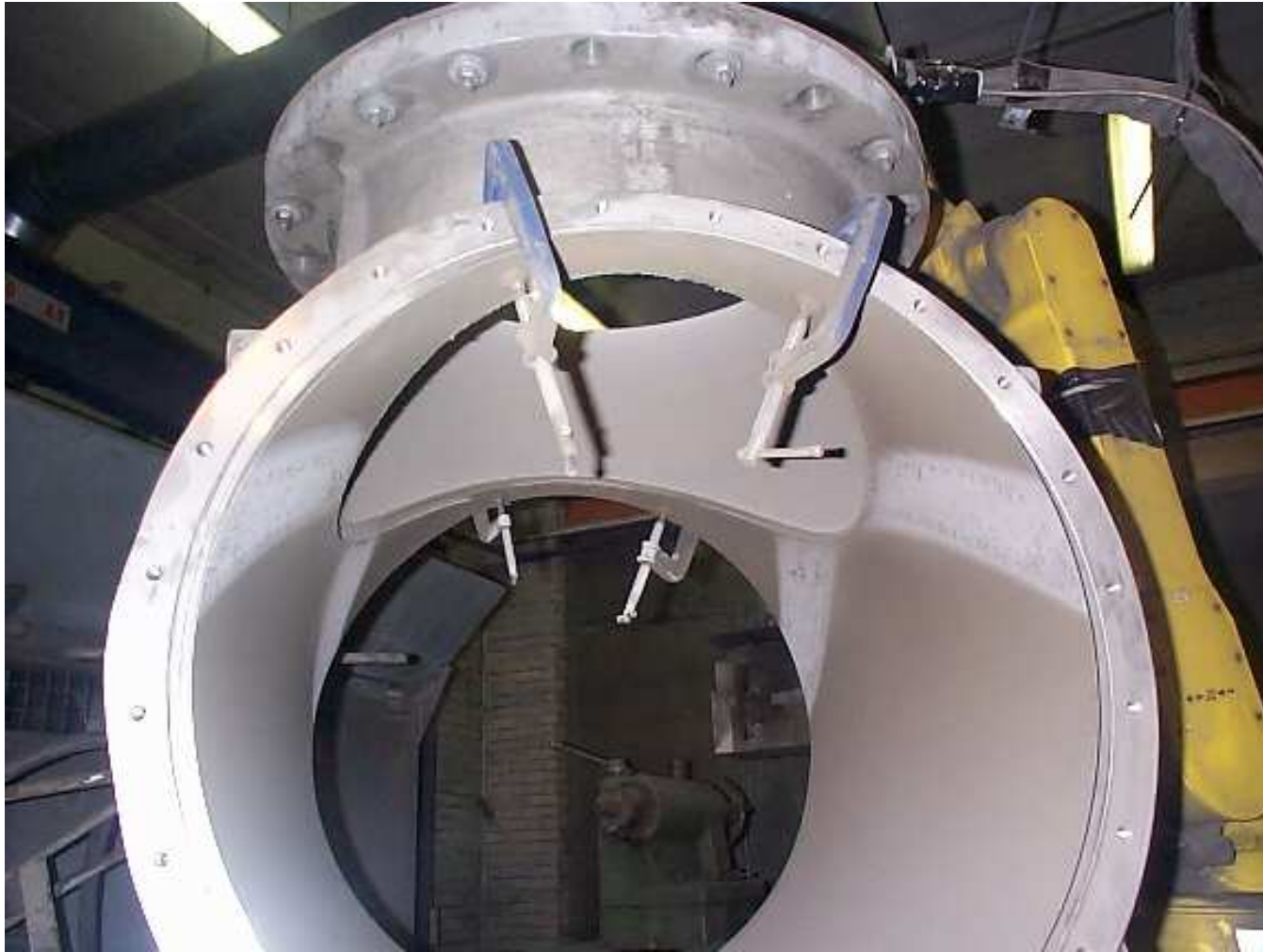
Valve body (JK591 – corrosion resistant)
