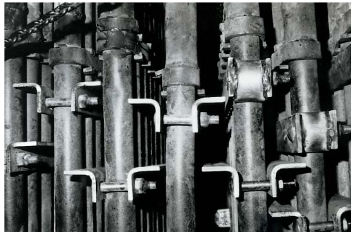
Coal fired power plant using a pressurized fluidized bed combustion (PFBC) boiler. RA 253 MA used for the cyclones (pictured), and gas collecting pipe for this project at American Electric Power (AEP) TIDD project in Brilliant, OH. Cyclones separate out particulate from the exhaust gases, which are fed into a gas turbine. Combustion temperatures were 1500-1600°F. RA 253 MA selected for its excellent strength and its resistance to wastage by the combined effects of oxidation, sulfidation and abrasion.
