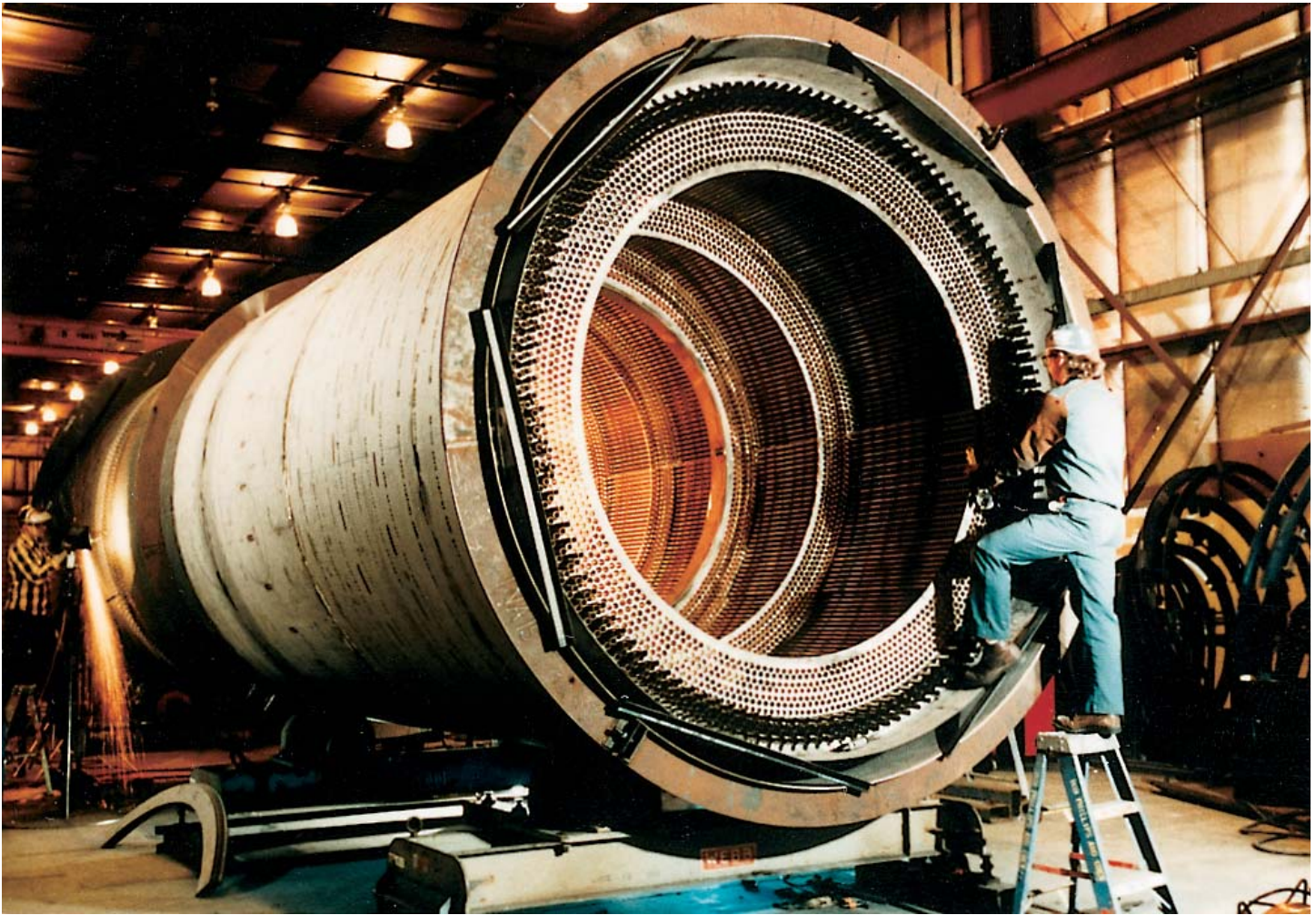
RA 253 MA material used for the hot sections of this recuperative thermal oxidizer for both the tubesheets and the shell. of the unit.
