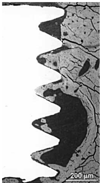
Fig. 3. Representative backscatter SEM of bone formed at machined implant (original magnification, \times 200 ).
