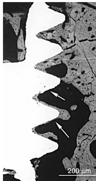
Fig. 5. Representative backscatter SEM of bone formed at implant with ideal pit topography (original magnification, \times 200 ). Note confluence of bone formation against implant surface.
