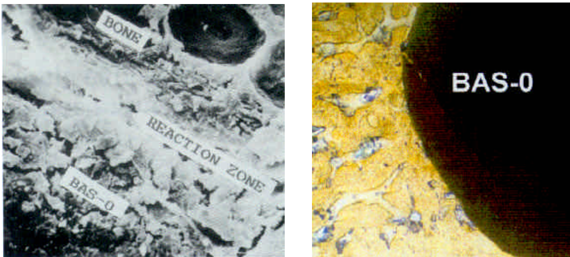
Fig.2: Detail of the interface of the bone tissue with a BAS-O implant 6 months after implantation (SEM). Fig.3: Photomicrograph of a section of BAS-0 granule implant in bone, 2 years after implantation (toluidine blue stain).
