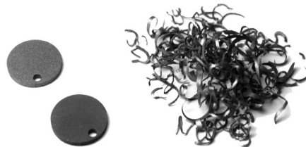
Fig. 1 Samples - titanium discs and turnings used for exposure in SBF
