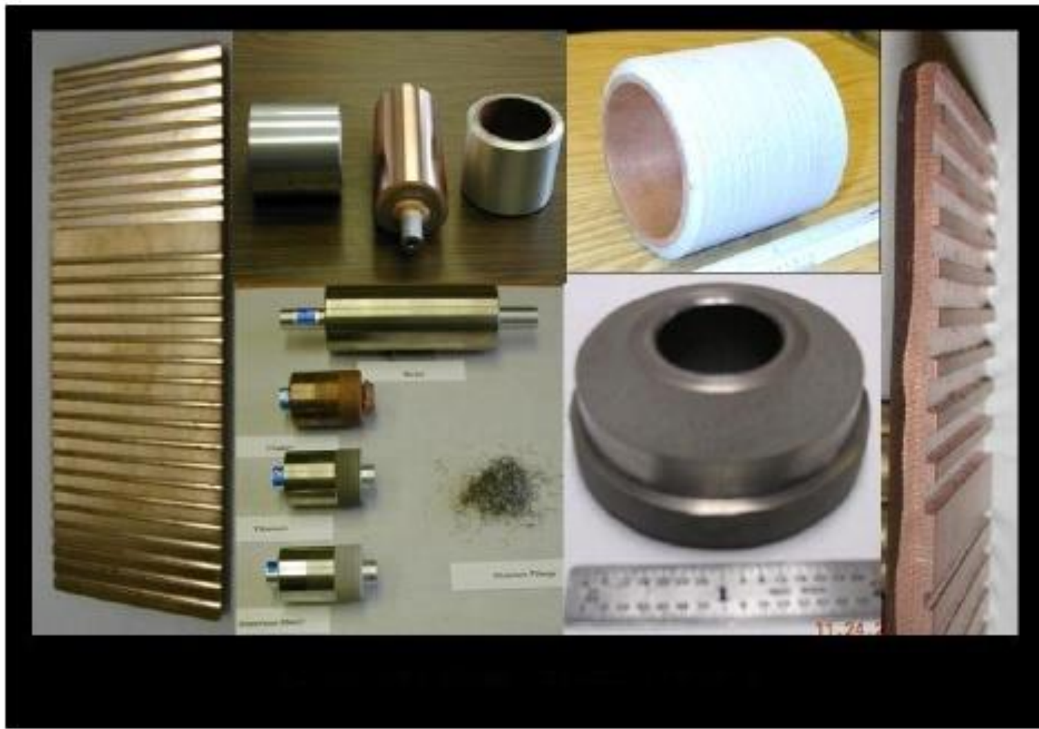
Figure. 6: Cold Spray Produced Bulk Forms
