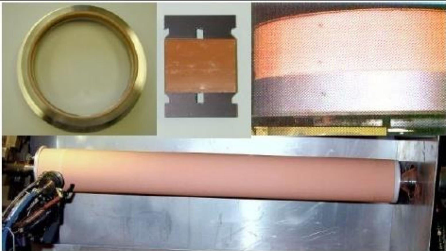
Figure 5: Typical Cold Sprayed Coatings
