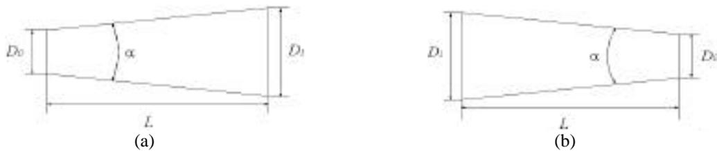
Figure 1. Schematic cross-sectional views of (a) a diffuser and (b) a nozzle
