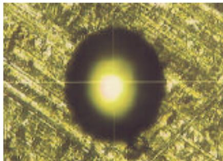
Figure 8. The picture of fabricated nozzle under optical microscope( $\times 200$ )
