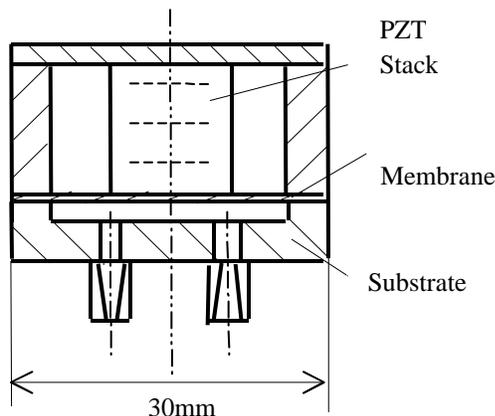
Figure 6. The diagram of the piezoelectric micro pump
